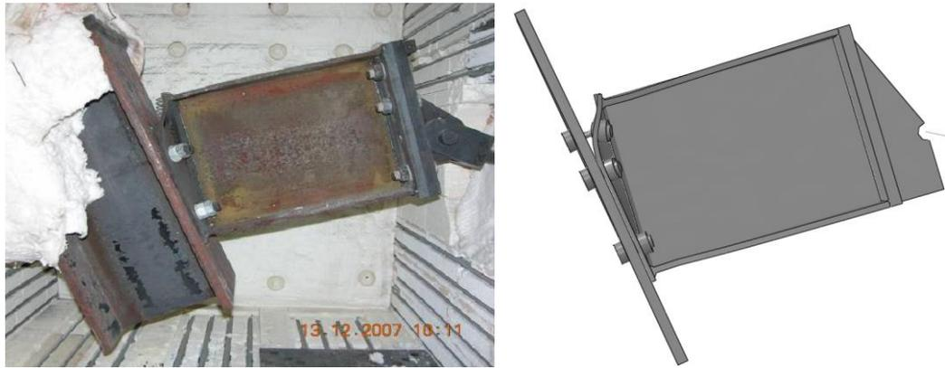
Figure 3-16 Overall deformation comparison
