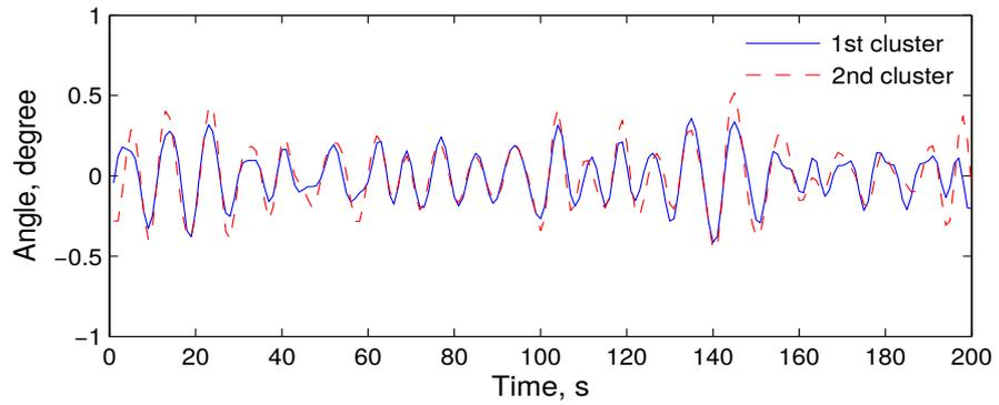
(b) DOA fluctuations in the frequency interval 0.05-0.2 Hz.
