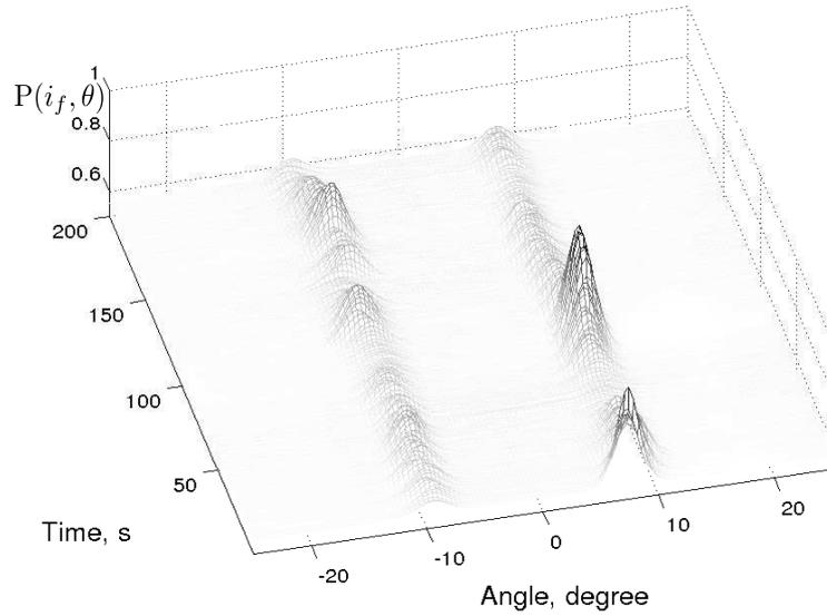
Figure 4.5: Spatial power distribution  $P(i_f; \theta)$  in the sea trial at a distance of 105 km; positive angles correspond to acoustic rays received from the sea surface direction while negative angles show rays from the sea bottom direction.
