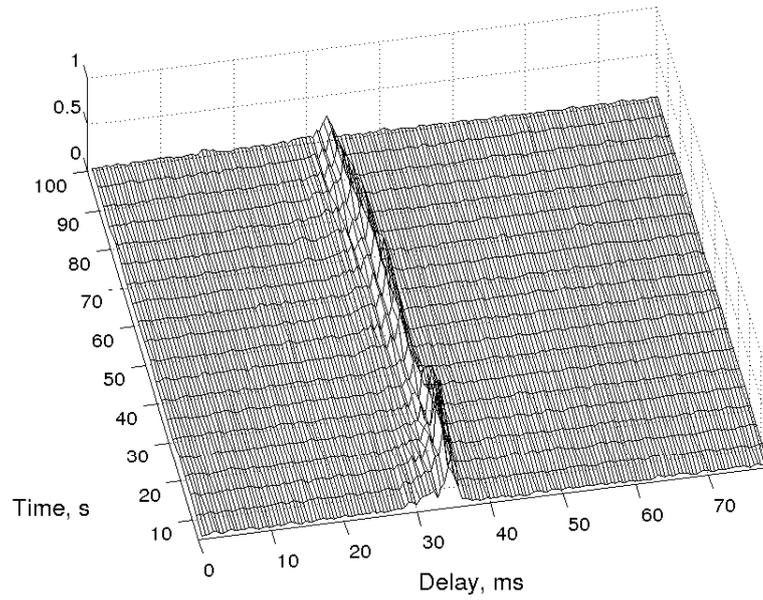
Figure 5.10: Fluctuations of the channel impulse response at the first hydrophone in the F1-1 session.
