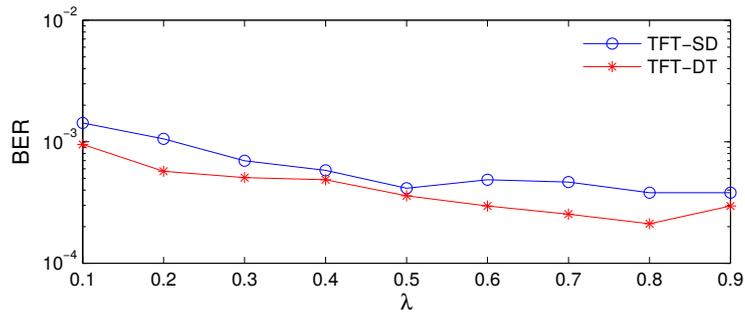
Figure 5.13: Coded BER performance of the receiver with the TFT-SD and the TFT-DT beamforming techniques in the F1-2 session; the code represented by polynomial in octal [5 7 7].
