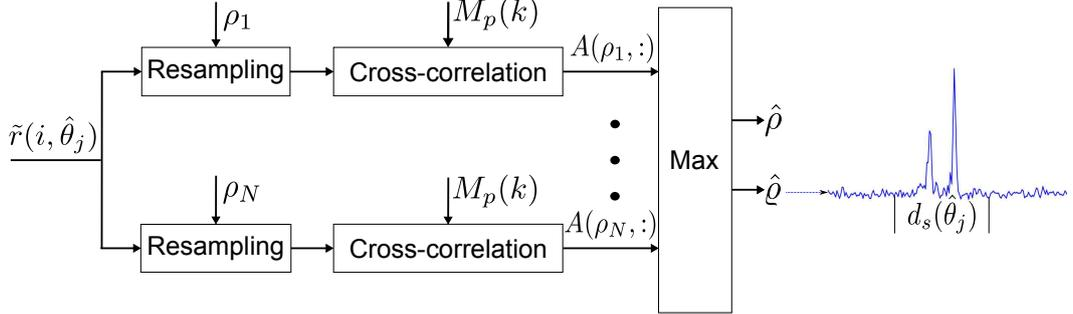
Figure 4.9: Block diagram of the Doppler estimator.
