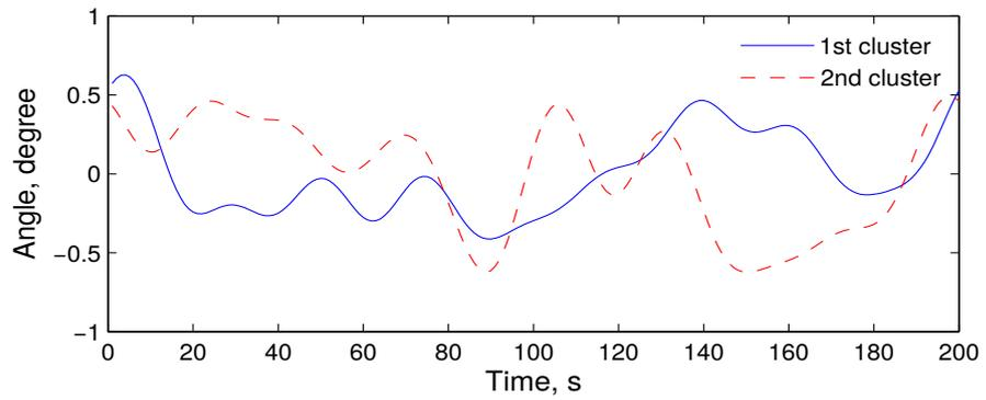
(c) DOA fluctuations in the frequency interval 0-0.05 Hz.
