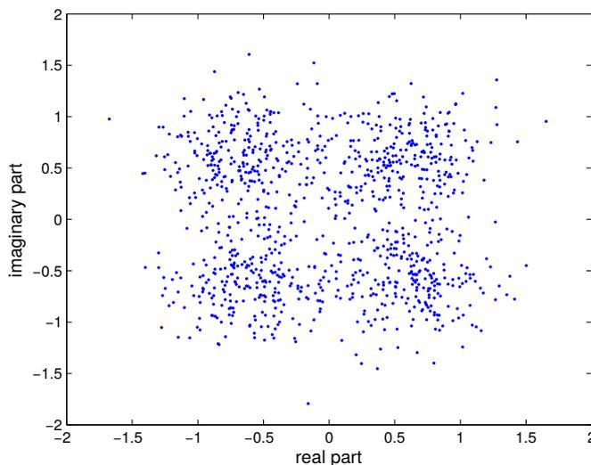
Figure 6.9: Constellation diagram of combined signal  $\tilde{X}_l(k)$  before OFDM demodulator shown in Figure 6.6.
