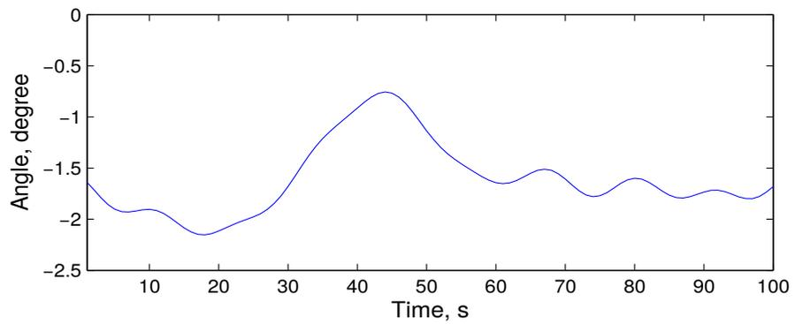
(c) DOA fluctuation in the frequency interval 0-0.05 Hz.
