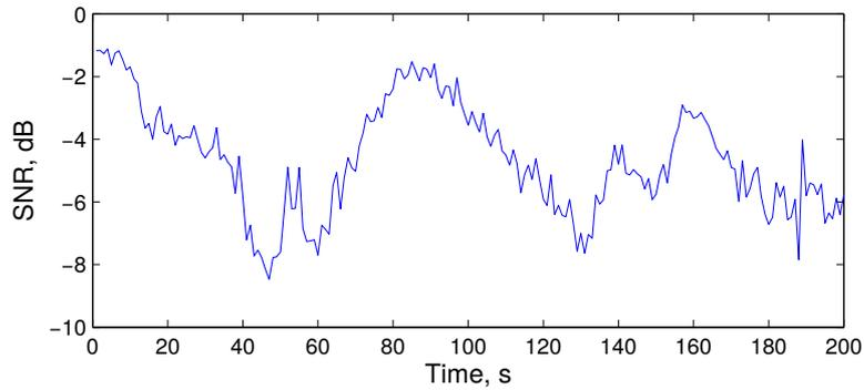
Figure 4.11: SNR at the first hydrophone in the sea trial at a distance of 105 km.
