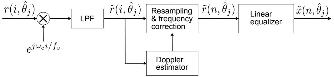
Figure 4.8: Block diagram of the equalizer.
