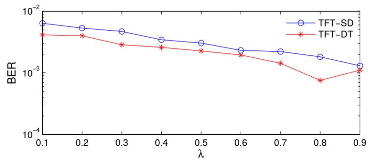
Figure 5.12: Coded BER performance of the receiver with the TFT-SD and the TFT-DT beamforming techniques in the F1-1 session; the code represented by polynomial in octal [561 753].
