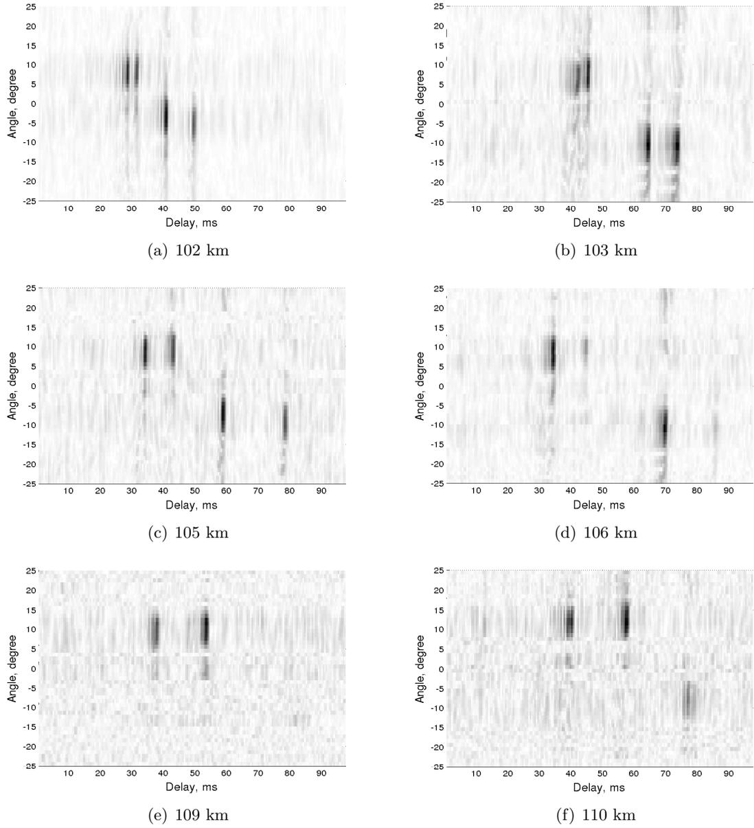
Figure 4.3: Experimental space-time distributions of received signal observed at various distances from 102 km to 110 km.
