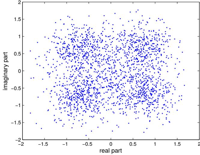
Figure 6.5: Constellation diagram of frequency domain signal before OFDM demodulator shown in Figure 6.1.
