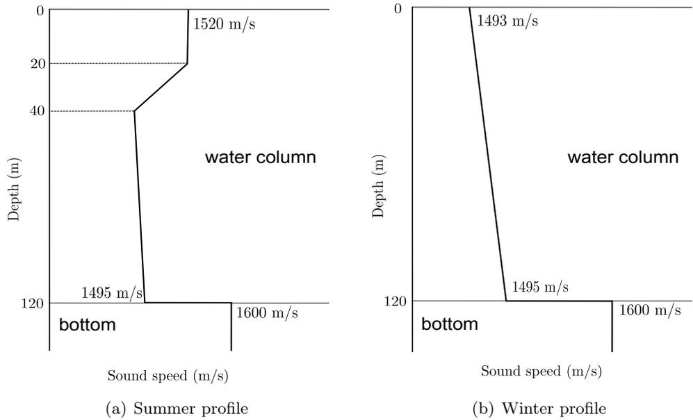
Figure 3.7: The canonical shallow water SSPs [2, 3] used in the simulation; For convenience, Figure 2.3 is shown here again.
