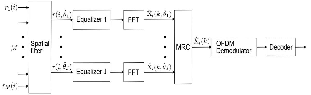
Figure 4.4: Block diagram of the receiver.
