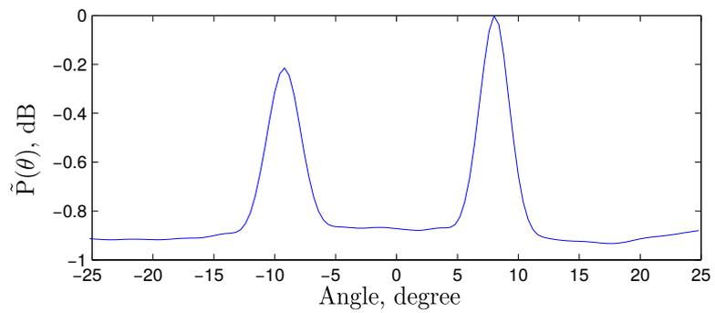
(b) The average spatial signal power  $\tilde{P}(\theta)$  obtained at an angle step of  $0.1^\circ$ .
