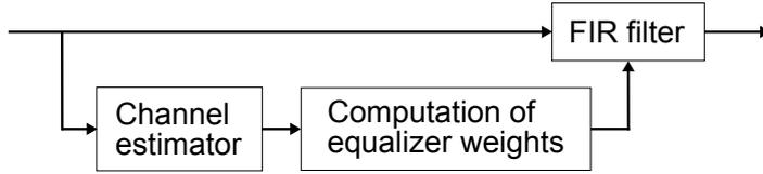
Figure 6.2: Block diagram of a single branch of the equalizer [4] (for convenience, we show Figure 3.5 again).
