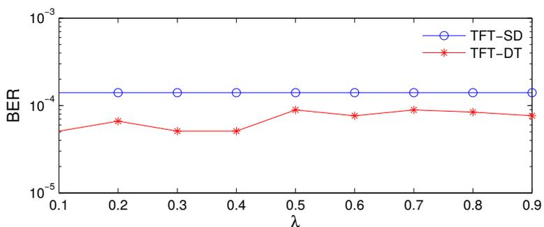
Figure 5.7: Coded BER performance of the receiver with the TFT-SD and the TFT-DT beamforming techniques in this simulation; the convolutional code described by the polynomial in octal [3 7].
