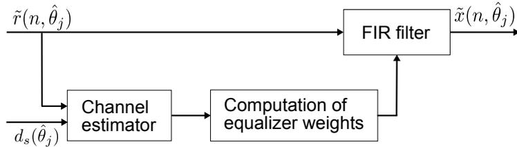
Figure 4.10: Block diagram of the linear equalizer.
