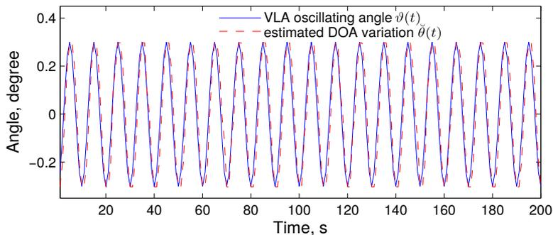
Figure 5.6: Comparison of the VLA oscillating angle  $\vartheta(t)$  and the estimated DOA fluctuation  $\check{\theta}(t)$  in this simulation.
