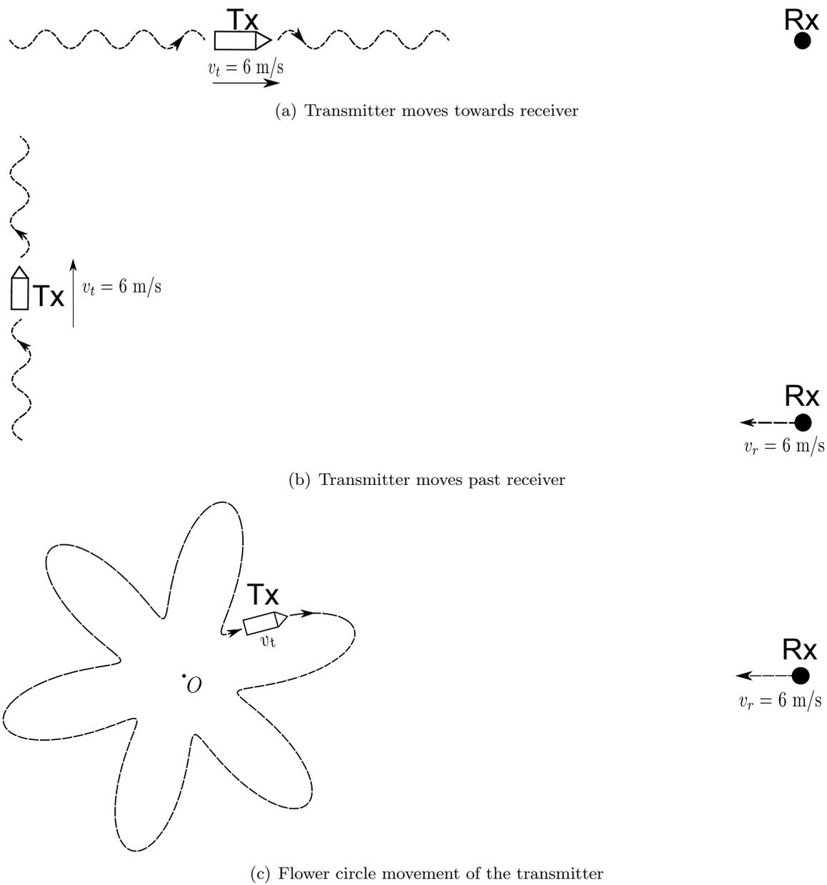
Figure 3.6: Simulation scenarios (top view; Tx is the transmitter, and Rx is the receiver).
