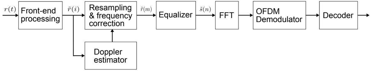
Figure 6.1: Block diagram of the receiver of guard-free OFDM signal.
