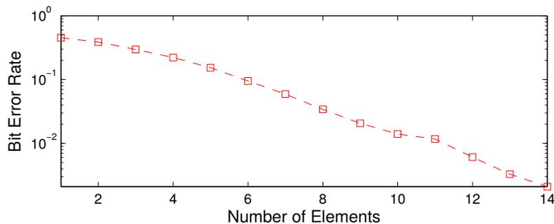
Figure 6.7: Coded BER performance with different number of elements; the convolutional code described by the polynomial in octal [225 331 367].
