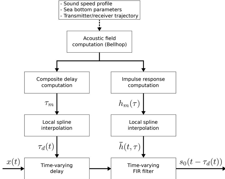
Figure 3.2: A block diagram of the *Waymark* underwater acoustic simulator; adapted to this chapter.
