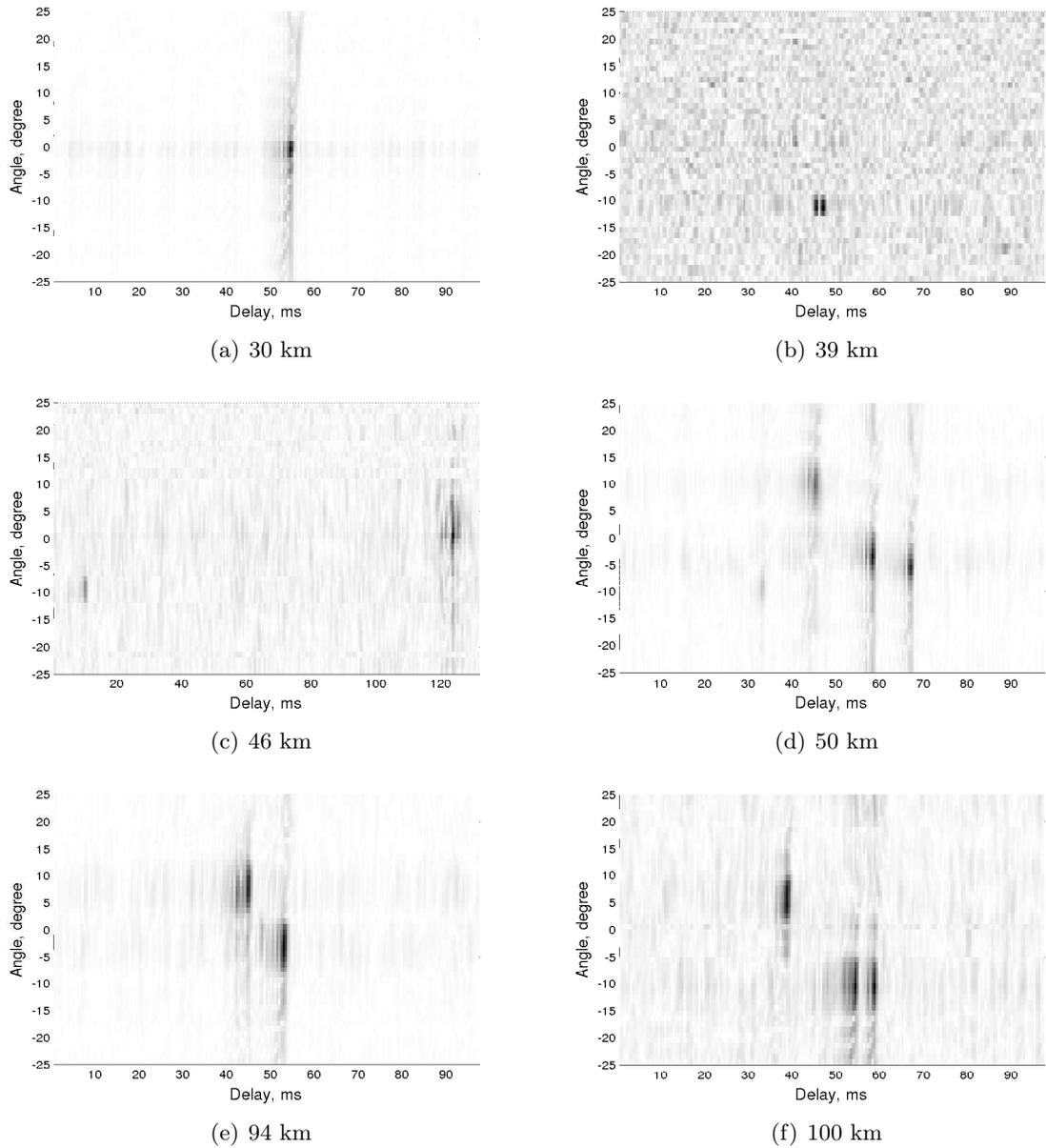
Figure 4.2: Experimental space-time distributions of received signal observed at various distances from 30 km to 100 km.
