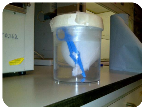
(a) Bladder being decellularised using the original process. Total volume of solution per bladder is 1 L.
