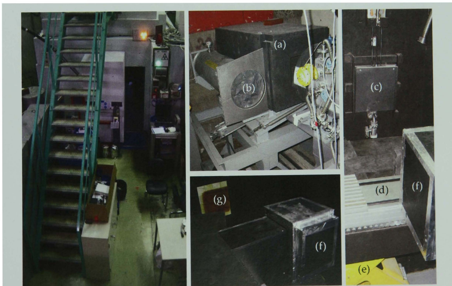
Figure 3.11: Photographs of Neutrograph (left), the primary casemate (top centre), and the experimental casemate (bottom centre and right) showing (a) the primary beam shutter, (b) the flight tube, (c) the secondary beam shutter, (d) the linear motion table, (e) the lifting table, (f) the camera box, and (g) the neutron beam stop.
