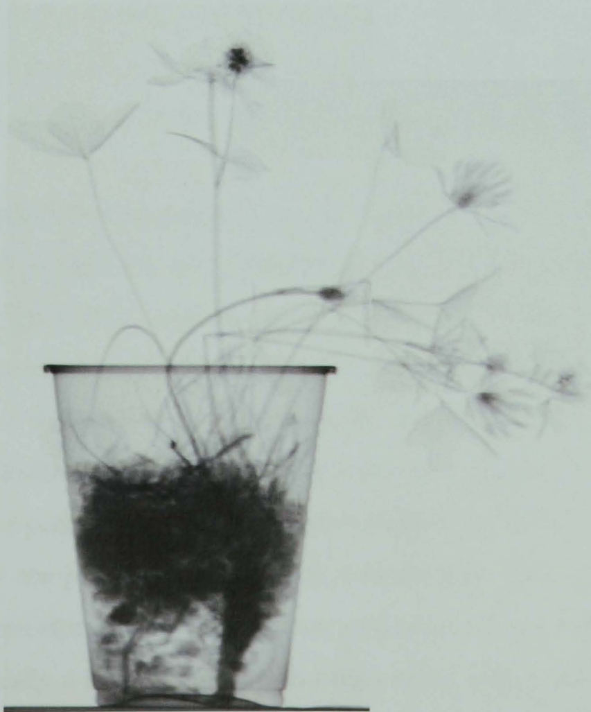
Figure 2.2: A neutron radiograph of a wild flower. The image is a negative; darker areas indicate higher attenuation.
