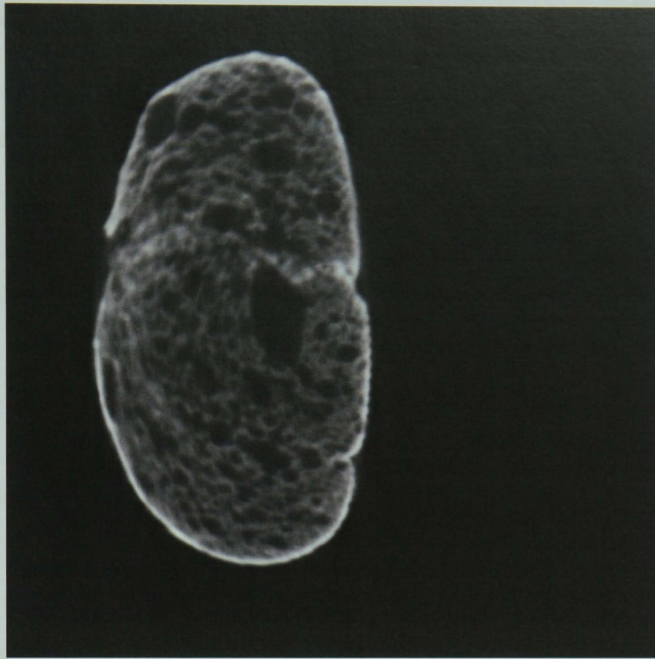
Figure 2.6: The reconstructed slice from the sinogram in Figure 2.5 reveals the internal aerated structure of the bread.
