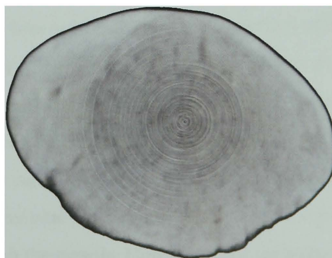
Figure 4.8: An example of ring artifacts in a reconstructed slice from a fossilised piece of whalebone.
