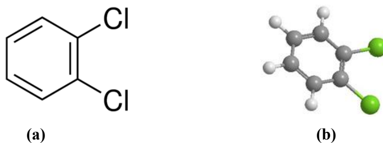
Figure 4.1. The chemical structure of 1,2-dichlorobenzene (a) The structural formula (b) the model of DCB (acquired from https://en.wikipedia.org/wiki/1,2-Dichlorobenzene )
