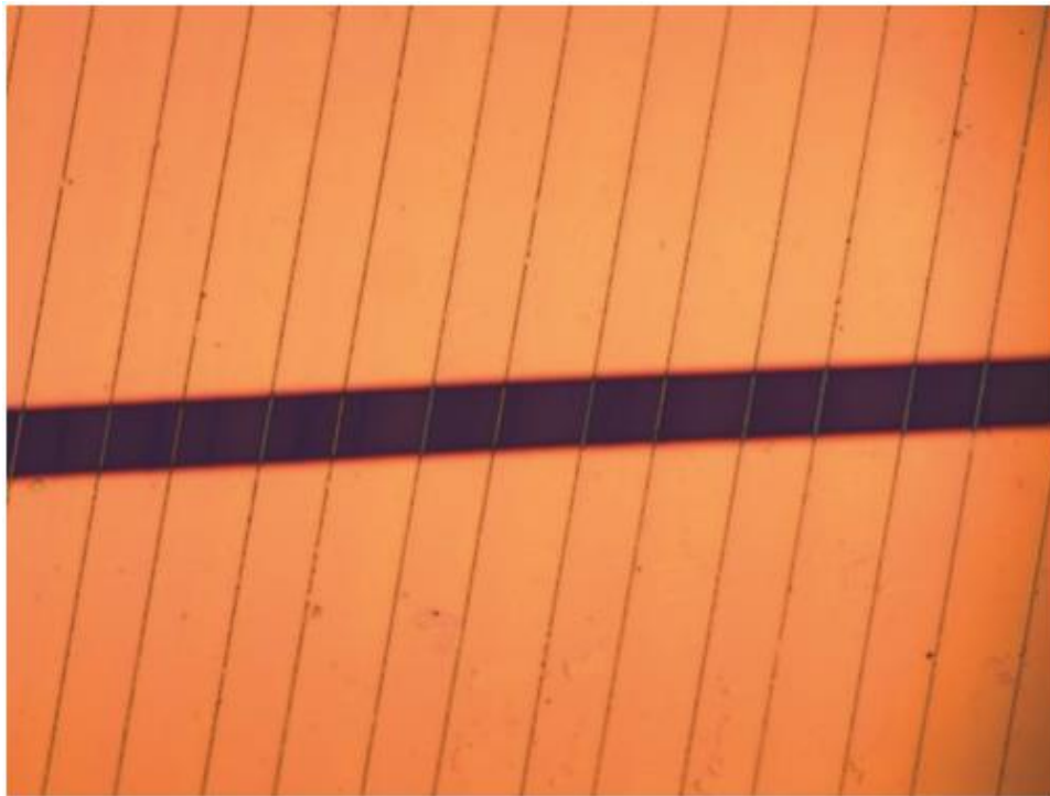
Figure 5.9. The optical image of bottom-gate poly(3,3''-didodecylquaterthiophene) (PQT-12) field-effect transistor
