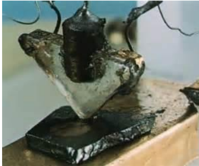
Figure 1.1. Photograph of the prototype of the point-contact transistor that was invented by Bardeen and Bartain in December 1947. A strip of gold foil, slit along one edge is pressed down into the surface of a germanium slab by a polystyrene wedge, forming two closely spaced contacts to this surface [3].
