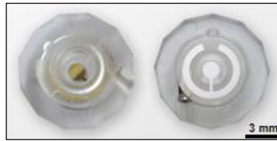
Figure 2.2.1.1. Top (left) and bottom (right) views of a SURFE2R N1 sensor chip, featuring a 3 mm-wide well. At its bottom lies a thin gold electrode coated with a hybrid biomimetic SSM to which the cell membrane preparations adhere (adapted from Nanion Technologies GmbH, 2016a).
