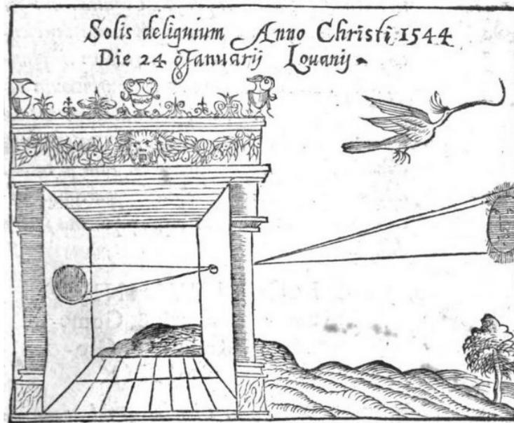
**Fig. 3.1:** representation of the camera obscura from *De radio astronomico et geometrico* [51:39]
