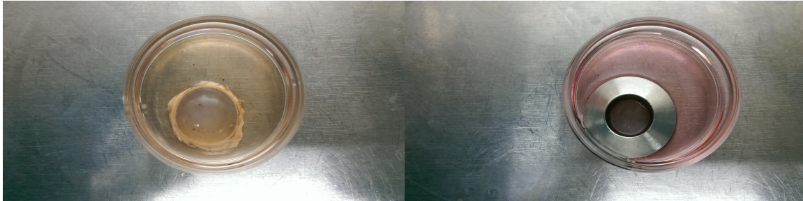
Figure 3.12: Cornea button prepared for imaging (left) and stainless steel ring placed on top of cornea to contain the cells embedded with SPIO nanoparticle.
