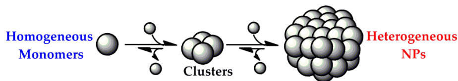
Figure 42: Scheme to illustrate the equilibria between the palladium monomers, clusters, and nanoparticles in solution during palladium catalysis.
