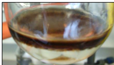
Figure 197: Dark brown, translucent THF layer, which forms after the Suzuki-Miyaura coupling of 4-bromo-6-methyl-pyran-2-one with 4-methylphenylboronic acid to form 6-methyl-4-(4-methylphenyl)-pyran-2-one, using the [\text{Pd}_3(\text{PPh}_3)_4][\text{BF}_4]_2 catalyst.
