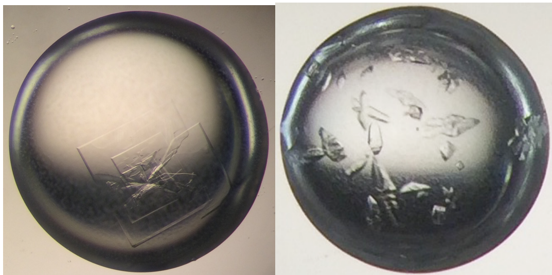
Figure 106 – Optimised crystals of AspRedAm in conditions containing: (left) 0.2 M lithium sulphate, 0.1 M BisTris pH 6.5, 27% (w/v) PEG 3350, 10 mM NADPH and 10 mM rac -rasagiline, and (right) 0.2 M lithium sulphate, 0.1 M BisTris pH 6.5, 27% (w/v) PEG 3350, 5 mM NADP + and 5 mM rac -rasagiline
