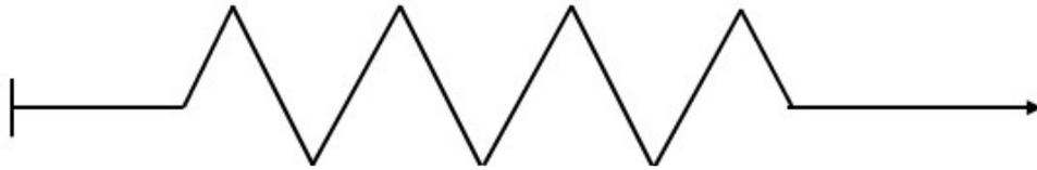
Figure 2-11: The Hookean spring: This perfect spring provides a model for elastic behaviour. Deformation is proportional only to force [109]
