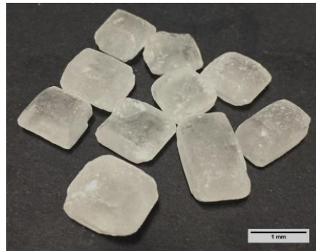
Figure 3-3. Large sucrose crystals used for contact angle measurements.
