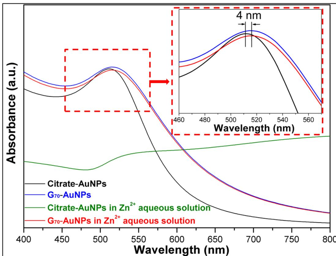
**Figure 6.4.** Visible absorption spectra recorded for as-synthesised citrate-AuNPs or G<sub>70</sub>-AuNPs in either water or an aqueous solution of 15 mM Zn(NO<sub>3</sub>)<sub>2</sub>. The inset shows that the surface plasmon band for G<sub>70</sub>-AuNPs is red-shifted by 4 nm compared to citrate-AuNPs. Notably, there is no further change in the presence of 15 mM zinc ions, indicating good colloidal stability for the G<sub>70</sub>-AuNPs under these conditions.
