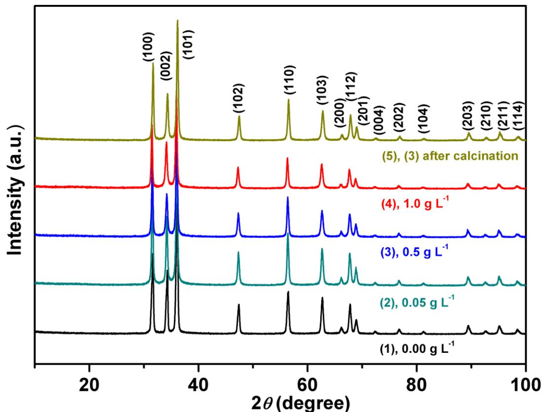
**Figure 5.9.** XRD patterns obtained for ZnO particle prepared in the presence of various S<sub>73</sub>-B<sub>300</sub> nanoparticle concentrations.
