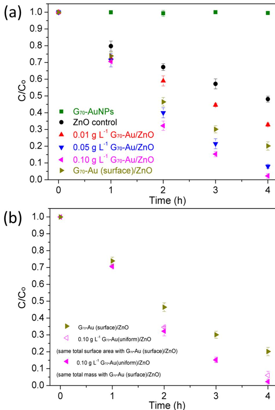
**Figure 6.15.** The rate of photocatalytic dye decomposition recorded for RhB in the presence of  $G_{70}$ -Au(surface)/ZnO and  $0.10 \text{ g L}^{-1} G_{70}$ -Au(uniform)/ZnO. The amount of  $0.10 \text{ g L}^{-1} G_{70}$ -Au(uniform)/ZnO crystals used in these experiments was reduced to produce approximately the same total surface area as that for the  $G_{70}$ -Au (surface)/ZnO crystals, but this had almost no discernible effect on the observed rate of dye decomposition.
