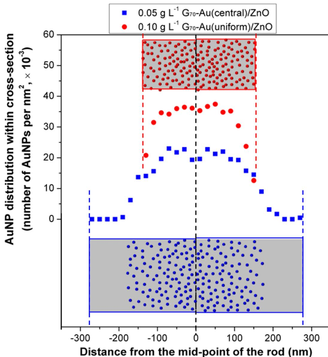
**Figure 6.9.** Comparison of the AuNP distribution within the cross-section of G<sub>70</sub>-Au(central)/ZnO and G<sub>70</sub>-Au(uniform)/ZnO rods. Note: schematic cartoons are drawn to approximate scale.
