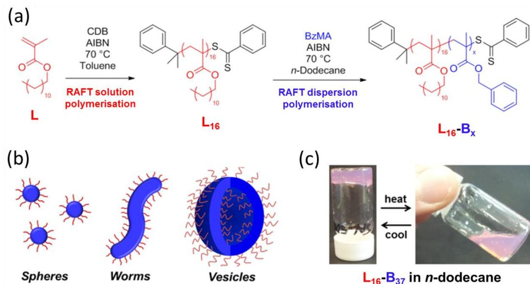
**Figure 1.18.** (a) RAFT dispersion polymerisation synthesis of poly(lauryl methacrylate)<sub>16</sub>-poly(benzyl methacrylate)<sub>x</sub> (**L<sub>16</sub>-B<sub>x</sub>**) diblock copolymer nano-objects; (b) Cartoons depicting spheres, worms or vesicles; (c) thermo-responsive behavior of a 20% w/w dispersion of **L<sub>16</sub>-B<sub>37</sub>** diblock copolymer nanoparticles from a free-standing worm gel at 20 °C to a dispersion of spheres on heating to 70 °C in *n*-dodecane.<sup>126</sup>
