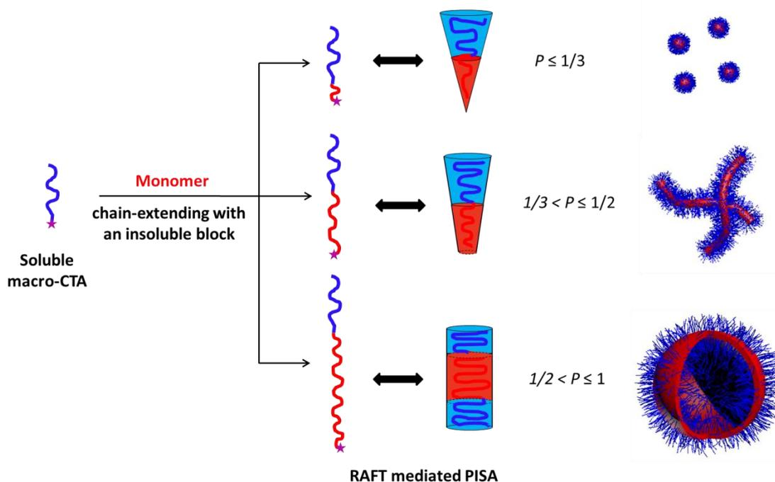
**Figure 1.13.** Schematic representation of the synthesis of diblock copolymer nano-objects via PISA. The macro-CTA is soluble in the continuous phase, which can be polar solvents (such as water, ethanol) or non-polar solvents (such as *n*-alkanes).<sup>27</sup>
