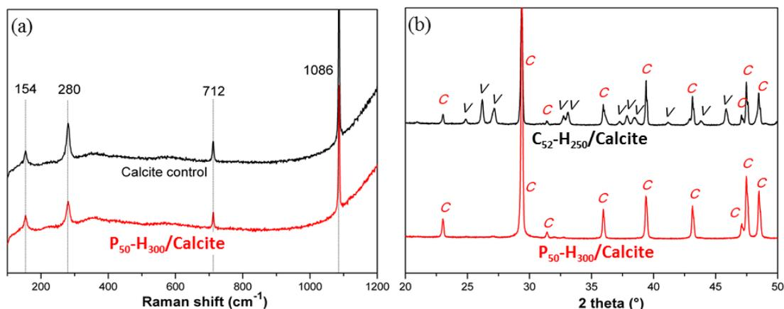
**Figure 3.10.** (a) Raman spectra recorded for a calcite crystal control and calcite containing occluded P<sub>50</sub>-H<sub>300</sub> nanoparticles; (b) XRD patterns recorded for calcite precipitated in the presence of C<sub>52</sub>-H<sub>250</sub> (C denotes calcite and V de-notes vaterite) and P<sub>50</sub>-H<sub>300</sub>.
