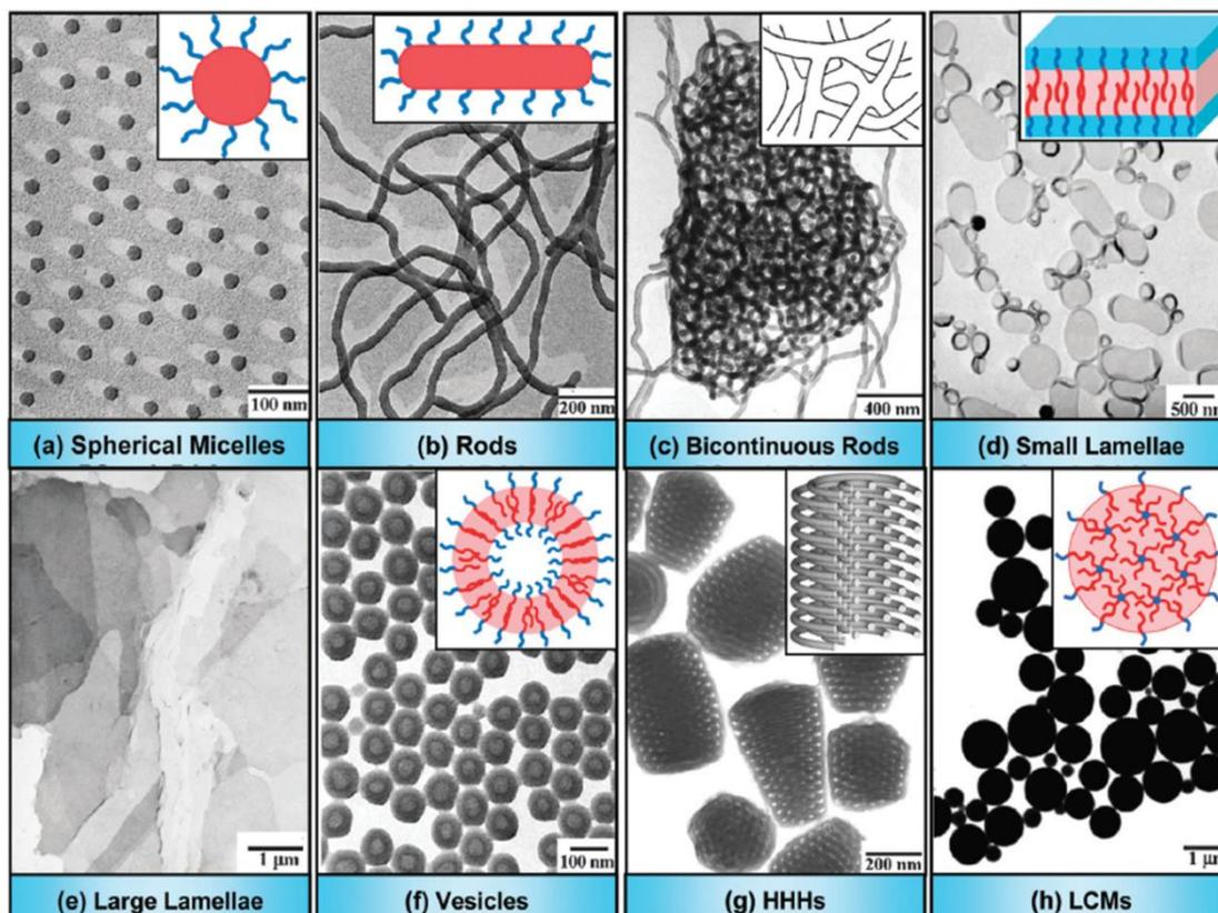
**Figure 1.12.** Transmission electron microscopy (TEM) images and corresponding cartoons for a range of copolymer morphologies formed by the self-assembly of asymmetric amphiphilic polystyrene-poly(acrylic acid) diblock copolymers in selective solvents ( $x$  and  $y$  represent the DPs of the PS and PAA blocks, respectively). In the cartoons, red denotes the hydrophobic PS block, while blue represents the hydrophilic PAA block.<sup>97</sup>
