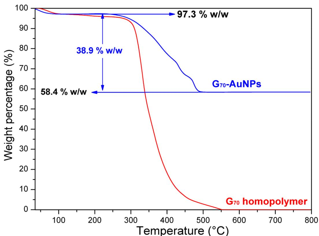
**Figure 6.3.** TGA of G<sub>70</sub> homopolymer (red) and G<sub>70</sub>-AuNPs (blue). As expected, G<sub>70</sub> homopolymer is pyrolysed completely above 550 °C. Given the presence of 2.7 % w/w water in the G<sub>70</sub>-AuNPs trace, the G<sub>70</sub> content in G<sub>70</sub>-AuNPs can be calculated to be 40.0 % w/w.
