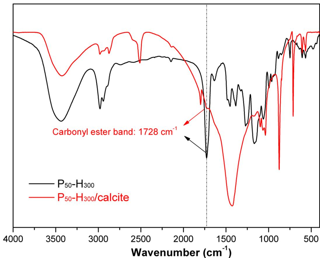
**Figure 3.12.** FT-IR spectra recorded for P<sub>50</sub>-H<sub>300</sub> nanoparticles alone and P<sub>50</sub>-H<sub>300</sub>/calcite nanocomposite crystals. A weak carbonyl ester band at 1728 cm<sup>-1</sup> is discernible in latter spectrum, confirming successful occlusion of copolymer nanoparticles within the calcite crystals.
