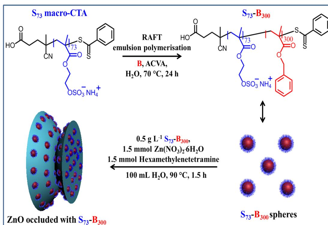
**Scheme 5.1.** RAFT aqueous emulsion polymerisation of benzyl methacrylate (B) using a  $S_{73}$  macro-CTA at 70 °C to produce  $S_{73}$ - $B_{300}$  diblock copolymer nanoparticles and associated cartoon showing  $S_{73}$ - $B_{300}$  spherical nanoparticles and their occlusion within ZnO.<sup>27</sup>
