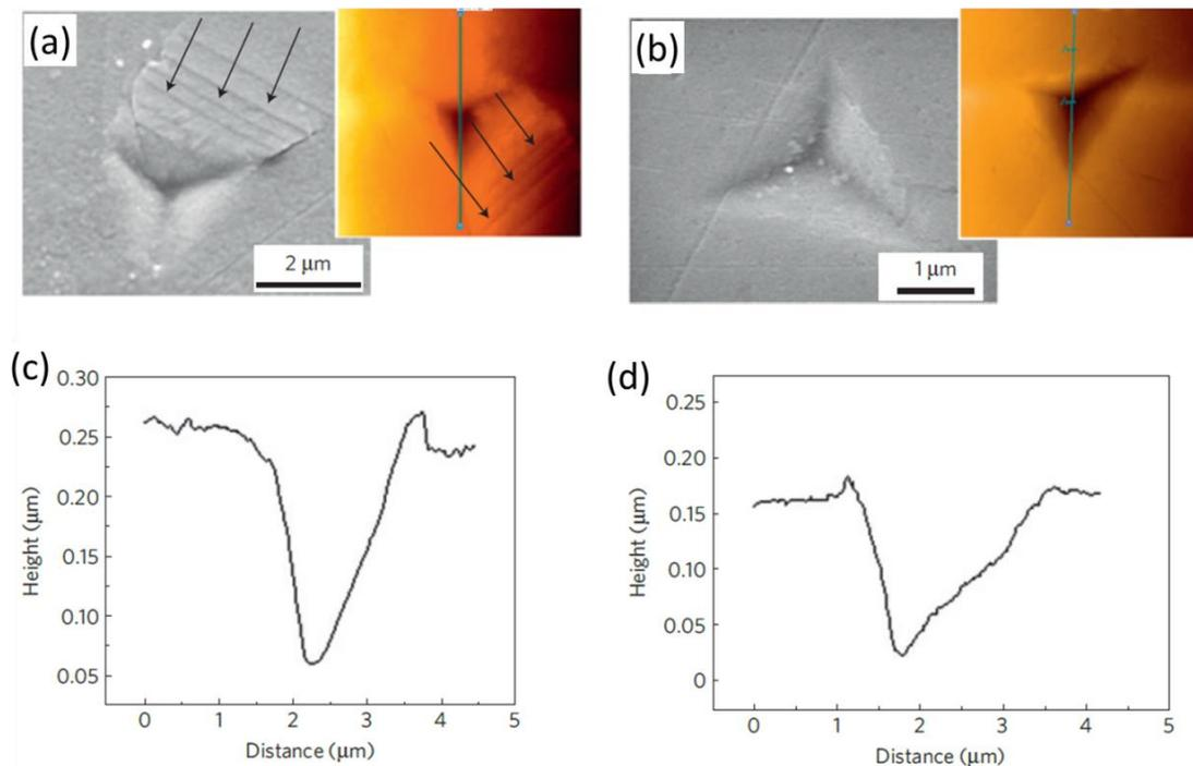
**Figure 1.26.** SEM and AFM images obtained for pure calcite (a) and nanocomposite crystals (b); AFM profiles of nano-indentation marks on a calcite control crystal (c) and a nanocomposite crystal after nanoindentation (d). Step formation around the indent in pure calcite was observed, as indicated by the arrows. However, this was not observed for the nanocomposite crystal.<sup>7</sup>
