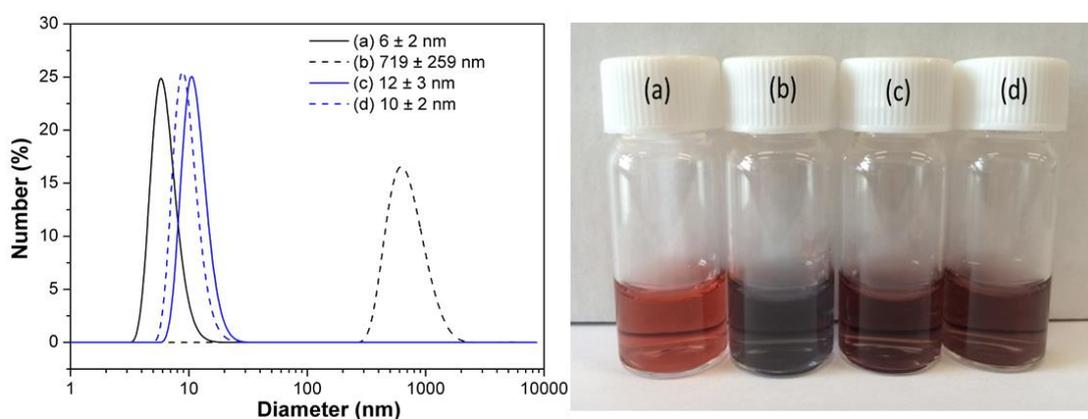
**Figure 6.2.** Mean hydrodynamic number-average diameter (left-hand) and optical photograph (right-hand) obtained for aqueous dispersions of (a) citrate-stabilised AuNPs (gold nanoparticles prepared using sodium citrate); (b) citrate-stabilised AuNPs in the presence of 15 mM zinc ions; (c)  $G_{70}$ -AuNPs; (d)  $G_{70}$ -AuNPs in the presence of 15 mM zinc ions.
