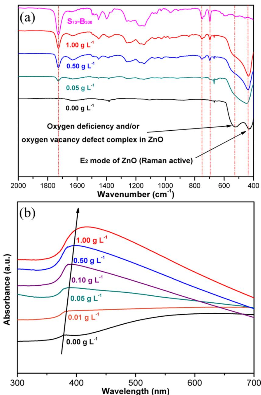
**Figure 5.8.** (a) FT-IR spectra recorded for ZnO nanocomposites prepared using various S<sub>73</sub>-B<sub>300</sub> nanoparticle concentrations and also a reference spectrum for S<sub>73</sub>-B<sub>300</sub> nanoparticles alone. (b) UV-visible absorption spectra recorded for ZnO particles prepared in the presence of various S<sub>73</sub>-B<sub>300</sub> nanoparticle concentrations after calcination.
