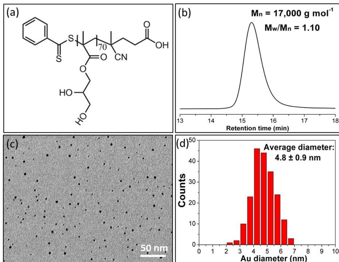
**Figure 6.1.** Characterisation of poly(glycerol monomethacrylate)<sub>70</sub> (G<sub>70</sub>) and G<sub>70</sub>-stabilised AuNPs. (a) Chemical structure of the G<sub>70</sub> polymeric stabiliser used in this work; (b) GPC data obtained for G<sub>70</sub> using a series of poly(methyl methacrylate) calibration standards; (c) representative TEM image obtained for G<sub>70</sub>-AuNPs; (d) particle size distribution determined for G<sub>70</sub>-AuNPs from TEM image analysis.
