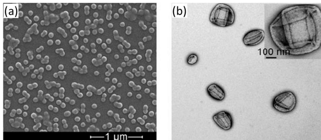
**Figure 1.14.** (a) Scanning electron microscopy (SEM) image of poly(glycerol monomethacrylate)<sub>65</sub>-poly(2-hydroxypropyl methacrylate)<sub>300</sub> (G<sub>65</sub>-H<sub>300</sub>) spheres prepared at 10 % solids. (b) TEM image of G<sub>65</sub>-H<sub>300</sub> vesicles prepared at 20 % solids.<sup>31</sup>
