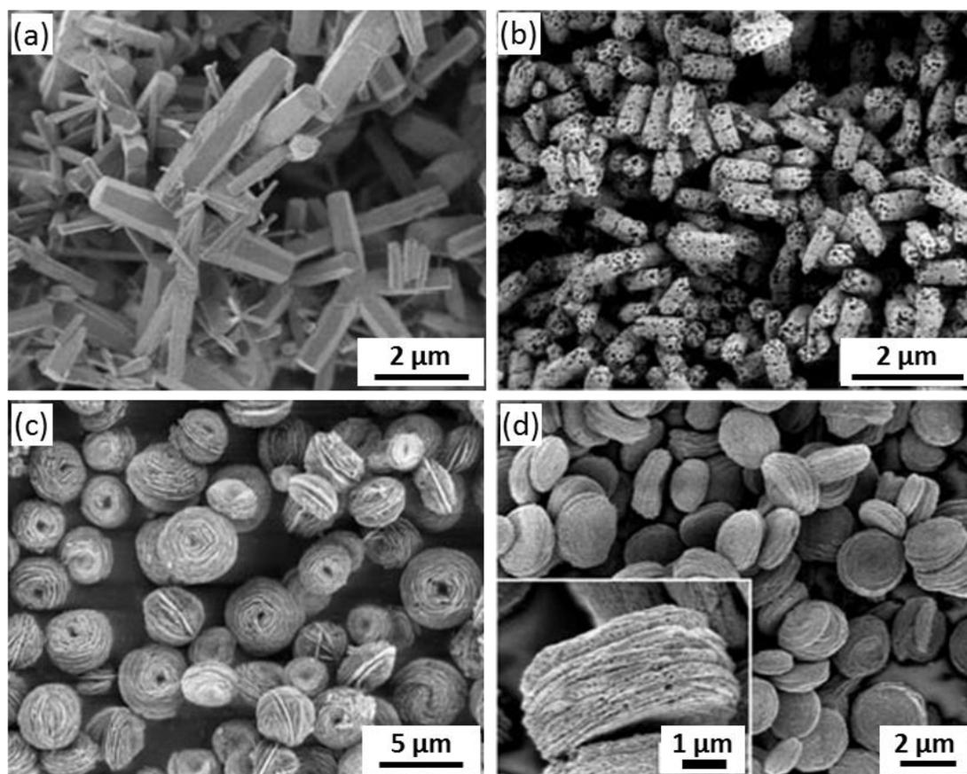
**Figure 1.27.** Zinc oxide samples crystallised (a) without additive; (b)  $6 \text{ g L}^{-1}$  polystyrene latex surface-functionalised with acrylic acid; (c)  $6 \text{ g L}^{-1}$  polystyrene latex surface-functionalised with maleic acid; (d)  $6 \text{ g L}^{-1}$  polystyrene latex surface-functionalised with ethylene glycol methacrylate phosphate.<sup>173</sup>
