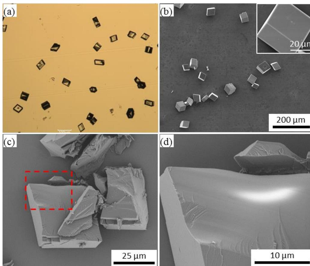
**Figure 3.7.** Calcium carbonate crystals prepared in the absence of any additives. (a) optical micrograph; (b) SEM image; (c) SEM image showing the crushed crystal; (d) magnified SEM image showing the dashed rectangle area indicated in (c). Note: the crystallisation was conducted at an initial pH of 9.5.
