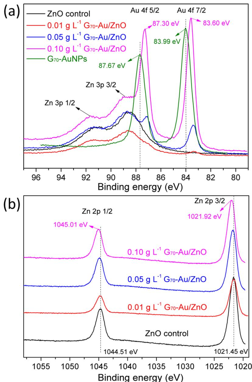
**Figure 6.14.** High resolution X-ray photoelectron spectra recorded for various G<sub>70</sub>-Au/ZnO nanocomposite crystals and appropriate reference materials: (a) Au4f; (b) Zn2p.
