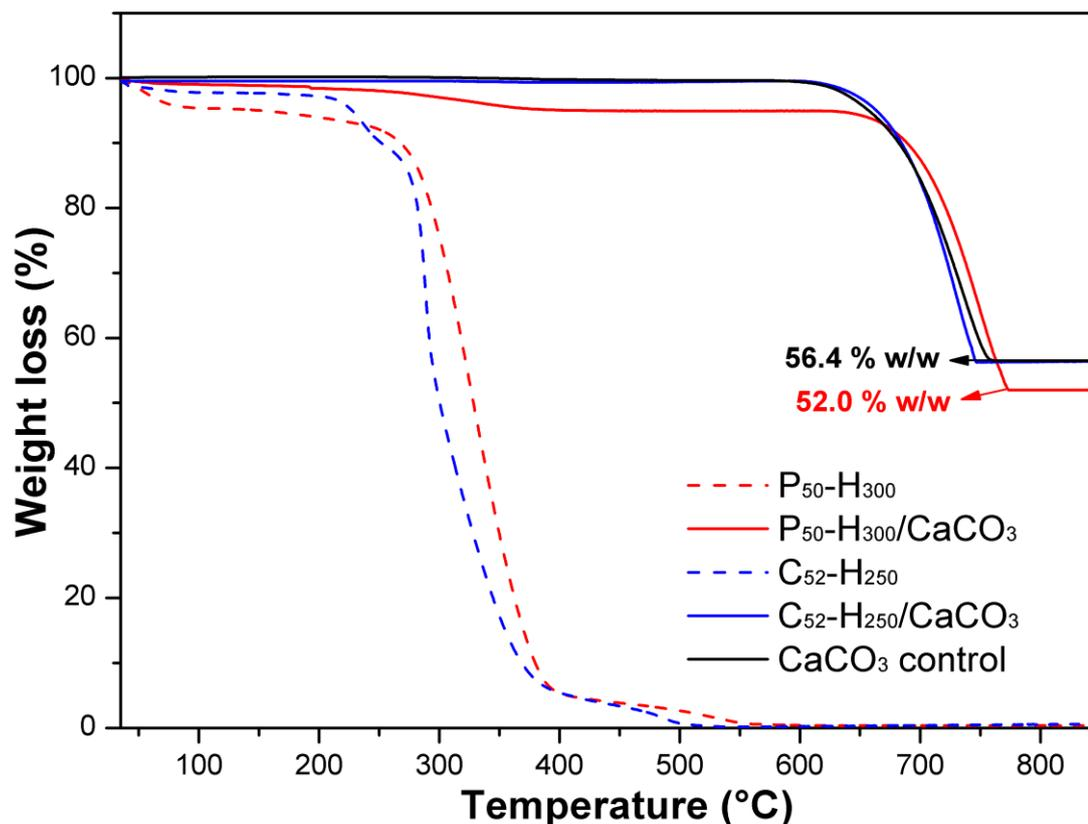
**Figure 3.11.** TGA curves recorded for  $\text{P}_{50}\text{-H}_{300}$  and  $\text{C}_{52}\text{-H}_{250}$  nanoparticles alone, calcite crystals grown in the presence of either  $\text{C}_{52}\text{-H}_{250}$  or  $\text{P}_{50}\text{-H}_{300}$ , and a pure calcite control.
