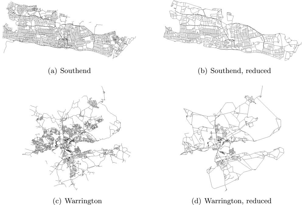
Figure 9.8: Original maps and reduced graphs for Southend and Warrington road networks, illustrating grid-like and tree-like road networks.
