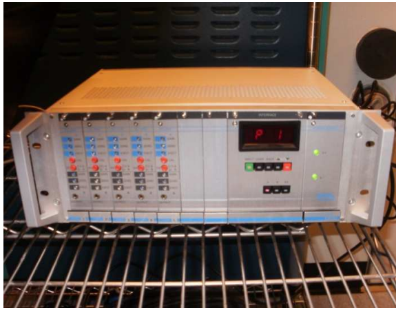
Figure 5.9: Load cell, platform & tray Figure 5.10: Modular 600 Data logger
