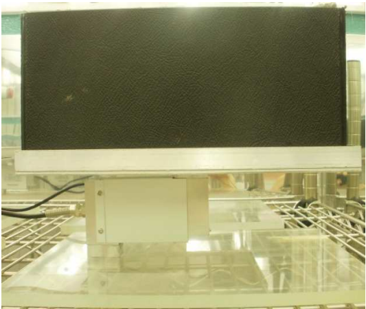
Figure 5.9: Load cell, platform & tray Figure 5.10: Modular 600 Data logger
