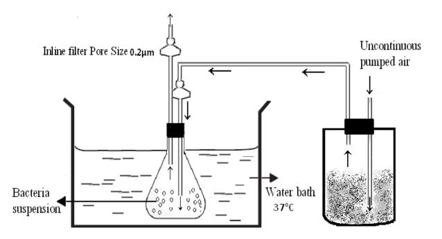
Figure 5.2: Airtight container contains 600 g of the blue blow fly larvae (*Calliphora quadrimaculata*) fed on beef heart; larval fumes were pumped un-continuously from the jar into a flask contained 200 ml of *Mycobacterium phlei* suspension through silicone tube. Pumped air was sterilized by inline filters pore size  $0.2\mu$ m fixed to silicone tube. The flasks were placed and fixed in a water bath at 37°C for 16 h.
