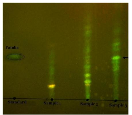
Figure 6.4: TLC plate showing that patulin was detected in sample number 3 (extracted from liquid culture of fungus isolated from apple). TLC plate sprayed with 0.5 ml *p*-anisaldehyde in 85 ml of methanol containing 10 ml of glacial acetic acid and 5 ml of concentrated sulphuric acid, heated at 110°C for 10 min and observed under UV light (300–360 nm). (Left to right) Three samples and one standard are shown.
