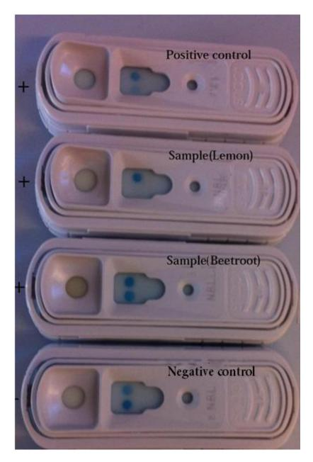
Figure 6.3: SNAP devices showing different results according to samples sources. Note in positive control, lemon and beetroot samples the control spot are darker than the sample spot (positive results), whereas in the negative control (sterilized Czapek Dox liquid medium) control spot was lighter than the sample spot.
