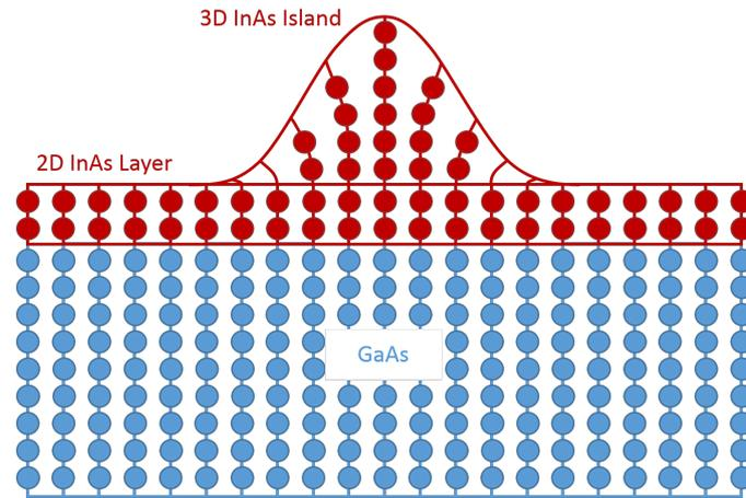
Figure 2.2: Illustration of the structure of an InAs/GaAs SAQD.
