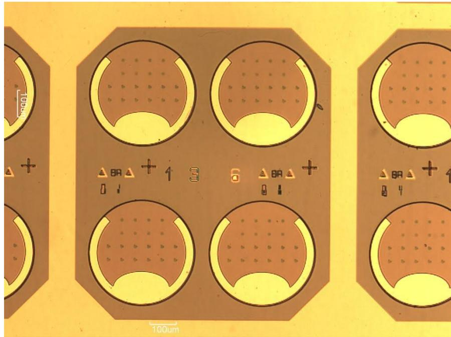
Figure 3.7: Micrograph of the fabricated sample surface. Four complete mesas each corresponding to a single  $p-i-n$  diode are visible in the centre of the image. The smaller features within each diode are PhCs. Image courtesy of Christopher Bentham and reproduced with permission.
