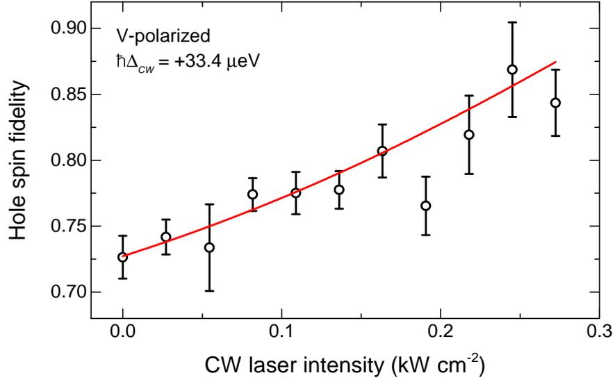
Figure 4.18: Hole spin initialisation fidelity of QD C vs. CW laser intensity for a V-polarized CW laser at  $E = -72 \text{ kV cm}^{-1}$  to maximize photocurrent detection efficiency. The line is a fit of the model (Equation 4.20) incorporating the variation of  $\delta$  with CW laser intensity (see appendix A.1 for full details).
