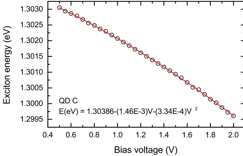
Figure 4.7: Example plot of exciton energy (extracted from single pulse photocurrent spectra) vs. bias voltage for QD C. The data agrees well with a quadratic fit of the form of Equation 2.4 (red line) allowing accurate conversion from bias voltage to energy for high resolution photocurrent spectroscopy.
