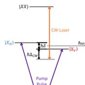
Figure 4.15: Illustration of the OSE scheme using the QD energy levels in the linear basis. The neutral exciton eigenstates ( $X_{H/V}$ ) are split by  $\hbar\delta$ . The CW laser is  $V$ -polarized and positively detuned from the  $X_V \rightarrow XX$  transition by  $\Delta_{CW}$ . The pump pulse addresses both exciton levels owing to its circular polarization and  $\text{FWHM} \gg \hbar\delta$ .
