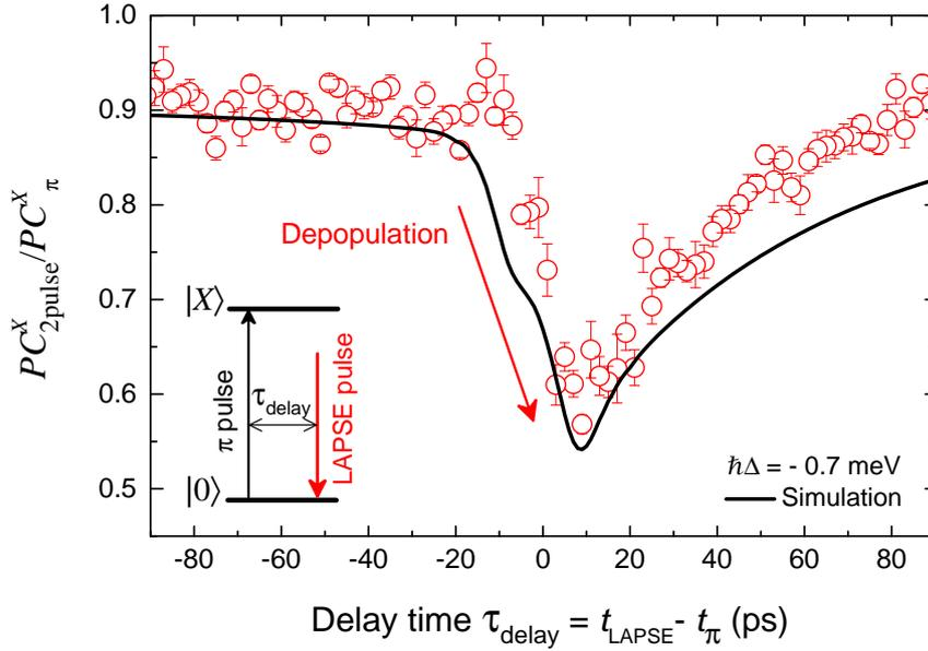
Figure 5.10: Time dynamics of the LAPSE process. Red circles:  $PC_{2\text{pulse}}^X/PC_{\pi}^X$  measured as a function of  $\tau_{\text{delay}}$  using the same pulse configuration as Figure 5.9.  $\tau_{\text{delay}} = t_{\text{LAPSE}} - t_{\pi}$ , where  $t_{\text{LAPSE}}$  and  $t_{\pi}$  are the arrival times of the LAPSE pulse and the  $\pi$  pulse. The pulse area of the LAPSE pulse is  $5.25\pi$ . Black line: Numerical simulation. Inset: Excitation scheme.
