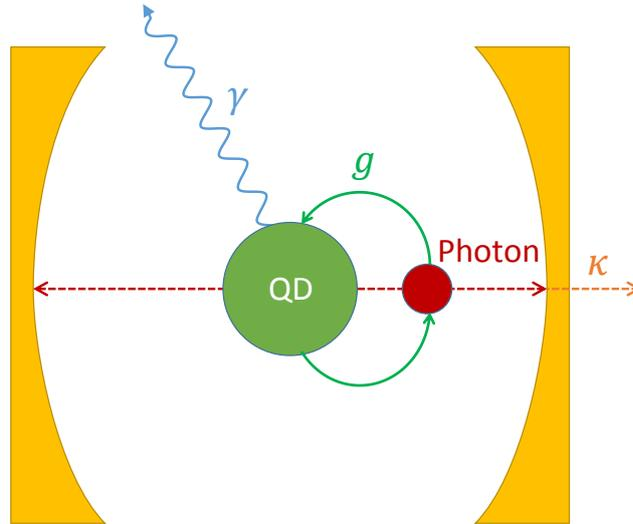
Figure 2.15: Schematic illustrating the key parameters of a coupled cavity-QD system. The strength of the interaction between the cavity photons and the QD is defined by the coherent coupling strength  $g$ . The rate of leakage from the cavity mode is defined as  $\kappa$  whilst  $\gamma$  is a rate incorporating both decay and dephasing of the QD state.
