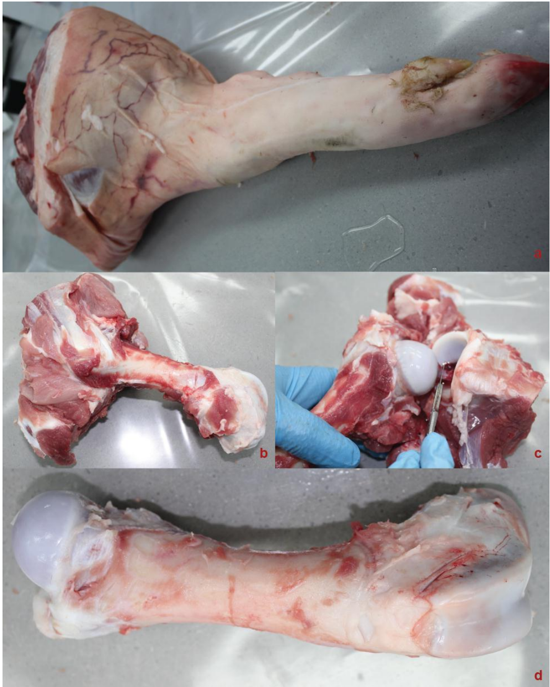
Figure 3-2 - (a) A porcine leg as received from the abattoir. (b) Tissue stripped from the leg. (c) Ligamentum teres being cut to separate the femoral head from the acetabulum. (d) Stripped porcine femur.
