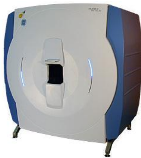
Figure 3-6 – XtremeCT scanner by Scanco used for obtaining CT images from the bone samples (“XtremeCT scanner,”)
