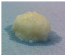
Figure 5-5 - A sample treated in KOH for 7 days. The sample had lost its solid structure, swelled and was destroyed in handling.
