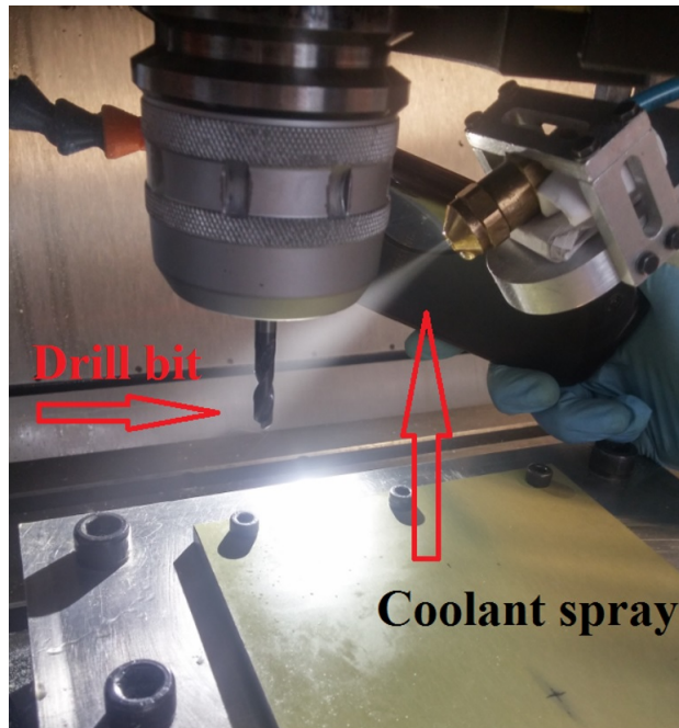
Figure 3.5: Schematic representation of the nozzle holder fitted inside the CNC machine
