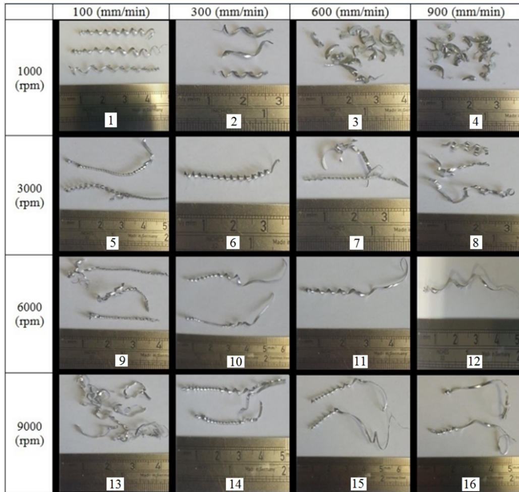
Figure 5.29: Chip shapes produced when drilling GLARE 2B
