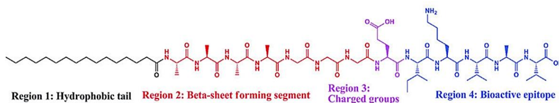
Fig. 1-25 IKVAV-containing peptide amphiphile molecule and its self-assembly into nanofibers, by Stupp. 117
