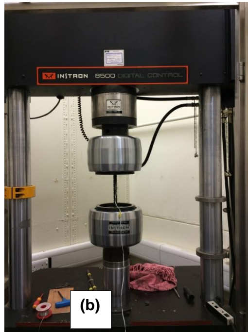
Photo 3-5: (a) Prepared samples of plates and reinforcing bars and (b) tensile test machine
