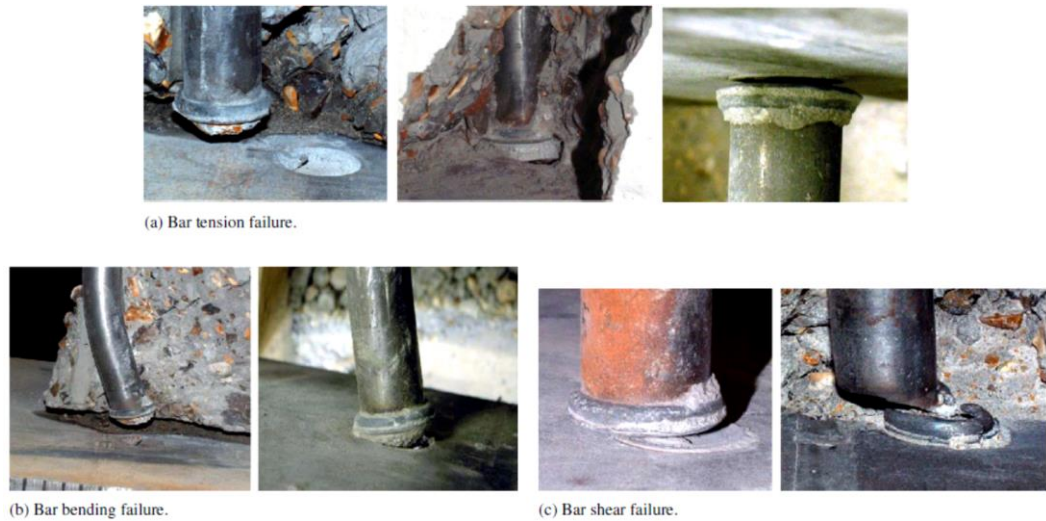
Figure 2-15: Failure modes in shear connectors (Xie et al., 2007)
