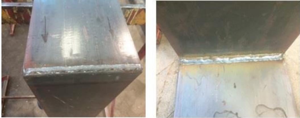
Photo 3-2: Welded joint of the steel plate
