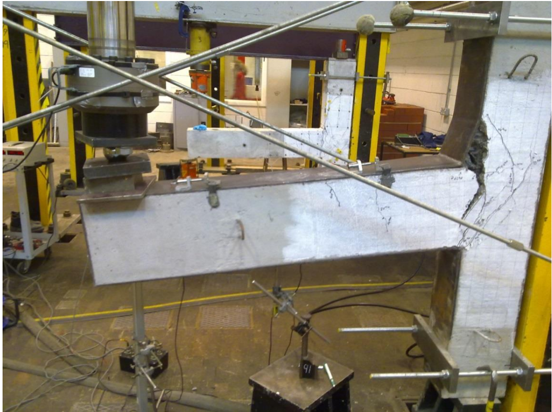
Photo 4-7: Failure of SCS joint with welded bars
