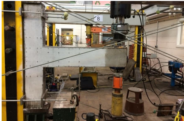
Photo 4-20: Cyclic test arrangement
