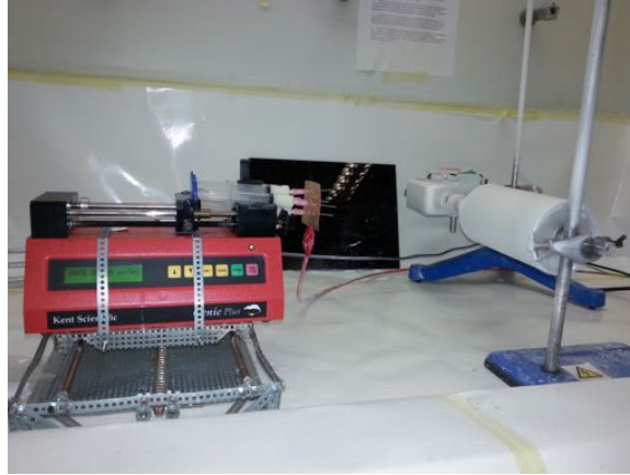
Figure 2.5: The Electrospinning Set-Up in our Lab (used in this thesis)
