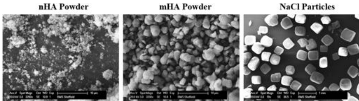
Figure 6.9: SEM of nHA, mHA and NaCl particles used in fabricating PL scaffolds Scale Bar of SEM images = 10\ \mu\text{m} , 10\ \mu\text{m} & 1\ \text{mm}
