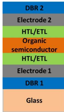
Figure 8-3 – Microcavity OLED working in the strong coupling regime with minimized losses in order to achieve organic polariton condensation.
