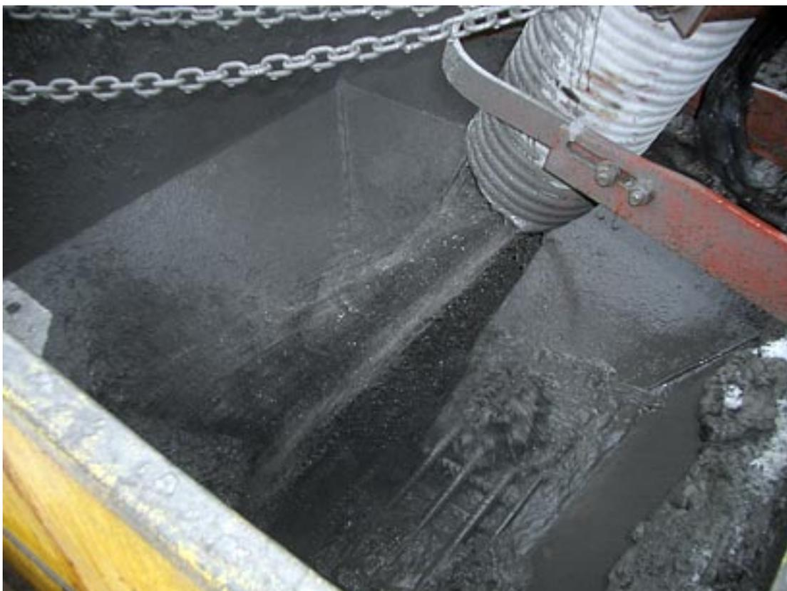
**Figure 1.6:** Process of depositing backfill mine wastes into a surface borehole. Picture reproduced from Engels [20].
