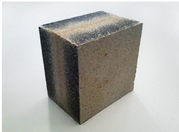
Figure 3.18: Dry medium sand after one-dimensional compression to 800 MPa.
