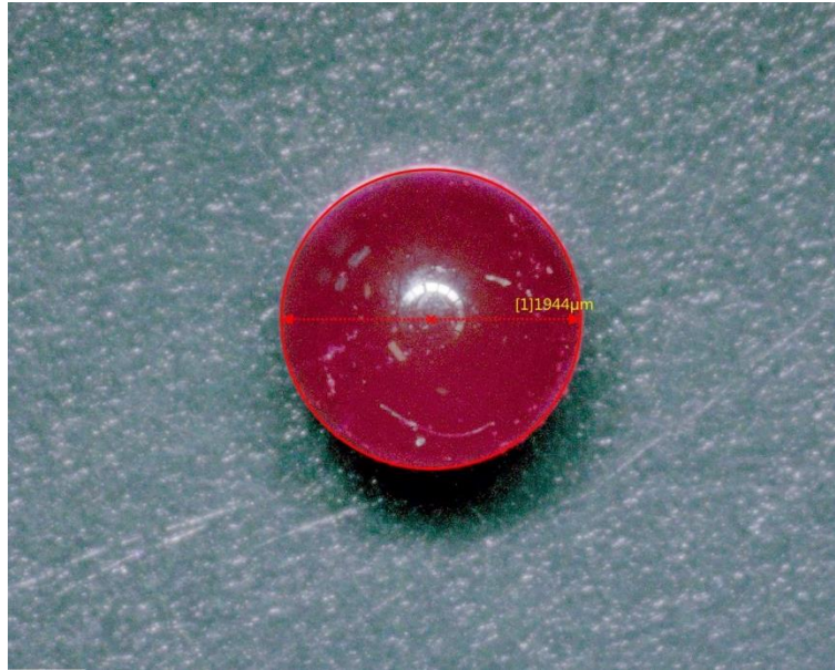
Figure 8-2: Sapphire ball that used as indenter to determine the hardness of the ribbon
