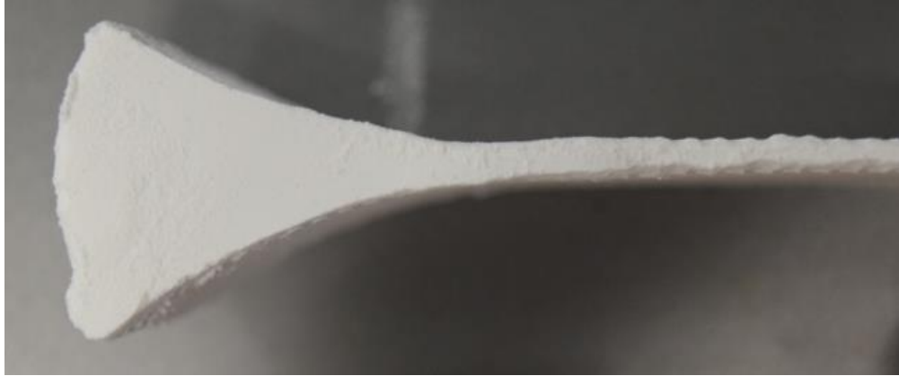
Figure 6-4: Pre-compacted body of Avicel PH-101 and the ribbon
