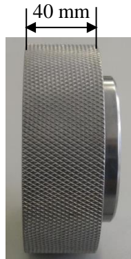
Figure 5-15: Image of the roller showing its width
