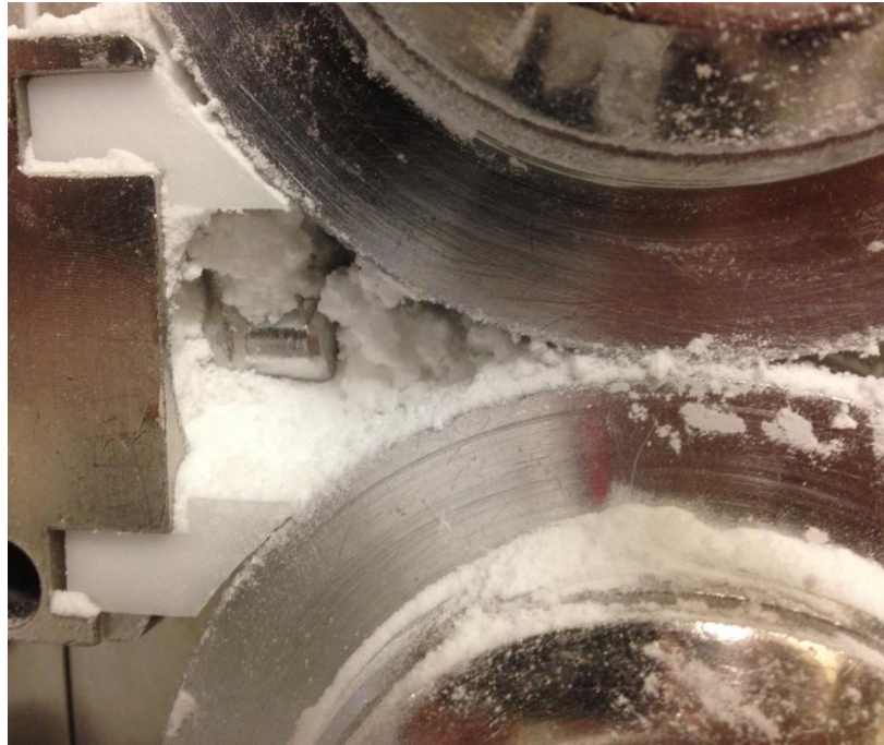
Figure 5-2: Image shows melting of Glucidex®6 between the two rollers
