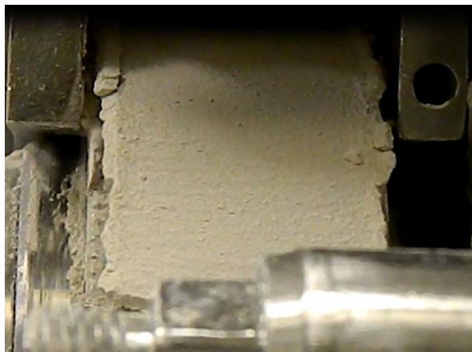
Figure 7-5: Image of calcium carbonate ribbon during compaction showing un-compacted ribbon sides compared to the centre
