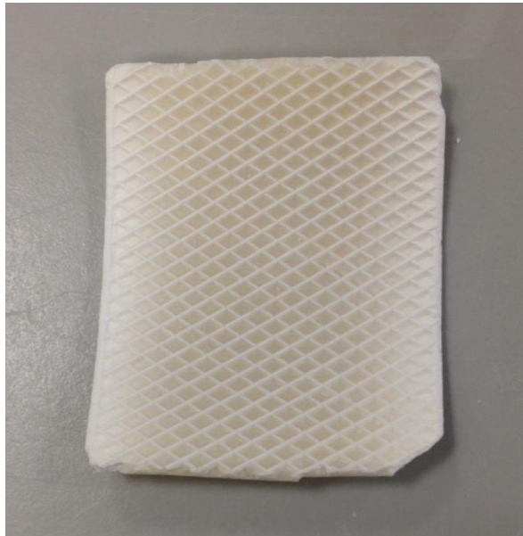
Figure 7-7 : Avicel PH-101 ribbon produced at 150 bar with dark colour at the centre part of the ribbon
