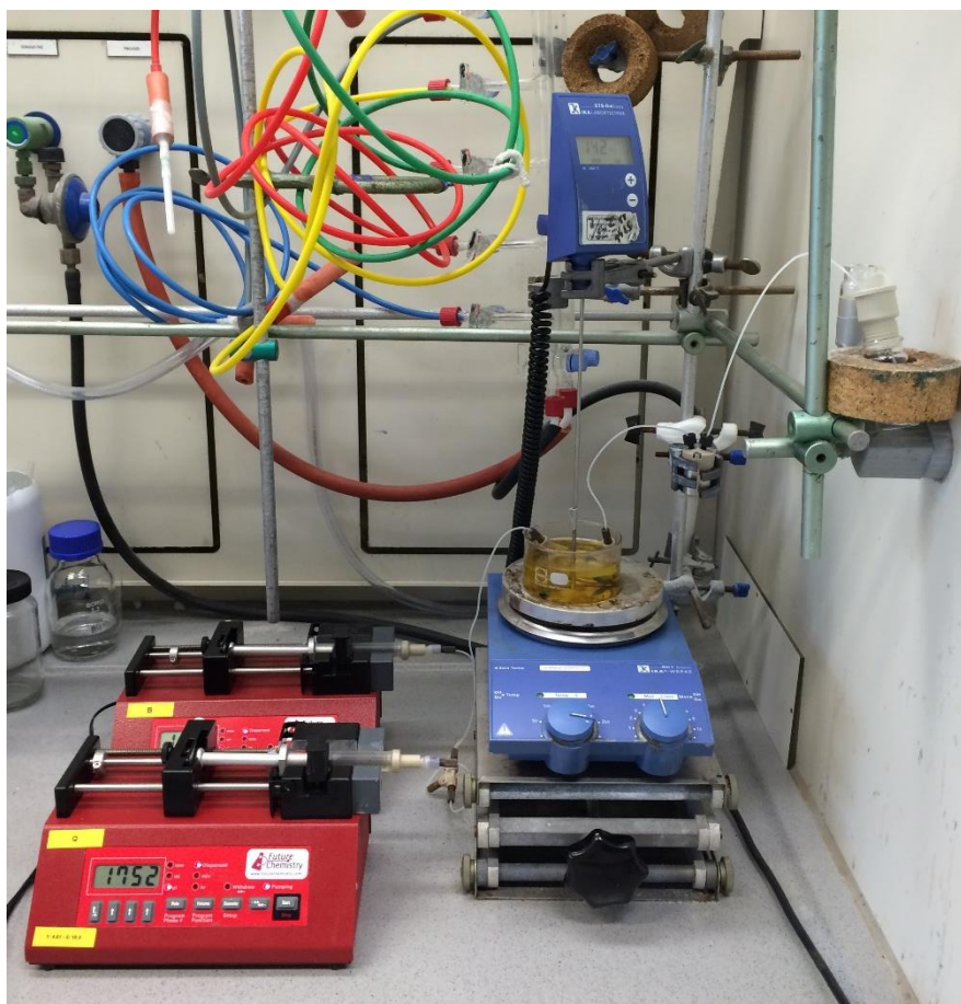
Figure 8. Full flow setup to perform cycloaddition reactions.
