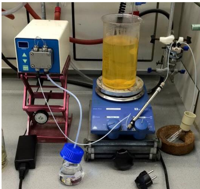
Figure 9. Scaled-up flow system for the cycloaddition reactions.
