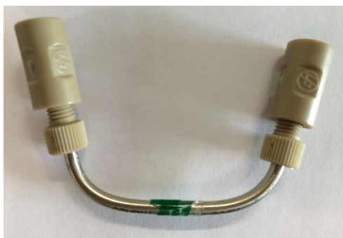
Figure 7. U-shaped stainless steel cartridge packed with supported copper catalyst.
