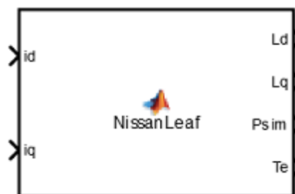
Fig. A.26 Schematic of the polynomial based high fidelity machine model for Nissan-Leaf motor
