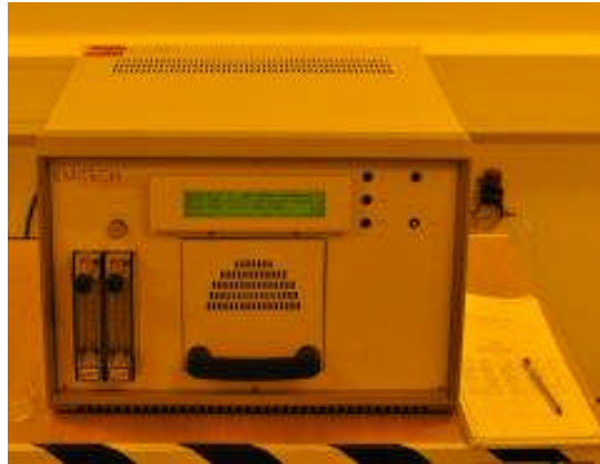
Figure 2-5 Oxygen plasma asher
