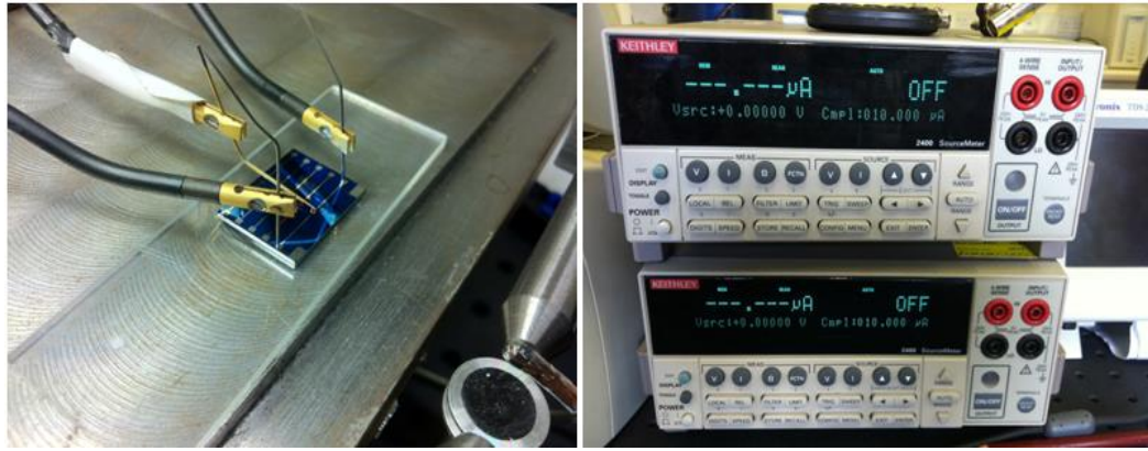
Figure 3-2: Source, drain and gate probes (Left) are connected to Keithley 2400 source measure units (Right) Water gated-TFT.
