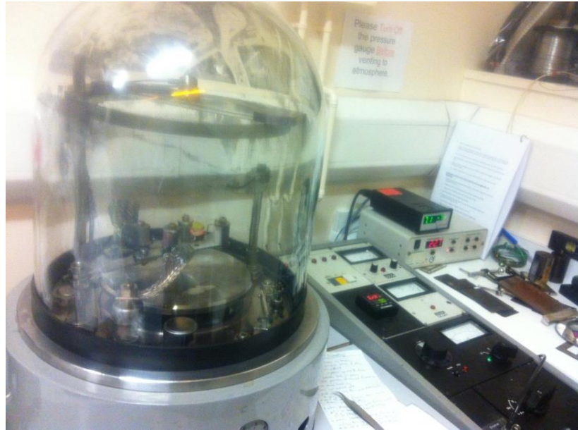
Figure 2-3: Edwards E306 thermal evaporator.
