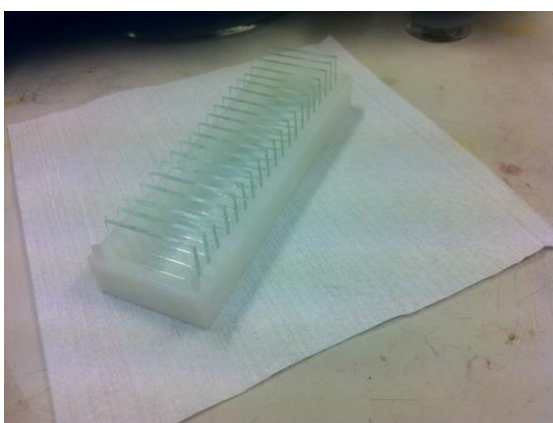
Figure 2-2: Amorphous SiO 2 ('Quartz') substrates after cleaning process
