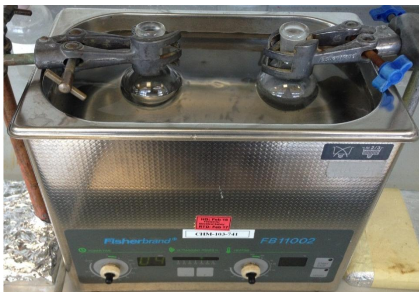
Figure 38: Optimum conditions for the ultrasonic cleaning, with a perfectly smooth water surface
