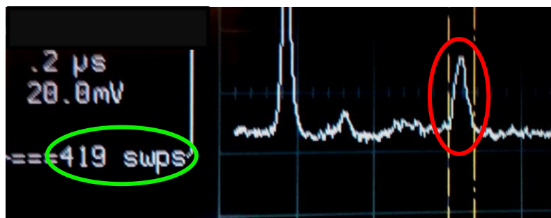
Figure 3.5: A photograph showing the display of the oscilloscope. An example of the OH signal can be shown, circled in red, at t = 200 \mu\text{s} ; whilst circled in green is the number of times the spectrum has been averaged.
