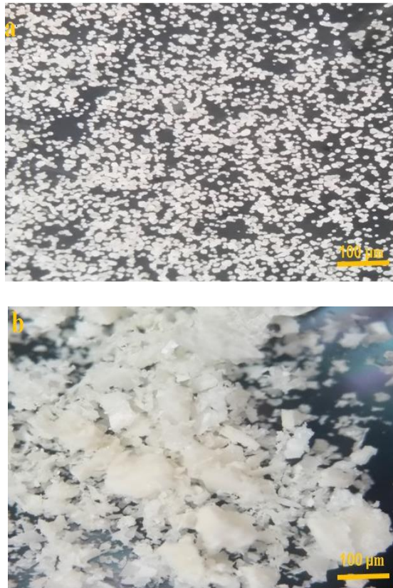
Figure 4.16: Light microscopy images of (a) spray dried and (b) freeze dried powders.
