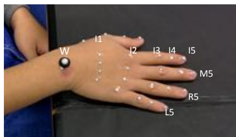
FIGURE 4.5 MARKER SET AND DEFINITION OF THE LOCAL REFERENCE SYSTEM
