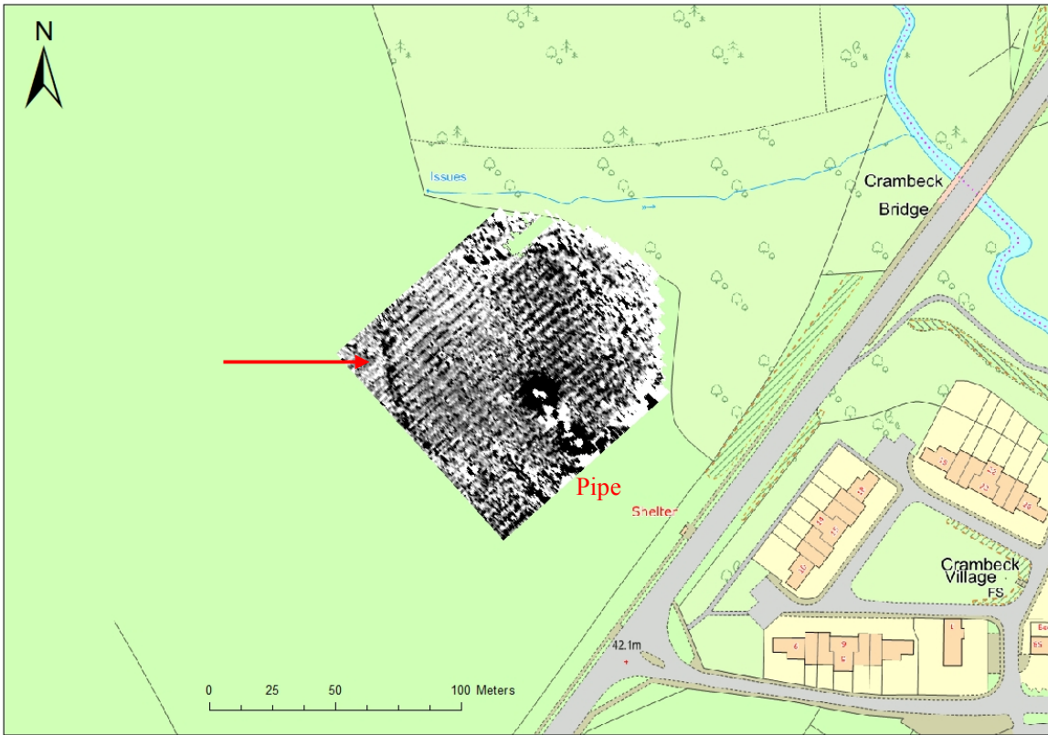
Figure 5 The circular feature is more visible in this image although the interference from the pipe has distorted the results.
