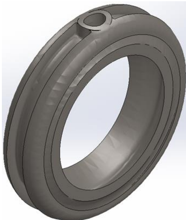
Figure B.32: The deformed shape of the regenerator holders.
