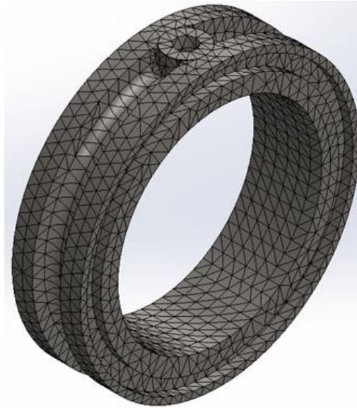
Figure B.29: Solid mesh of the configuration of the regenerator holders.
