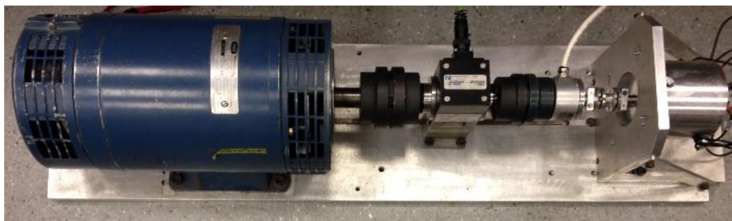
Fig.4.52 Phase winding PWM voltage (CH2), rotor position (CH3) and current (CH4) waveforms of the prototype operating at motor mode at 400rpm and photo of the test rig including DC machine, torque sensor, position sensor and prototype from left to right.
