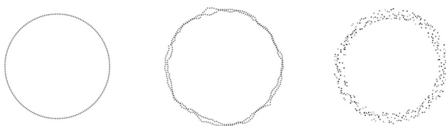
Figures 1a-c. (left to right), a) regular circle with uniform radius; b) circle drawn with two layers of fractal noise deviation applied to radius; c) circle drawn using random deviation applied to radius.
