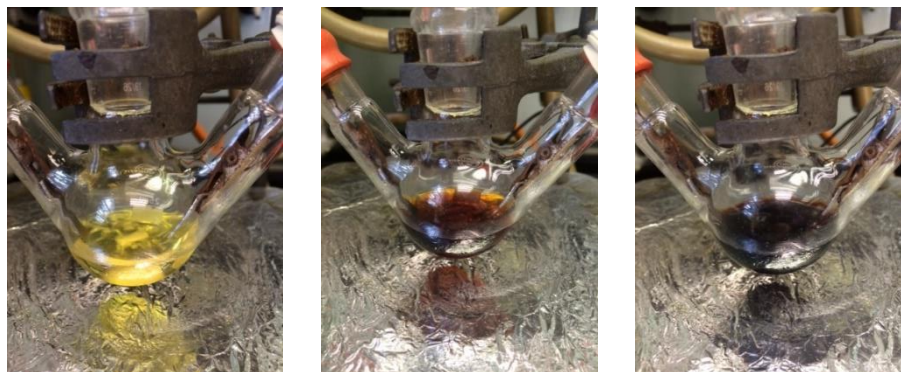
Figure 4.16 Images of inert reaction vessel before electrical potential application (left), during (middle) and after (right), illustrating formation of a purple reaction product, which precipitates from solution over time.
