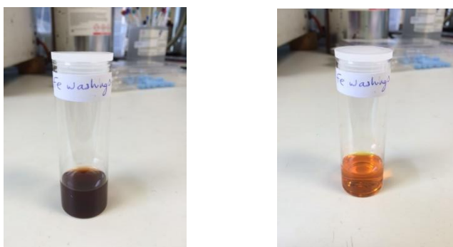
Figure 4.23 Exemplar images of residual Fe II -salen complexes in solution. Left: blanketed by an atmosphere of N 2 , prior to oxidation. Right: the same sample following ca. 10 seconds exposure to air.
