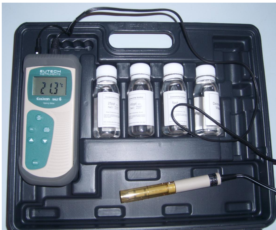
Figure 2.4 The salinity meter used for measuring salinity at sites. A Salinity Meter (Oaklon, Eutech), a microprocessor based, hand held meter which gives +/- 0.5% full scale accuracy and measures NaCl in either percentage or ppm. It includes a conductivity meter (cell constant, K=1), with built in temperature sensor.
