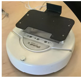
Figure 7.2: Differential drive robot which will be used to perform experimental research on MDAs.
