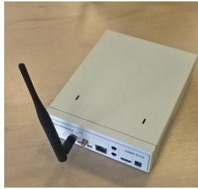
Figure 7.1: Software defined radio which will be used to perform experimental research on MDAs.
