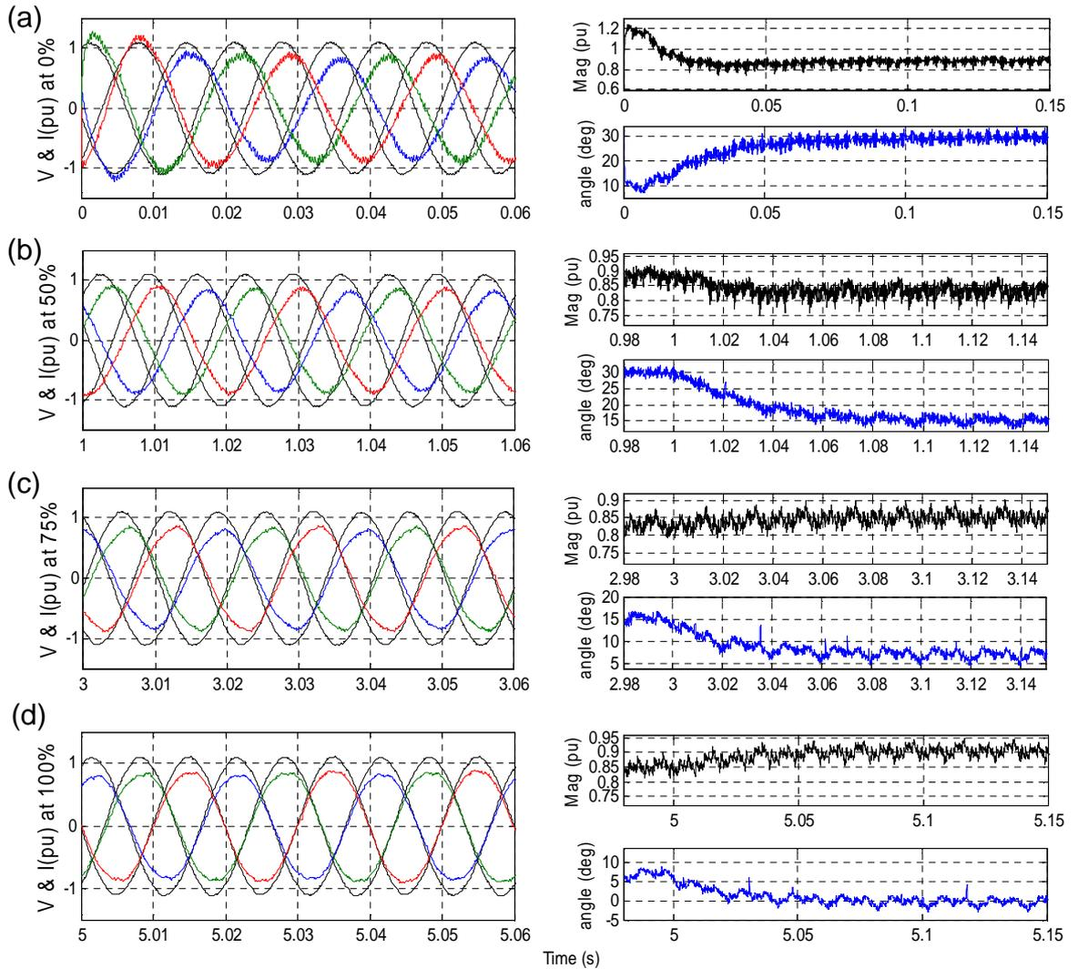
Figure 7.18: Voltage, Current and Power Factor Angle, (a) Zero compensation, (b) 50% compensation, (c) 75% compensation, (d) Full compensation
