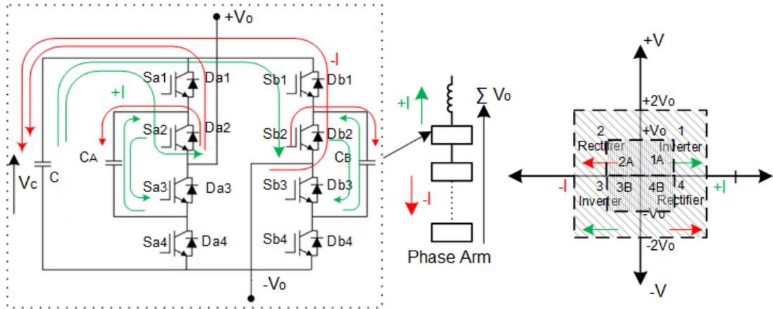
Figure 2.8:FC H-bridge Sub-module: (a) Power Circuit showing Rectifier and Inverter Mode (b) Sub-module arrangement for one phase (c) I-V four Quadrant operations
