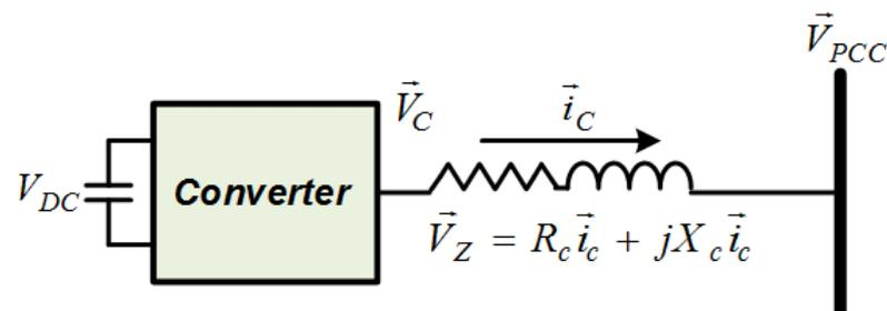
Figure 5.5: Voltage-Current relationship between Converter and PCC
