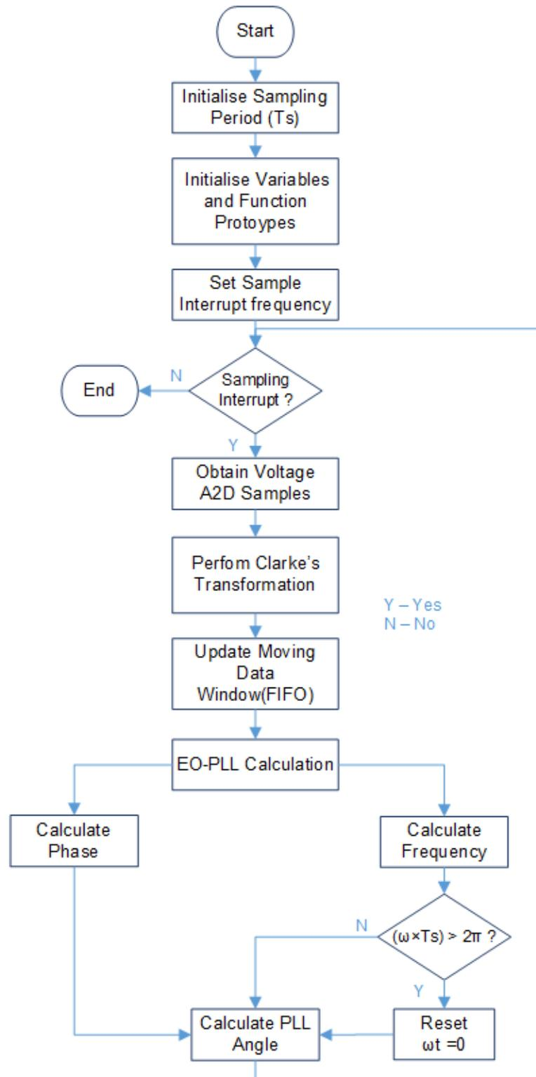
Figure 4.16: Program Flow Chart for EO-PLL Scheme
