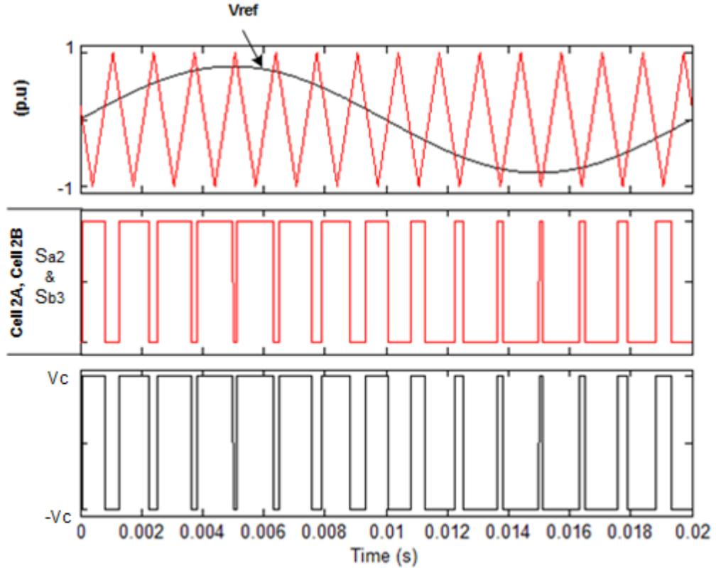
Figure 3.2: Bipolar Switching of Unit Cells
