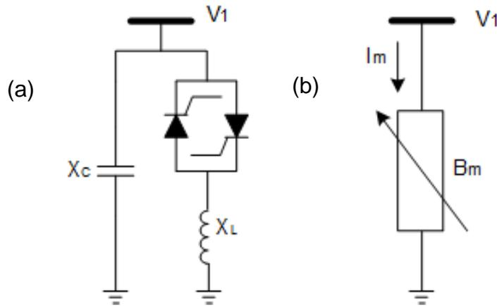
Figure 1.3: Static VAR Compensator: (a) TCR with fixed capacitor
