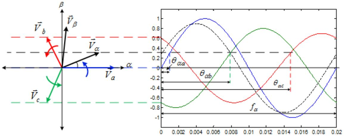
Figure 4.5: Graphical Illustration of EO-PLL Under Unbalanced Voltages
