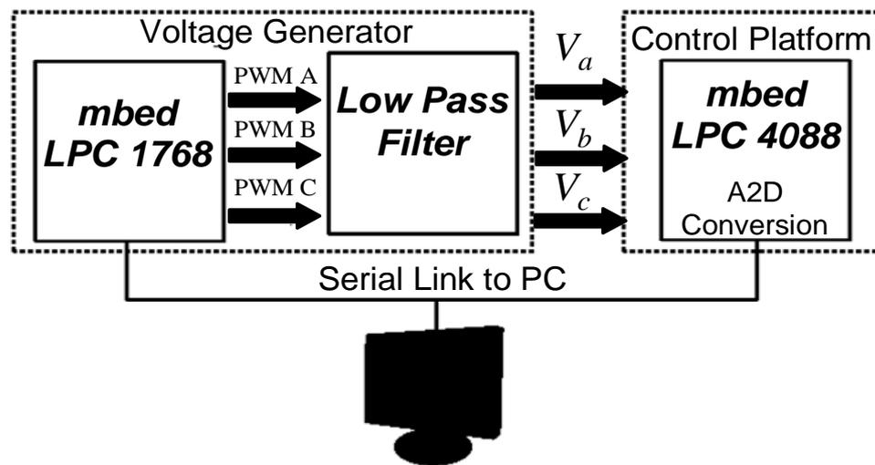
Figure 4.14: EO-PLL hardware test circuit setup
