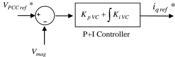
Figure 5.13: PCC Voltage Controller
