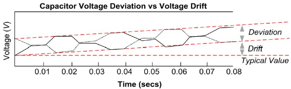
Figure 3.6: Illustration of Capacitor Voltage Deviation and Voltage Drift
