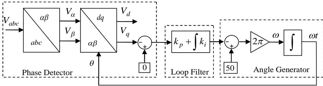
Figure 1.13: Synchronous Reference Frame PLL (SRF-PLL)
