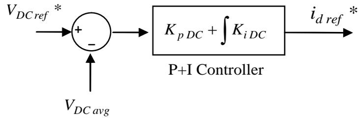
Figure 5.12: Capacitor DC Voltage Controller
