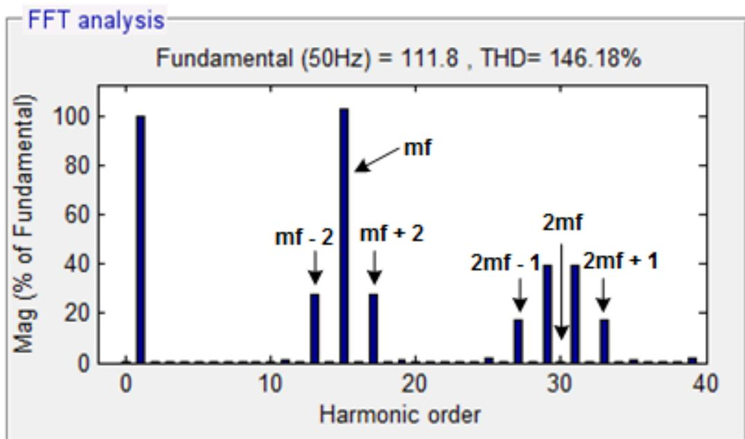
Figure 3.3: Total Harmonic Distortion (THD) for Bipolar Switching
