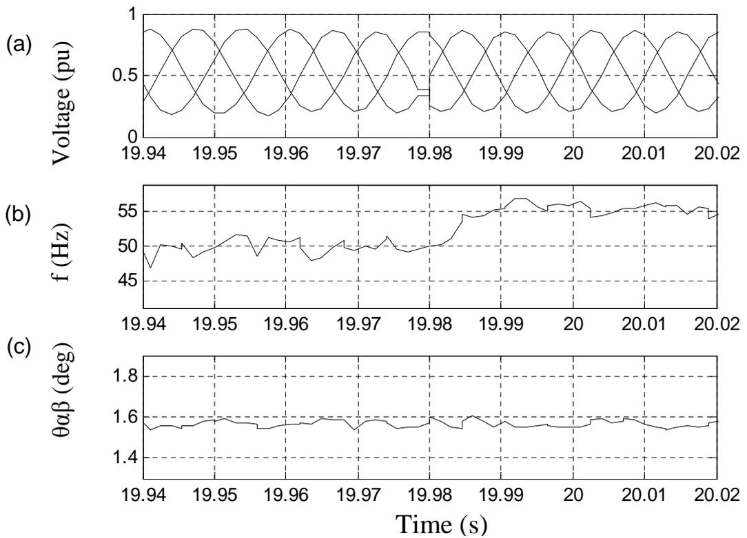
Figure 4.18: Experimental EO-PLL tracking changes in frequency from 50-55 Hz with no pre-filtering : a) Generated 3-phase voltage, b) estimated frequency, c) estimated phase
