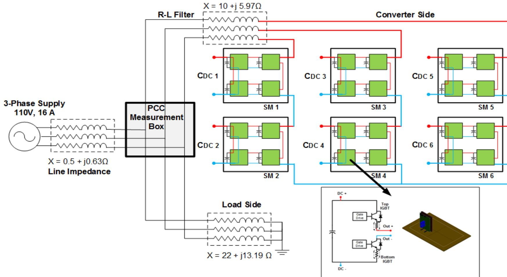
Figure 7.1: Experimental Power System Configuration
