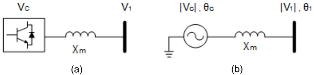
Figure 1.5: Static Synchronous Compensator: (a) Converter shunt connected to the network (b) Equivalent power circuit representation
