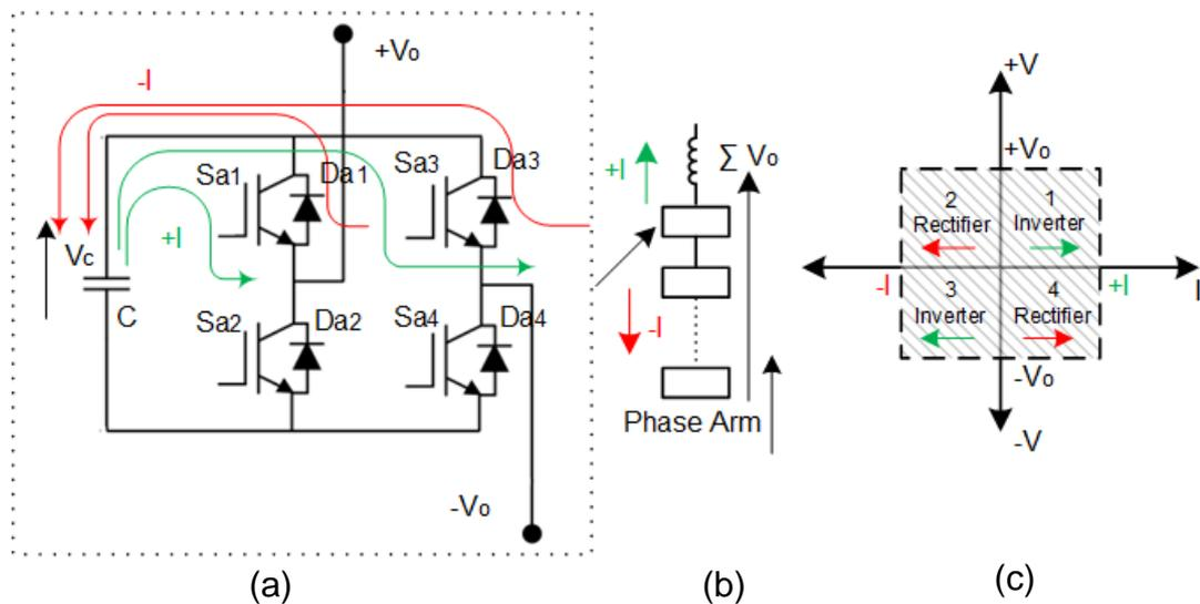
Figure 2.6:H-bridge Sub-module: (a) Power Circuit showing Rectifier and Inverter Modes (b) Sub-module arrangement for one phase (c) Four Quadrant operation modes
