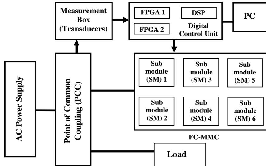
Figure 6.1: Block Diagram of FC-MMC STATCOM
