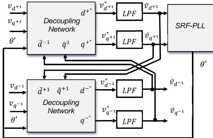
Decoupling Network + SRF-PLL (DDSRF-PLL)
