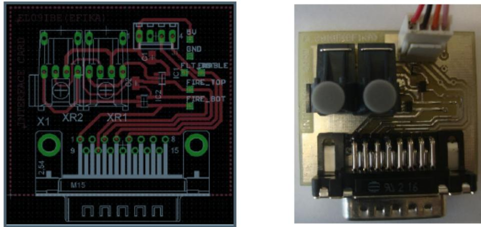
Figure 6.9: Fibre Optic Receivers PCB Design
