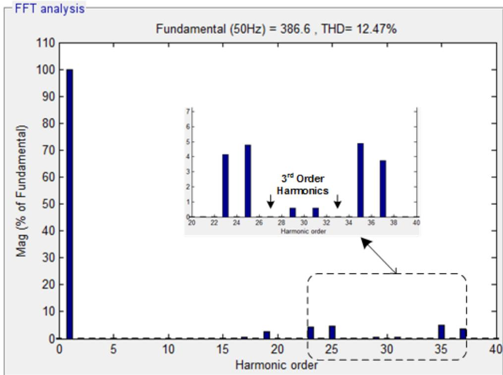
Figure 3.10: Line Voltage Spectrum & THD value for PD-PWM at  $m_f = 15$
