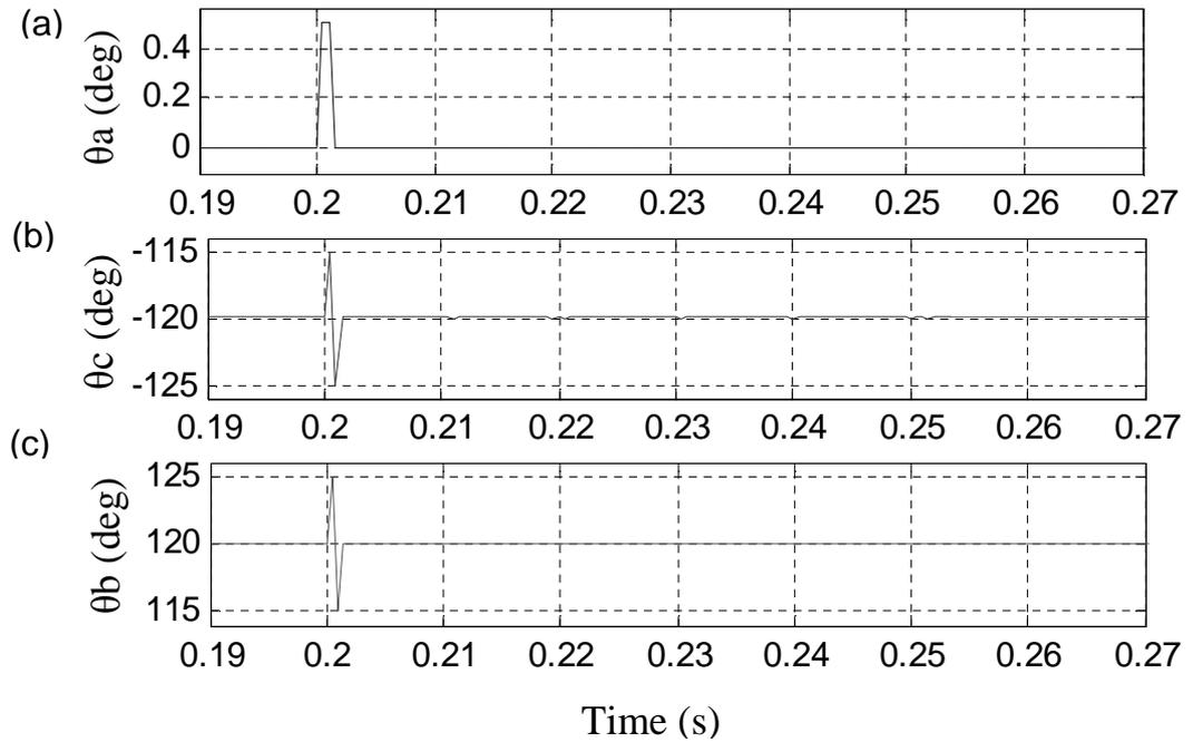
Figure 4.10: EO-PLL Estimation of Phase Angles under type B fault; (a) Phase A (degrees) (b) Phase C (degrees), (c) Phase B (degrees)
