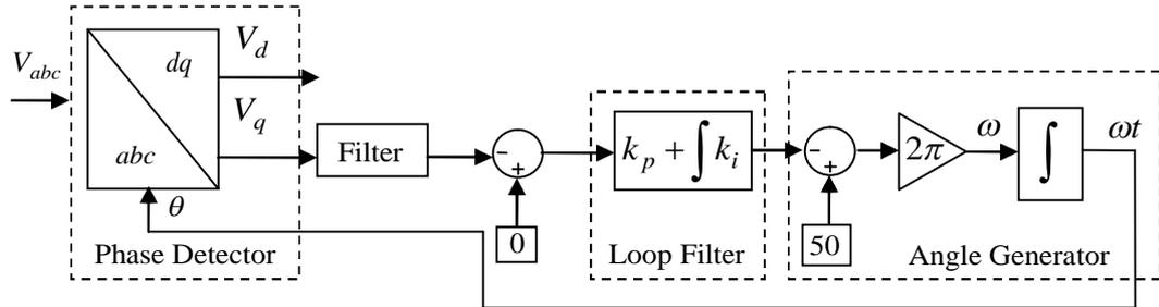
Figure 1.14: Filter +SRF-PLL
