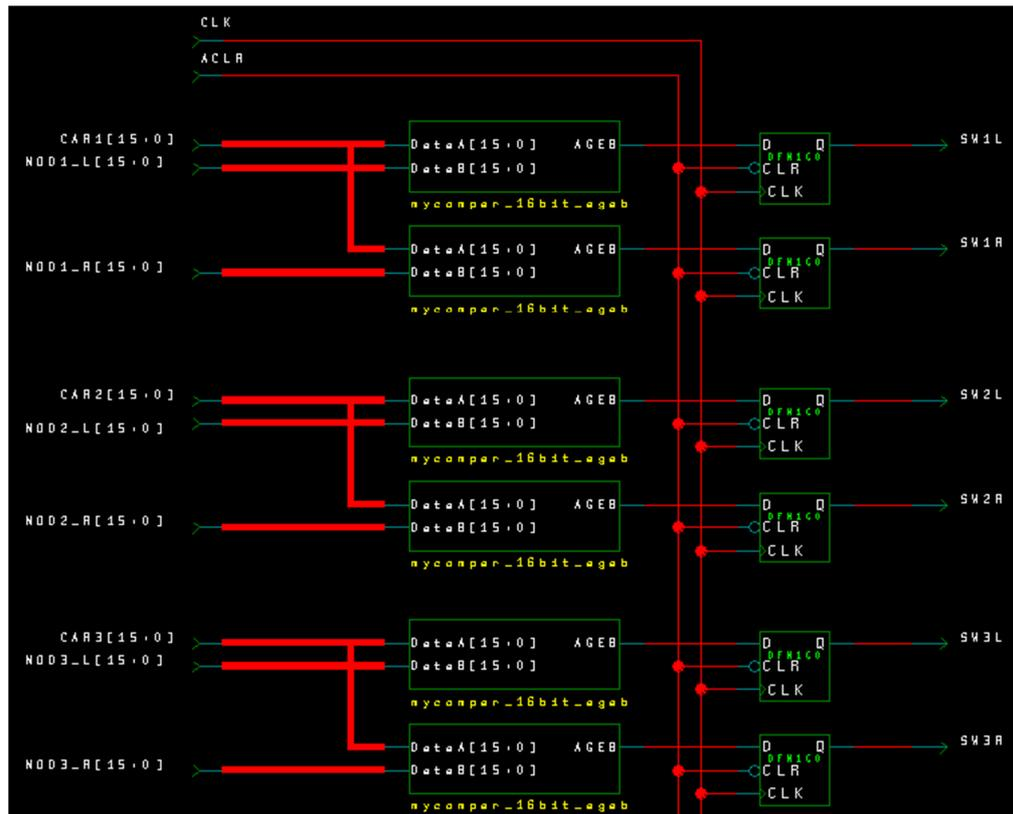
Figure 6.32: Pulse Generation unit in FPGA
