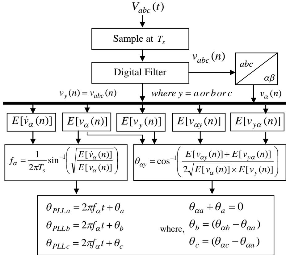
Figure 4.4: Block Diagram of EO-PLL Implementation
