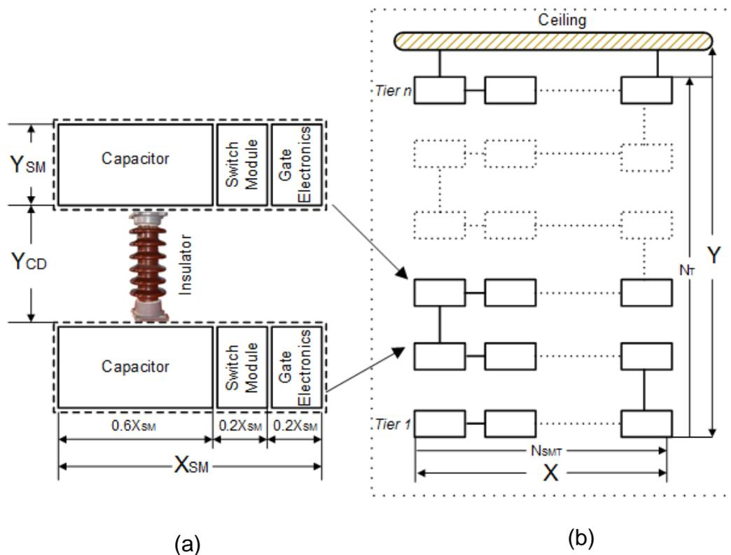
Figure 2.2: Guideline for Footprint Assessment (a) Sub-module Footprint with insulator (b) Platform Footprint with sub-modules
