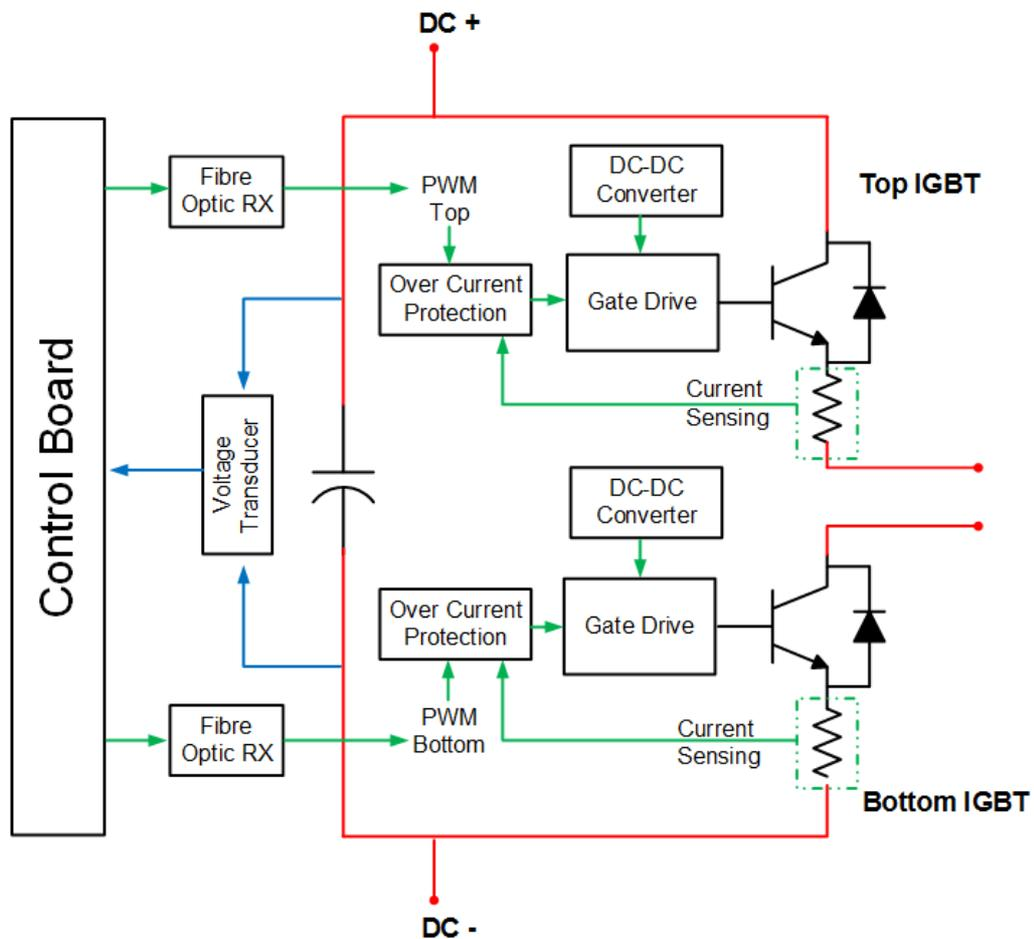
Figure 6.5: Unit Power Cell Circuit Diagram
