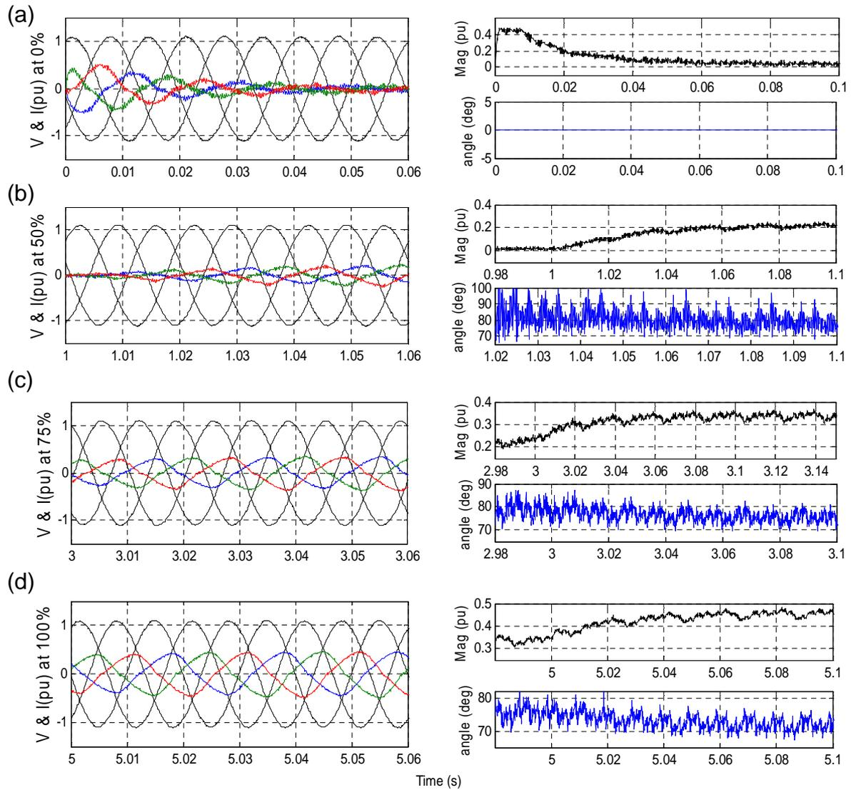
Figure 7.19: Voltage, Current and Converter Angle, (a) Zero compensation, (b) 50% compensation, (c) 75% compensation, (d) Full compensation
