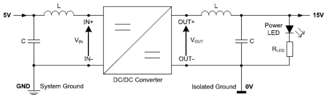
Figure 6.14: +15V Switch Mode Power Supply
