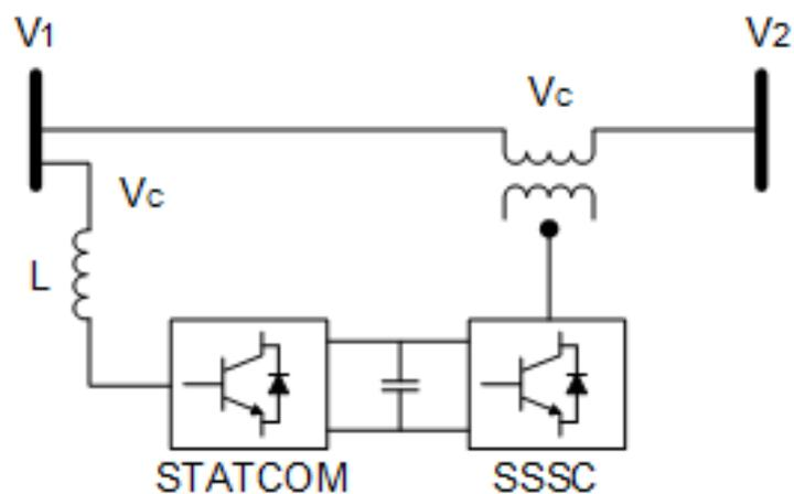
Figure 1.6: Unified Power Flow Controller
