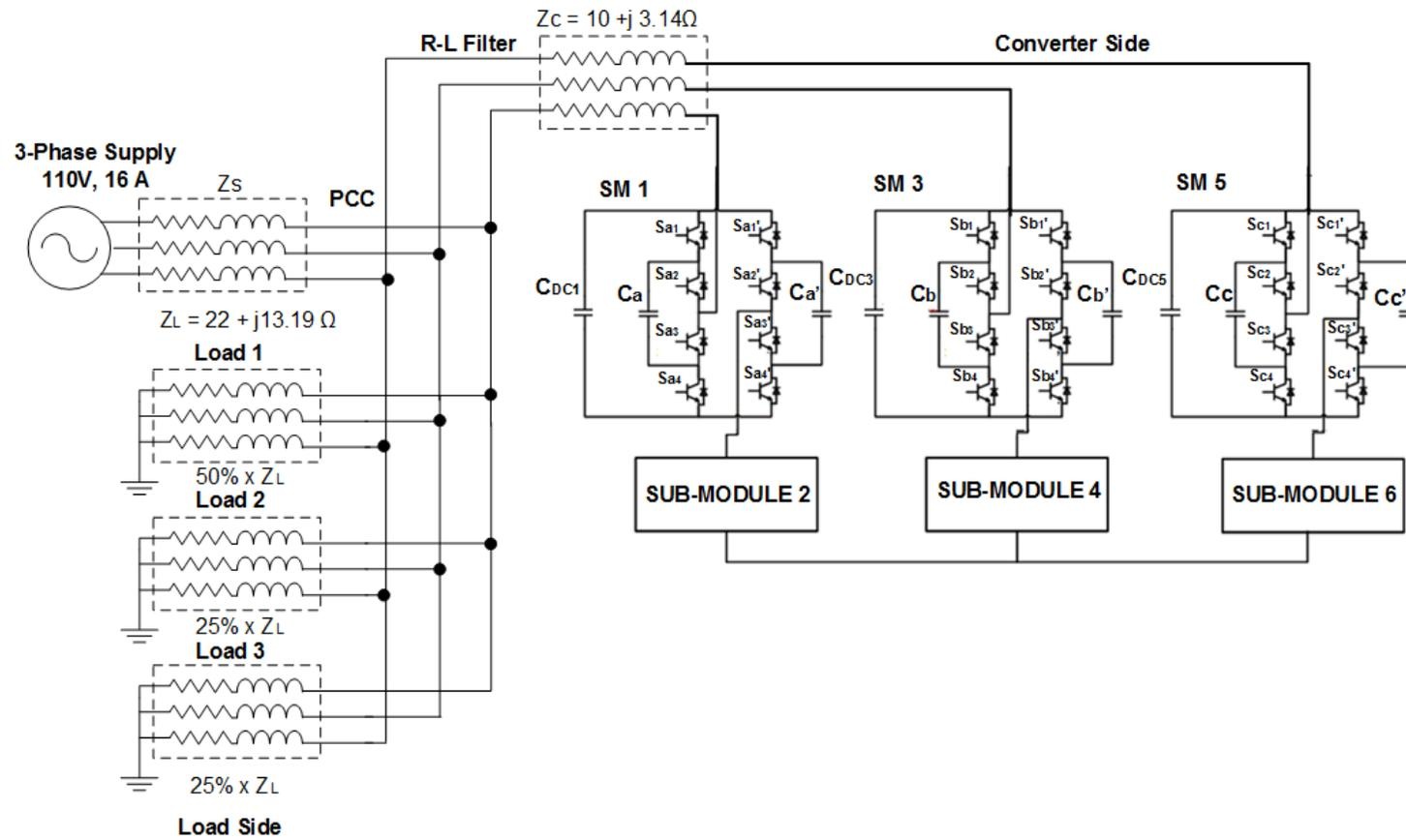
Figure 5.10: Simulation Power System Configuration
