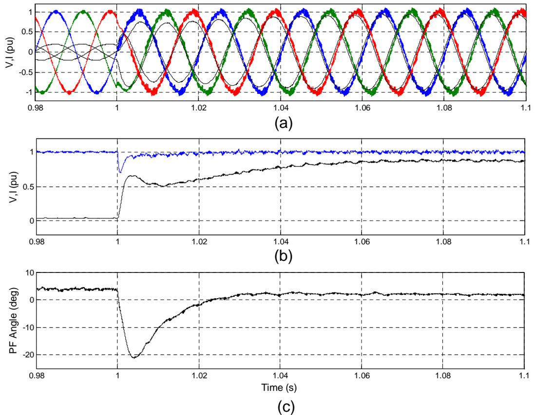
Figure 5.16: (a) Three Phase Voltage and Current, (b) Voltage Magnitude and Current Magnitude, (c) Power Factor Angle
