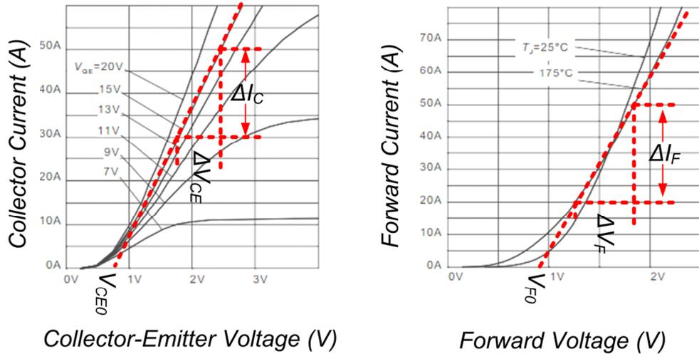
Figure 2.3: Characteristics of the IGBT Collector-Emitter Voltage to current and Diode Forward Voltage to current
