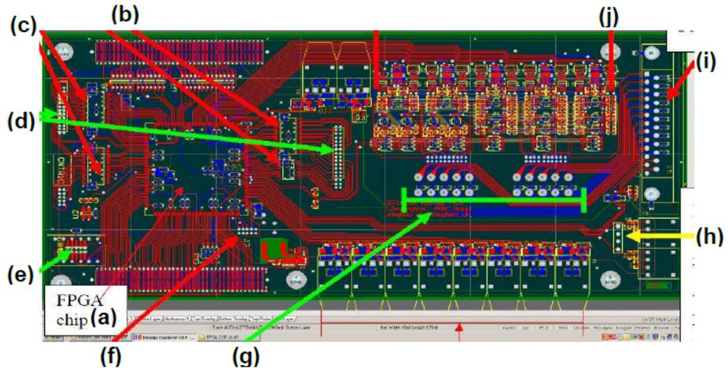
Figure 6.26: Actel Pro Asic 3 FPGA Layout
