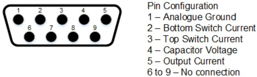
Figure 6.23: Pin layout Feedback Signals
