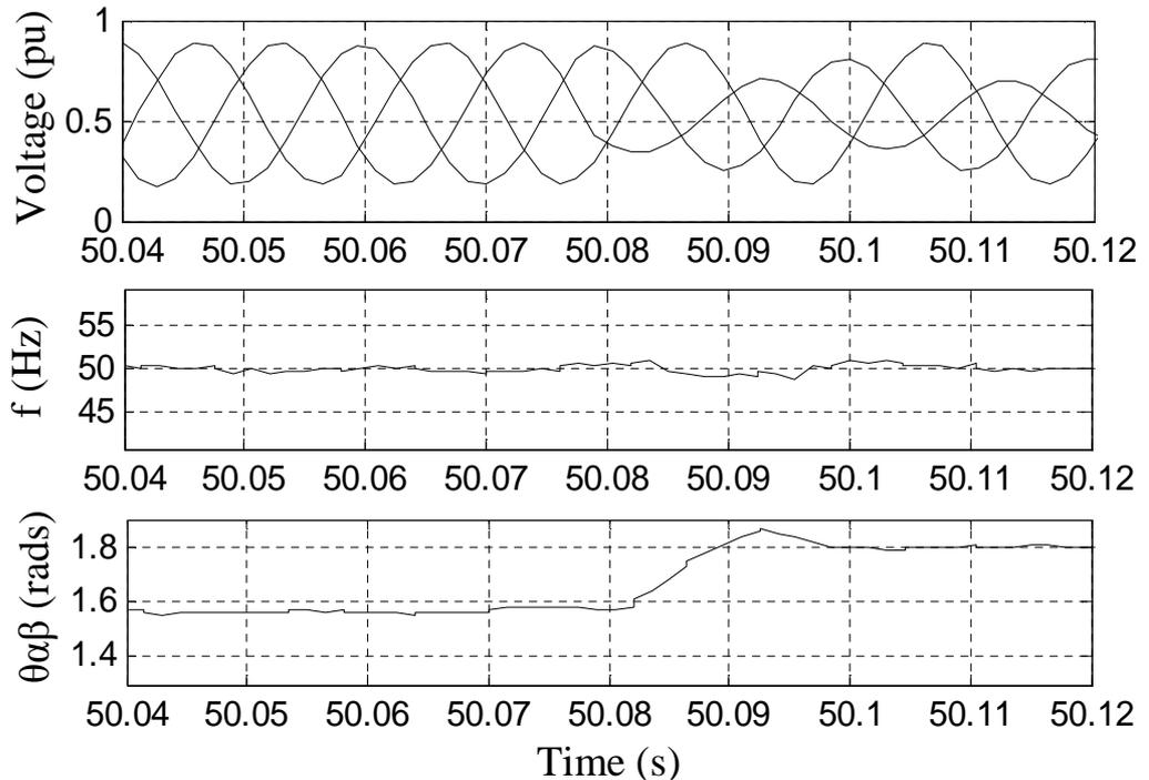
Figure 4.19: Detected result for 50% and 80% reduction in phase-B and phase-C respectively amplitude: a) Generated 3-phase voltage, b) estimated frequency, c) estimated phase
