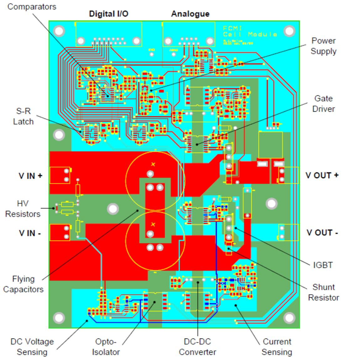
Figure 6.6: Unit Power Cell Card PCB Design
