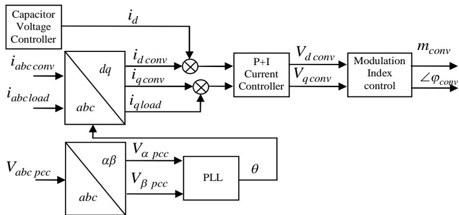
Figure 7.3: Block Diagram of the Control System
