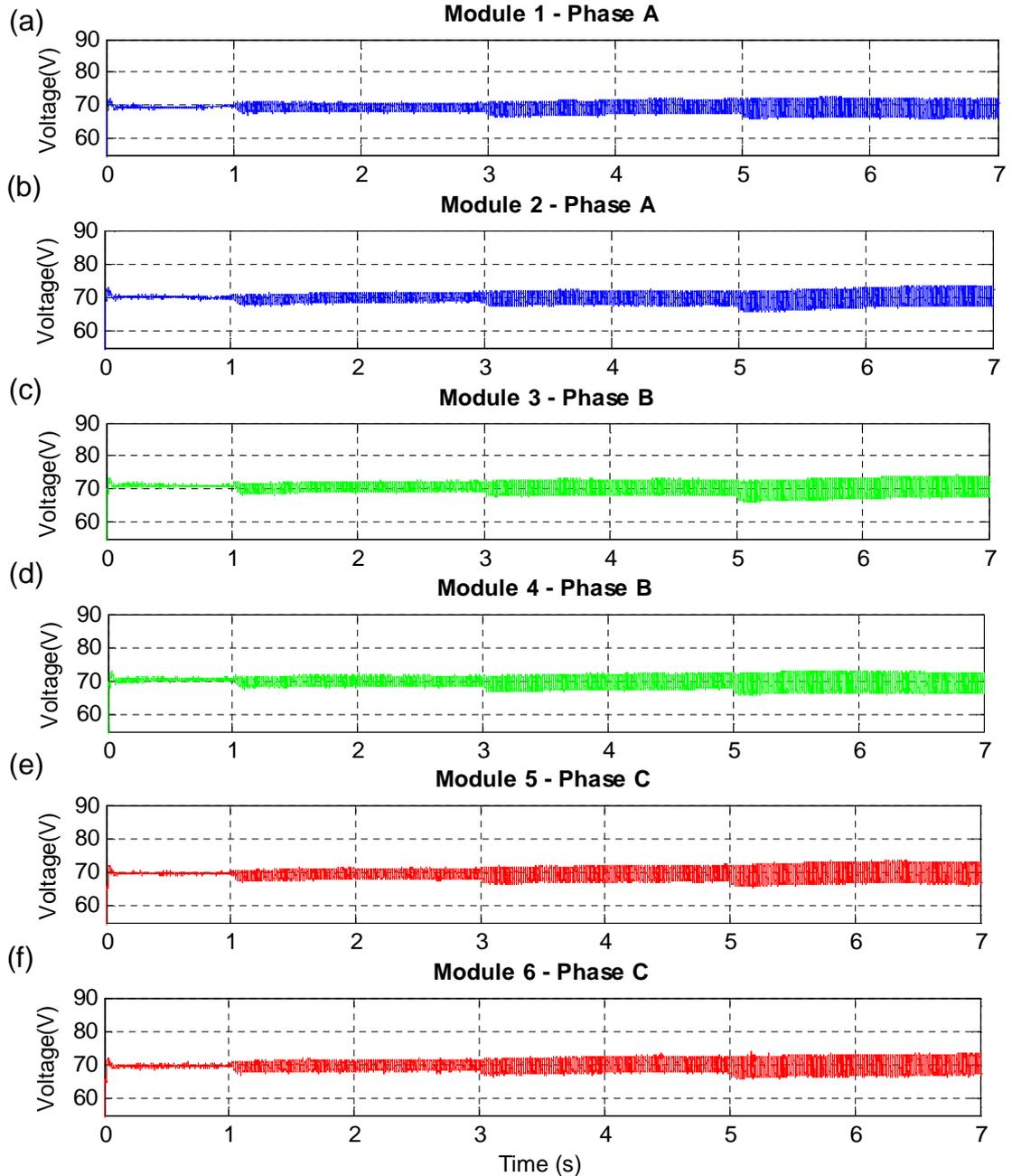
Figure 7.21: Outer Capacitor Waveforms
