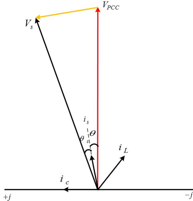
Figure 5.3: Phasor Diagram showing  $|V_S| = |V_{PCC}|$  operation
