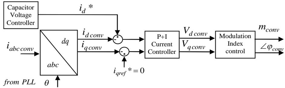
Figure 7.6: Block Diagram for Pre-Charge Control
