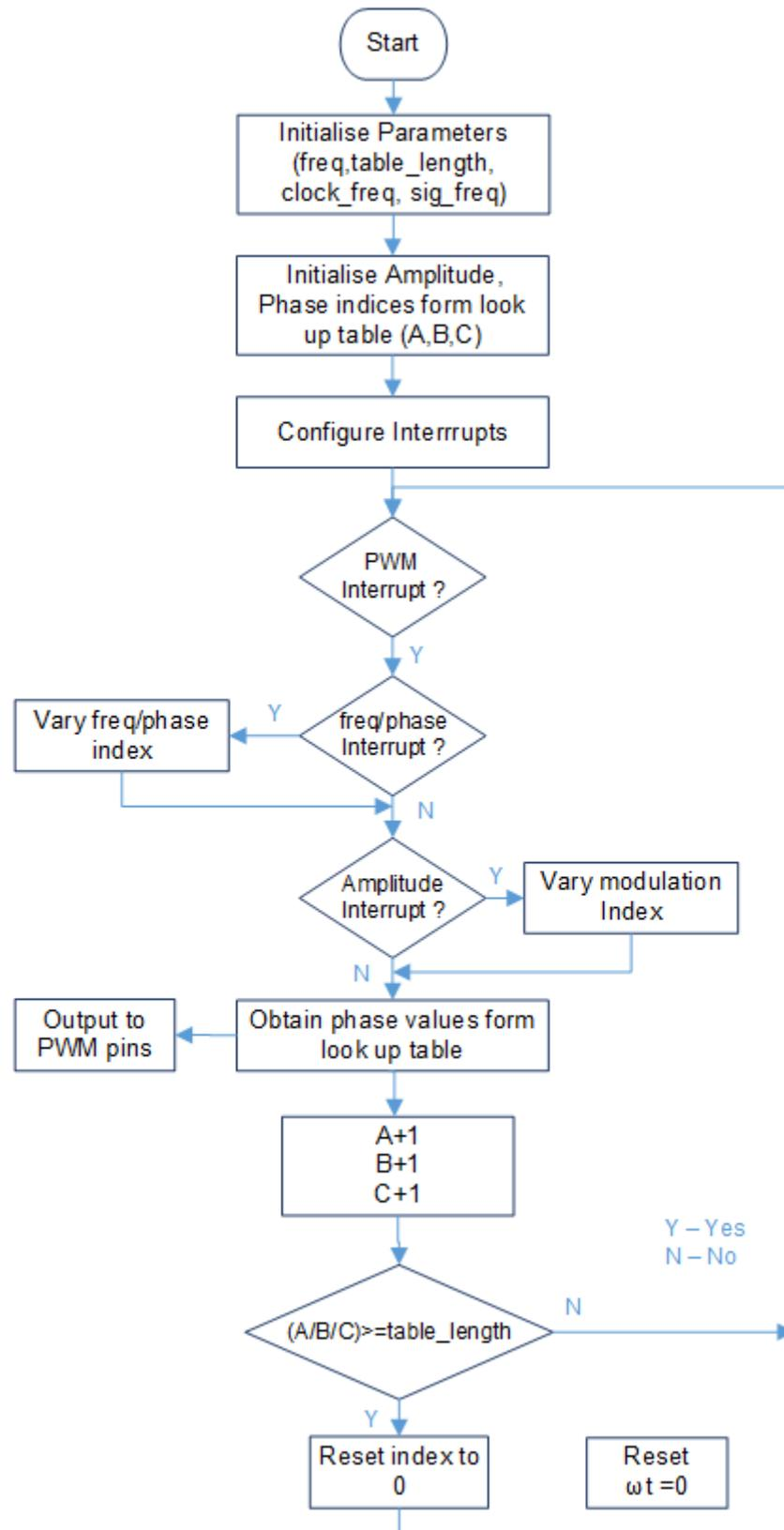
Figure 4.15: Voltage Generation Program Flow Chart
