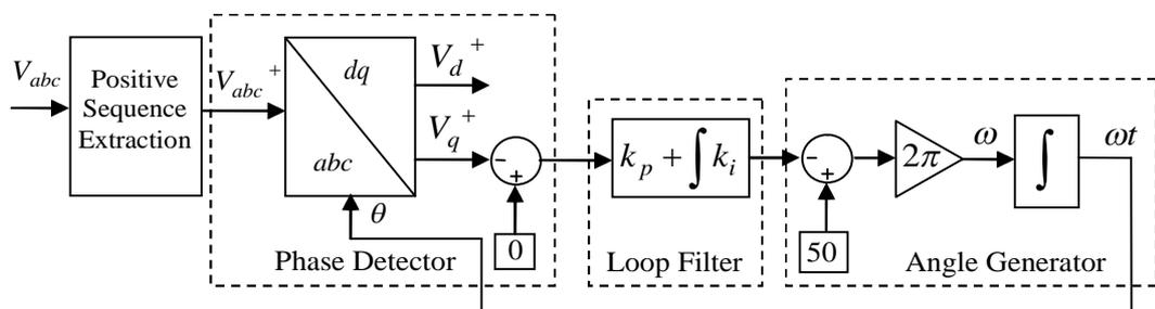
Figure 1.15: Positive Sequence Extraction + (SRF-PLL)
