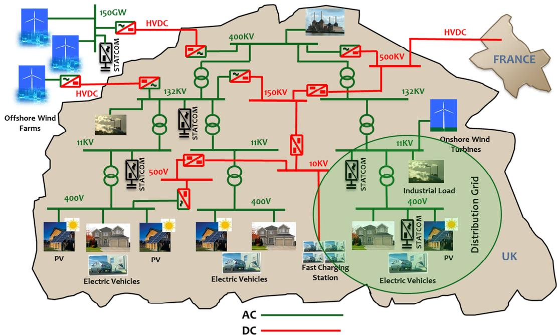
Figure 1.1: Future Transmission and Distribution Grid System
