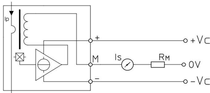
Figure 6.18: Current Transducer Circuit
