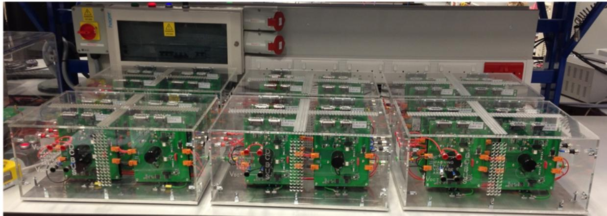
Figure 6.4: (a) Single Phase 5-level MMC-FC, (b) Three-Phase 5-level MMC-FC
