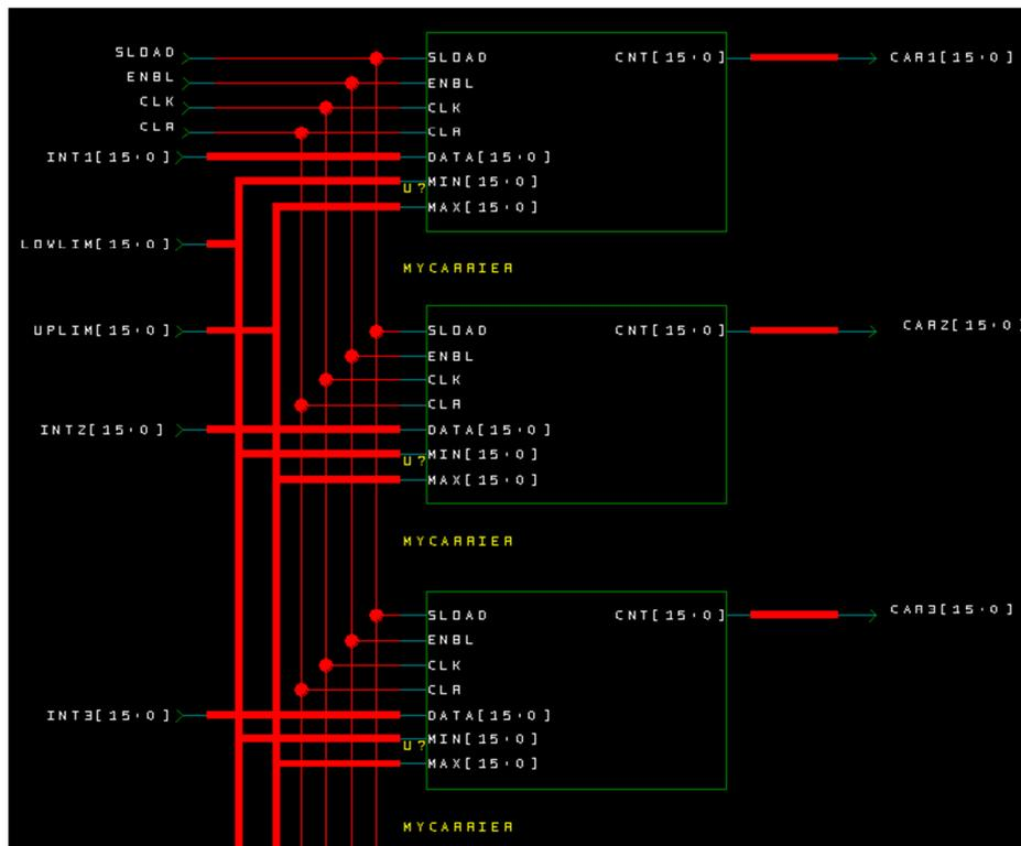
Figure 6.31: Carrier Generation Unit in FPGA
