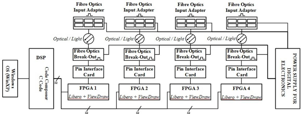
Figure 6.25: Block Diagram Software Control Unit
