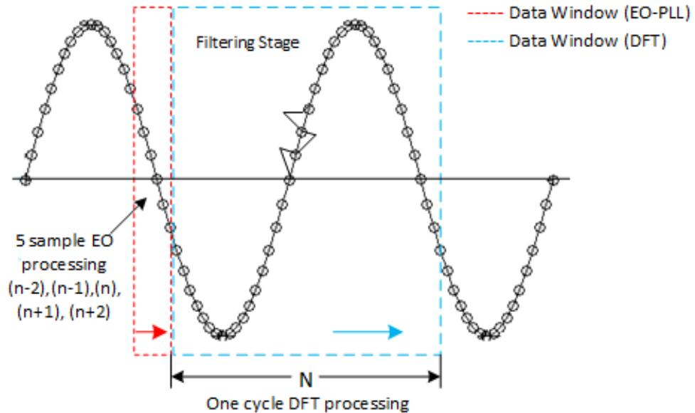
Figure 4.6: Data processing stages with a DFT as a filter
