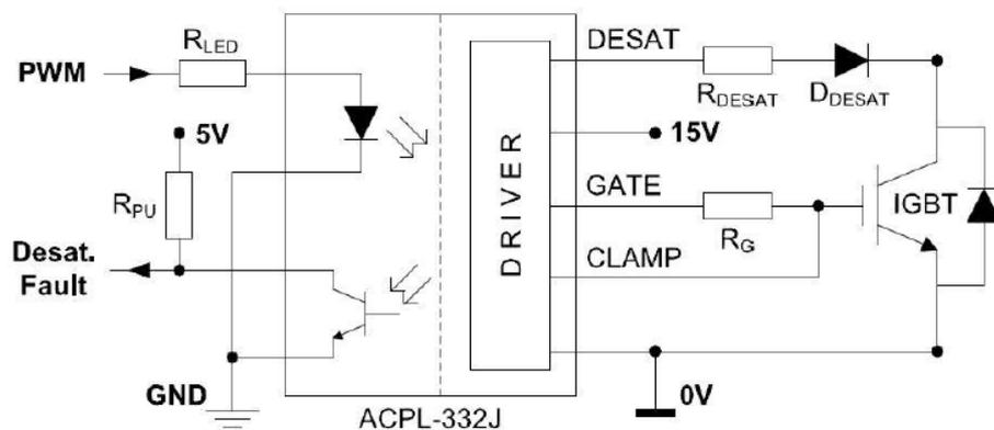
Figure 6.8: Gate Drive Circuit
