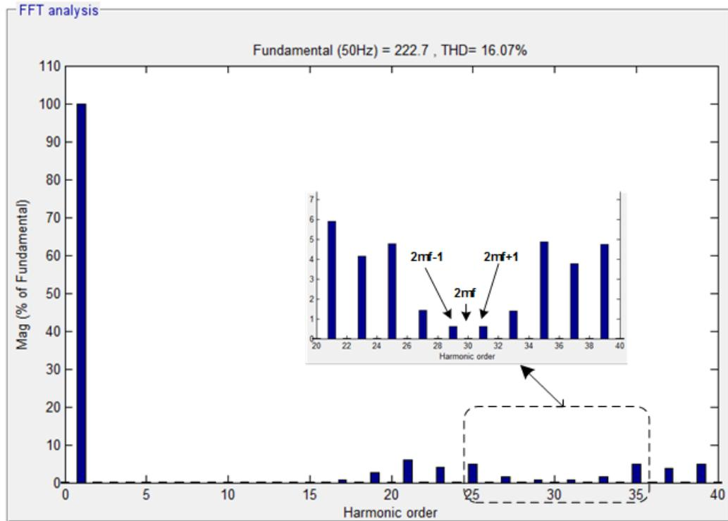
Figure 3.9: Phase voltage spectrum & THD value for PD-PWM at  $m_f = 15$
