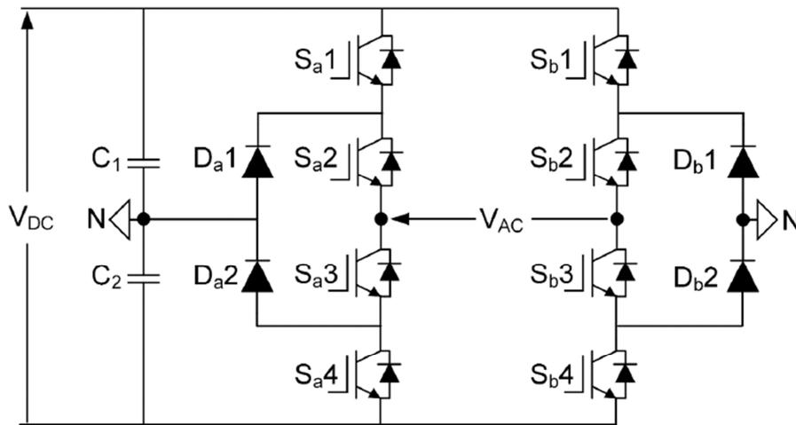
Figure 1.7: H-bridge Configuration of a Neutral Point Clamped Converter
