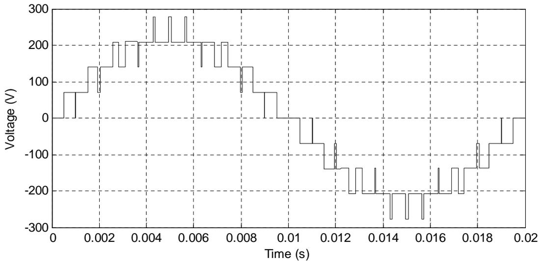
Figure 3.8: Phase Voltage of the FC-MMC under PD-PWM
