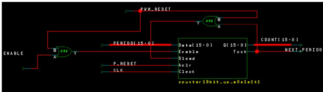
Figure 6.29: 16-bit Interrupt Counter
