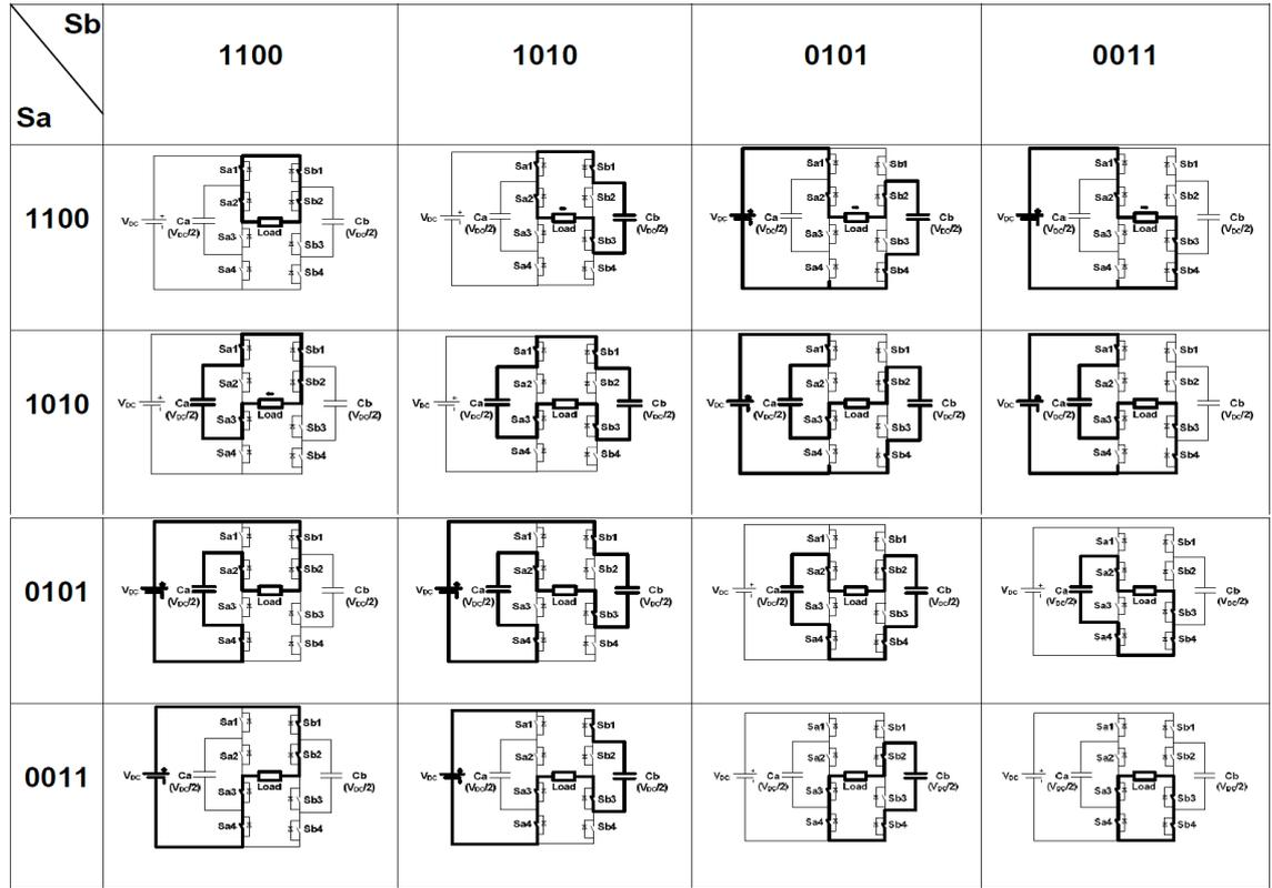
Current Paths for five-level flying capacitor multilevel inverter switching states
