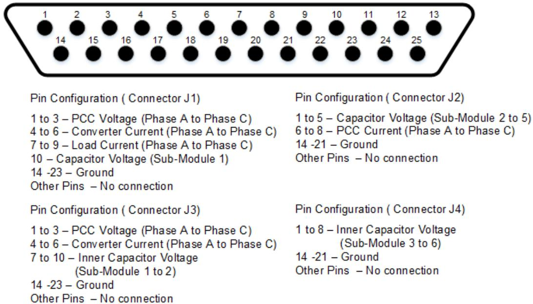
Figure 6.24: Pin Layout for Breakout Connectors
