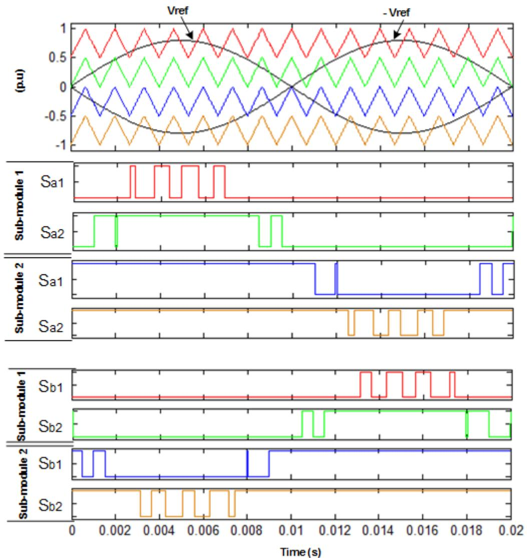
Figure 3.7: Phase Disposition PWM applied to FC-MMC at  $m_f = 15$
