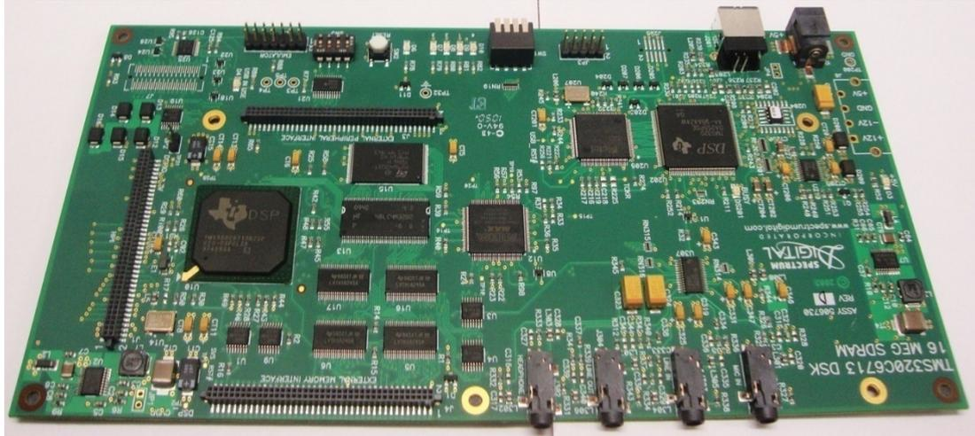
Figure 6.33: Texas Instrument TMS320C6713 DSP
