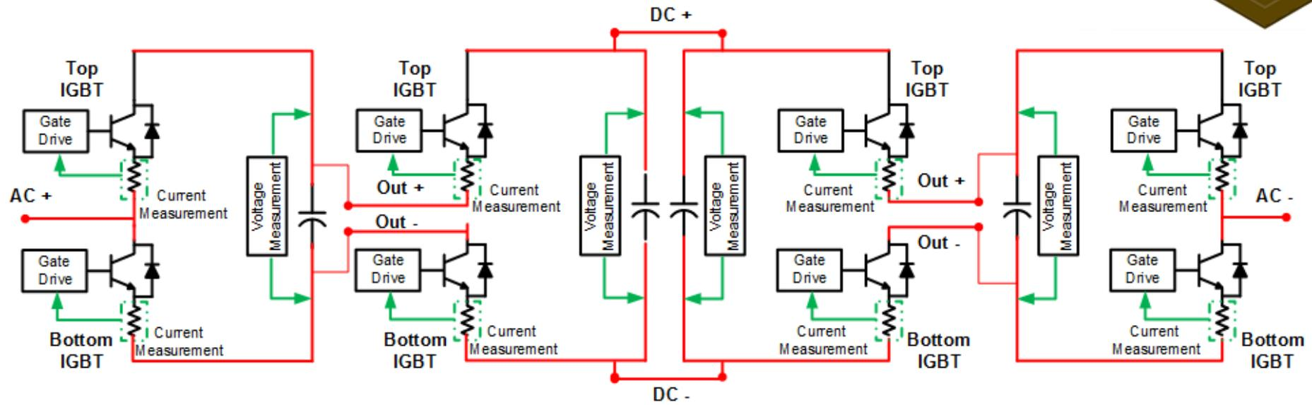
Figure 6.3: 5-level Full bridge Flying Capacitor
