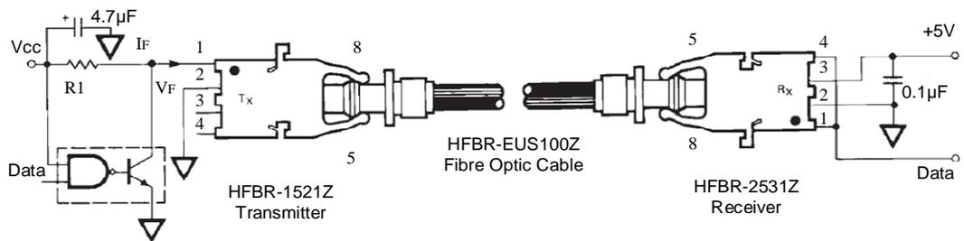
Figure 6.10: Fibre Optic Transmitter and Receiver Circuit Diagram
