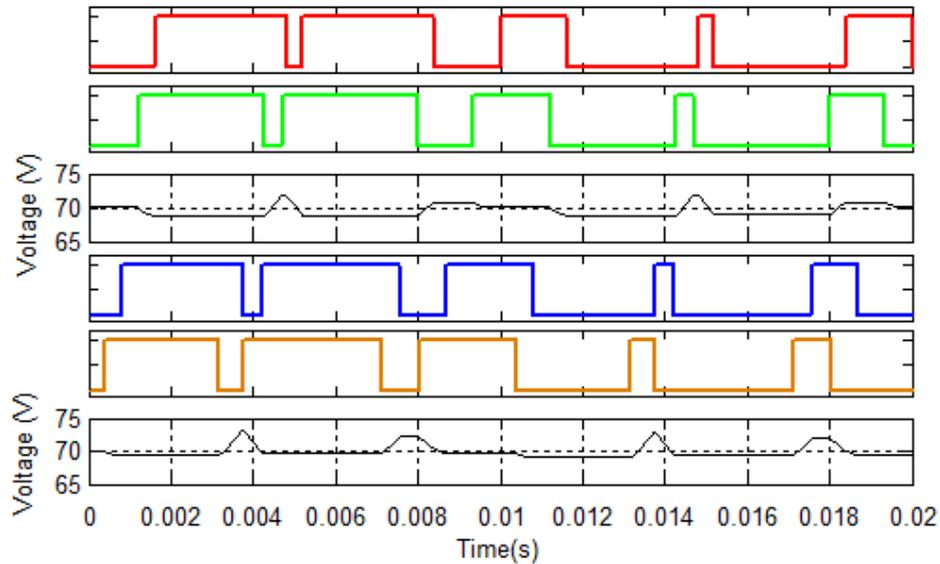
Figure 3.16: PS-PWM Switching actions in a fundamental cycle
