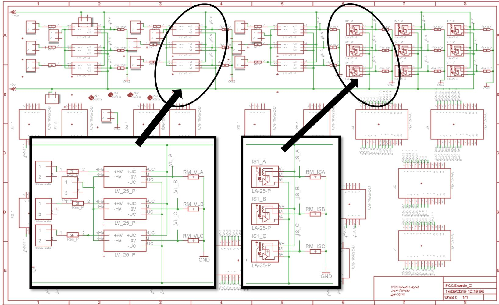
Figure 6.21: Schematic for PCC Measurement Box
