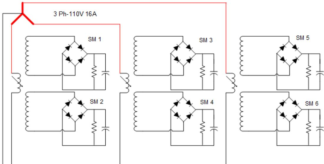
Figure 6.15: Isolated DC Power Supply Circuit
