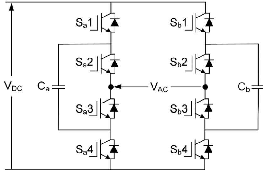
Figure 1.8: H-bridge configuration of a five-level Flying Capacitor Multilevel Inverter
