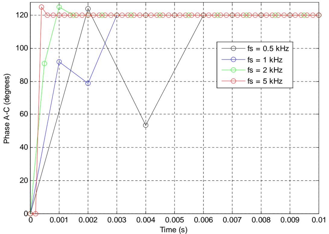
Figure 4.3: Phase angle estimation of a voltage signal at different sampling frequencies
