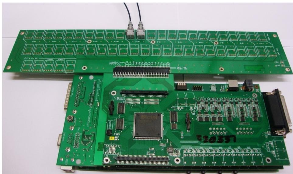
Figure 6.27: FPGA with Fibre Optic Break Out Boards
