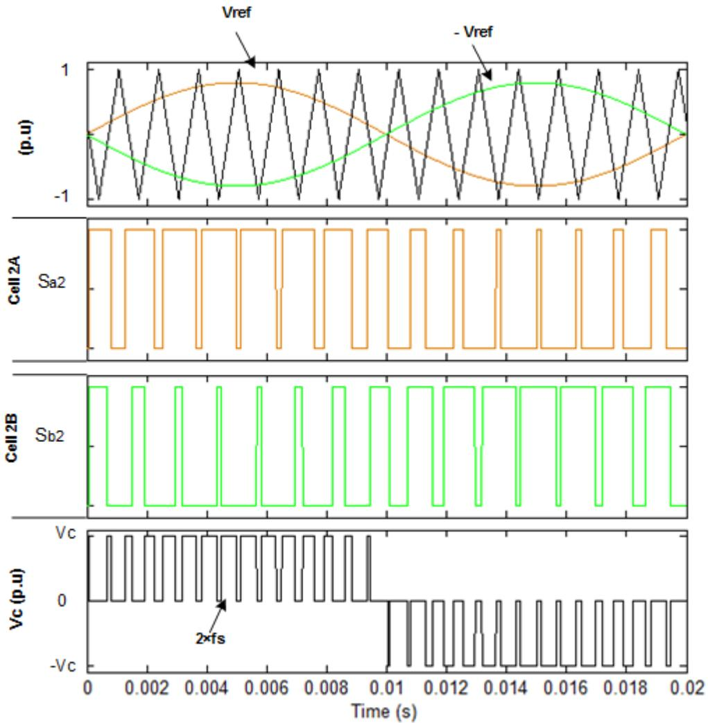
Figure 3.4: Unipolar Switching of Unit Cells
