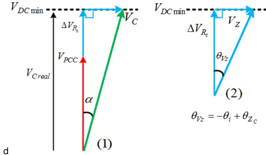
Figure 5.7: Simplified Phasor Diagram between Converter and PCC voltages
