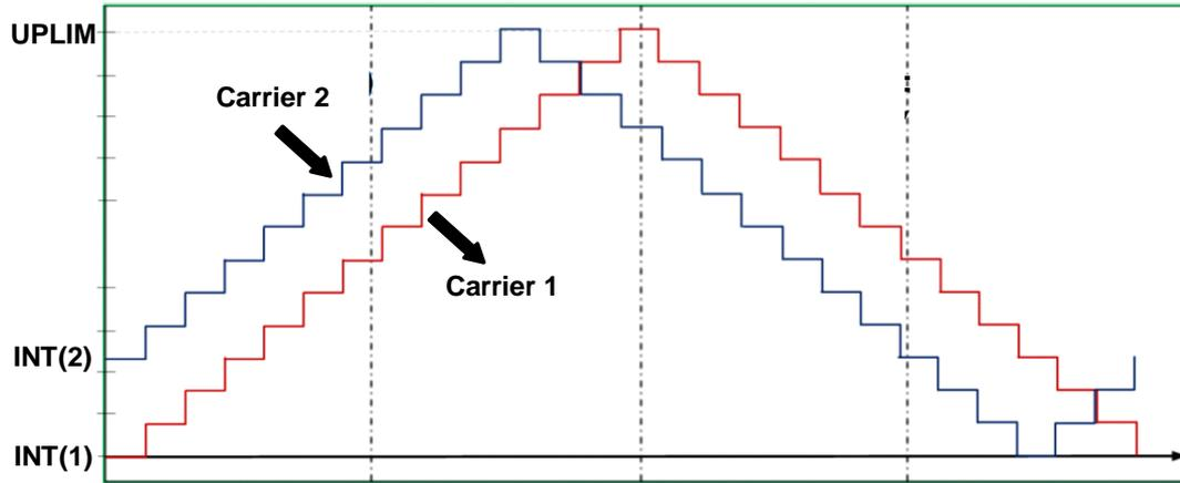
Figure 6.30: Triangular Carrier Generation
