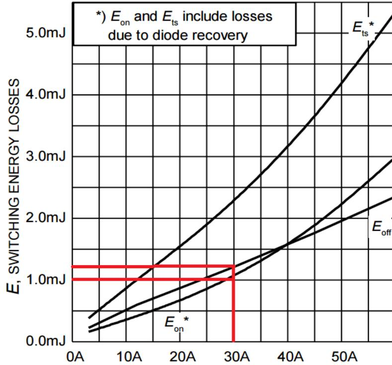
Figure 2.4: Characteristics of the IGBT current and switching energy losses [144].
