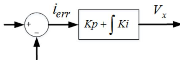
Figure 7.5: Block Diagram P+I Controller
