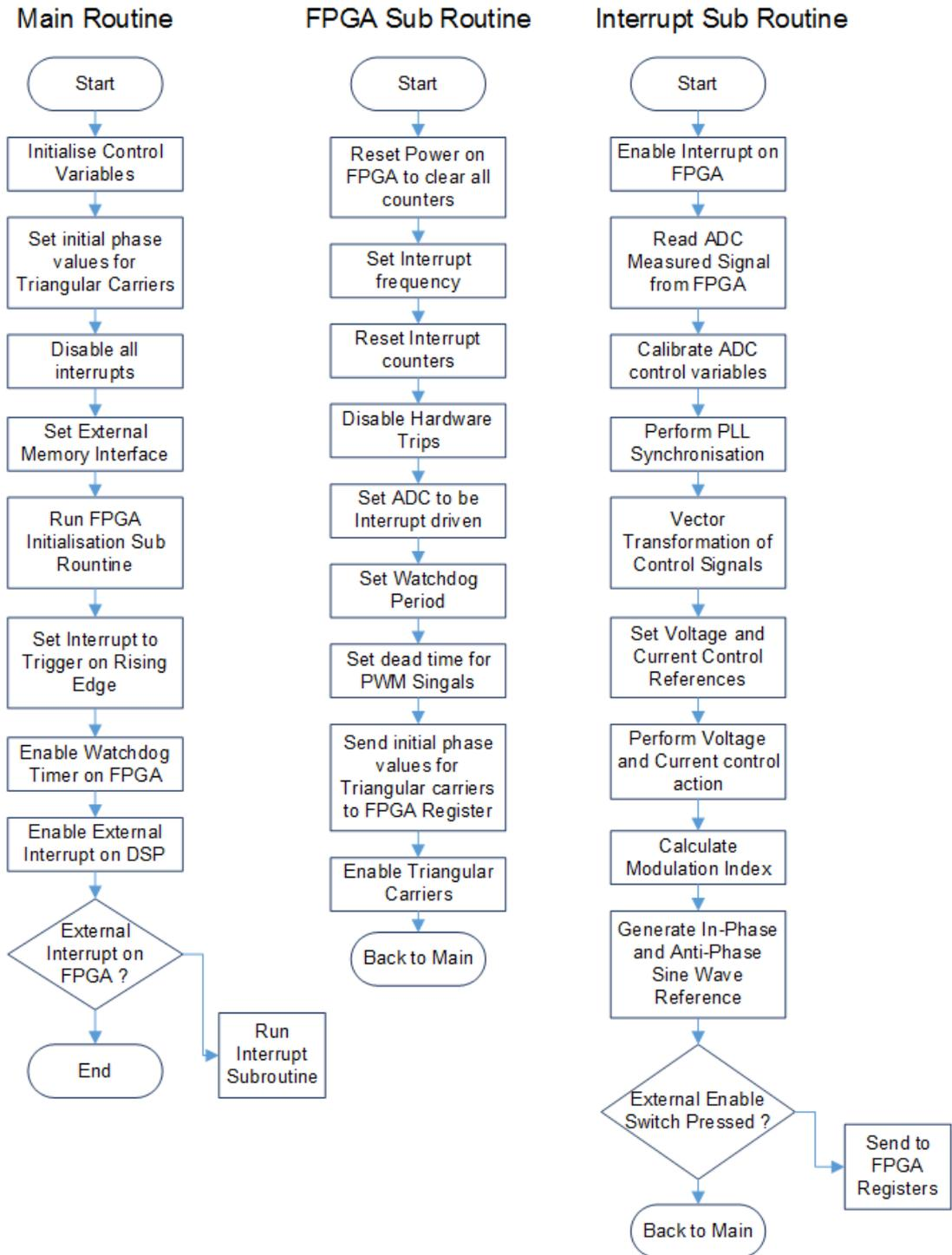
Figure 6.34: Program Flow Chart for Main Routine and Sub Routine
