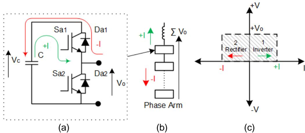
Figure 2.5: Half-bridge Sub-module: (a) Power Circuit showing Rectifier and Inverter Mode (b) Sub-module arrangement for one phase (c) Two Quadrant operation modes
