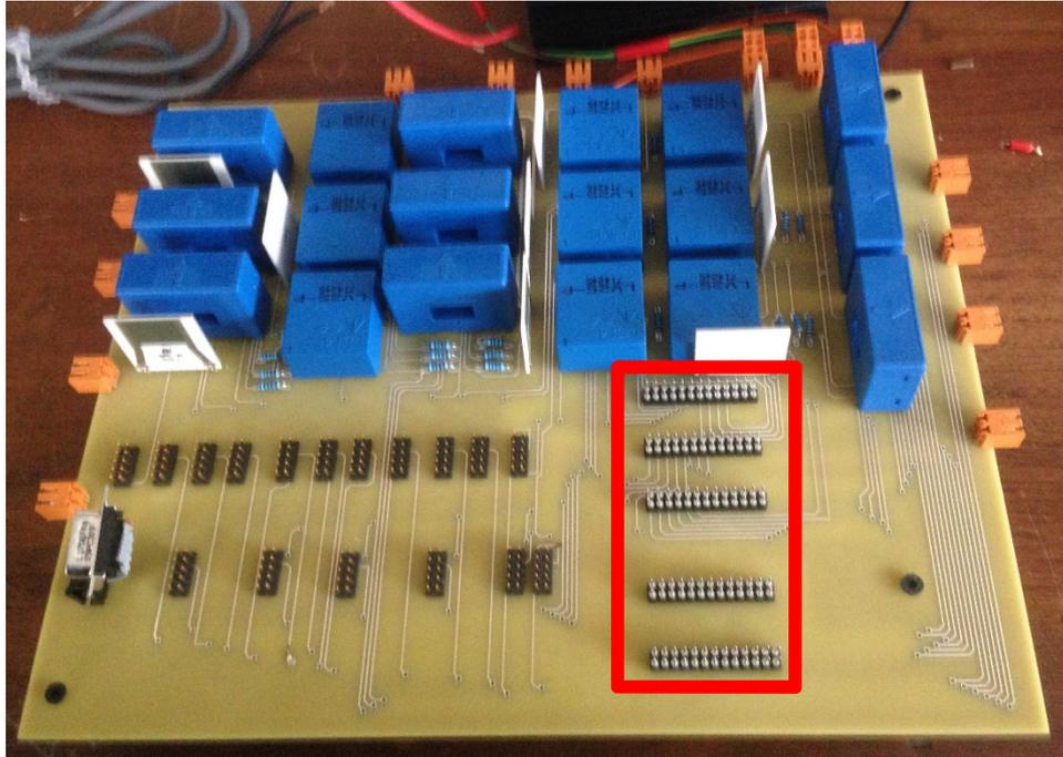
Figure 6.19: Populated PCB of PCC Measurement Box
