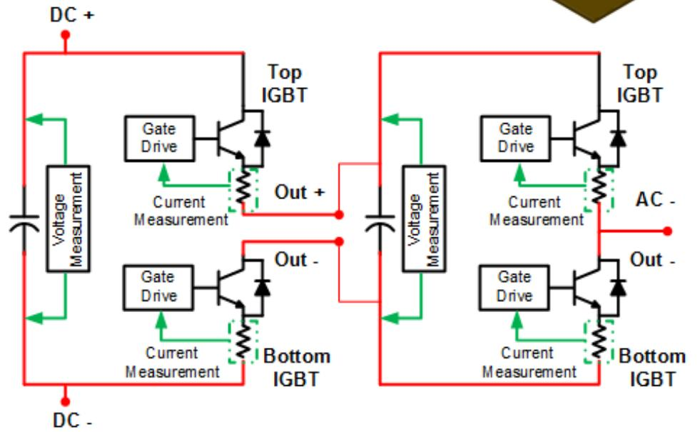
Figure 6.2: (a) Unit Power Cell (Half-bridge), (b) 5-level Half-bridge Flying Capacitor
