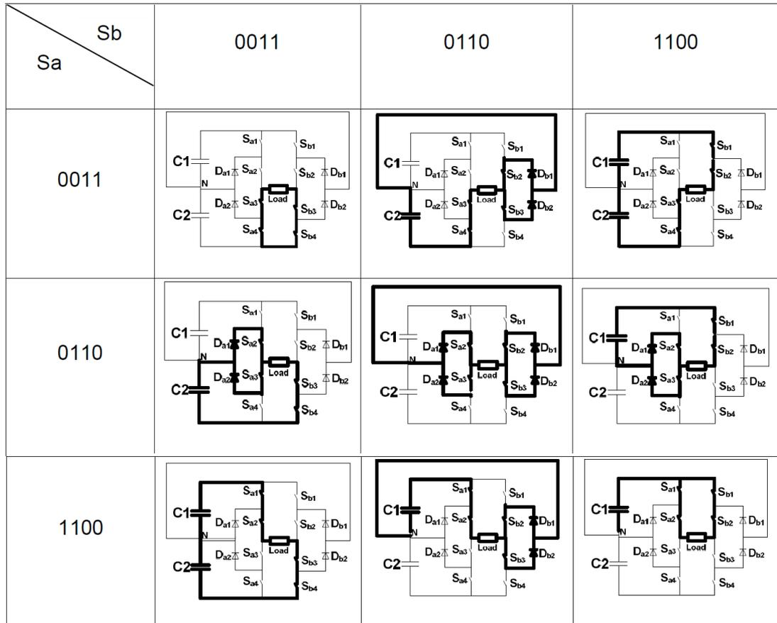
Current Paths for three-level neutral point clamped inverter switching states
