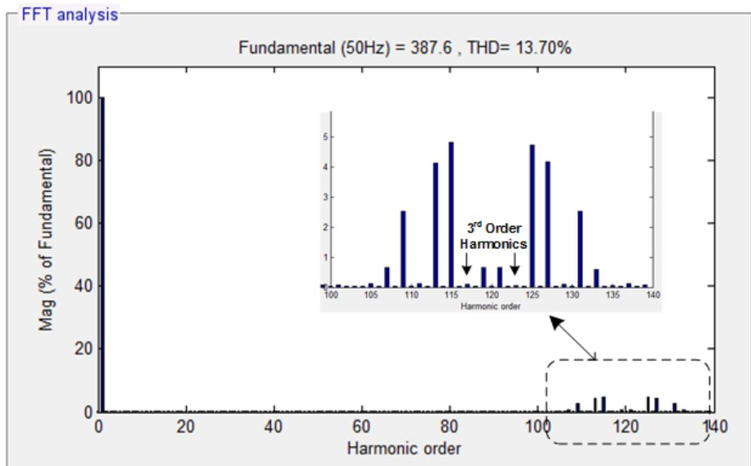
Figure 3.15: Line Voltage Spectrum & THD for PS-PWM at  $m_f = 15$
