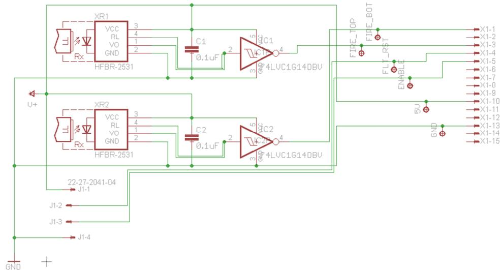
Figure 6.11: Schematic for Fibre Optic Transmitter and Receiver
