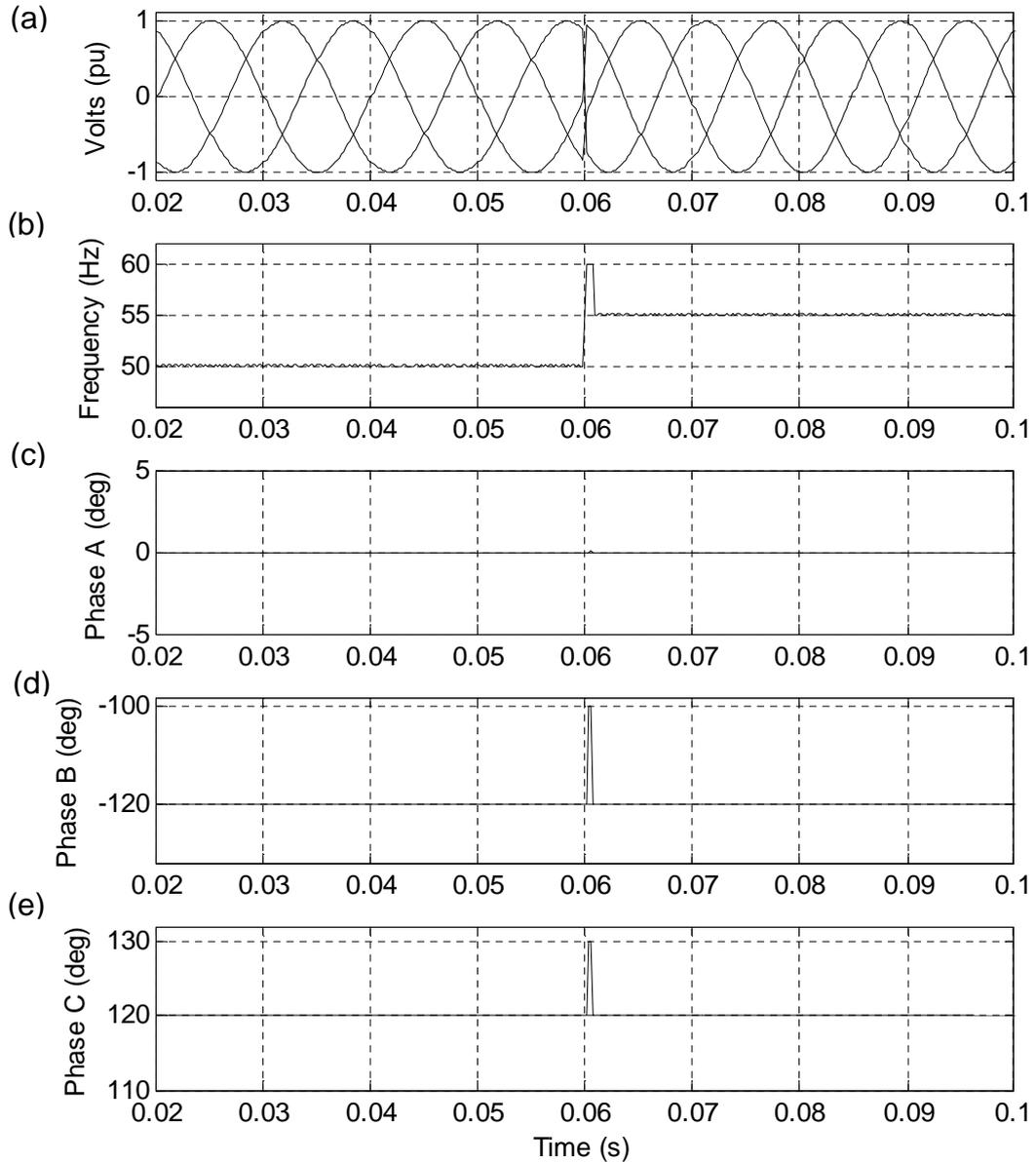
Figure 4.7: EO-PLL Under Balanced Voltage Conditions
