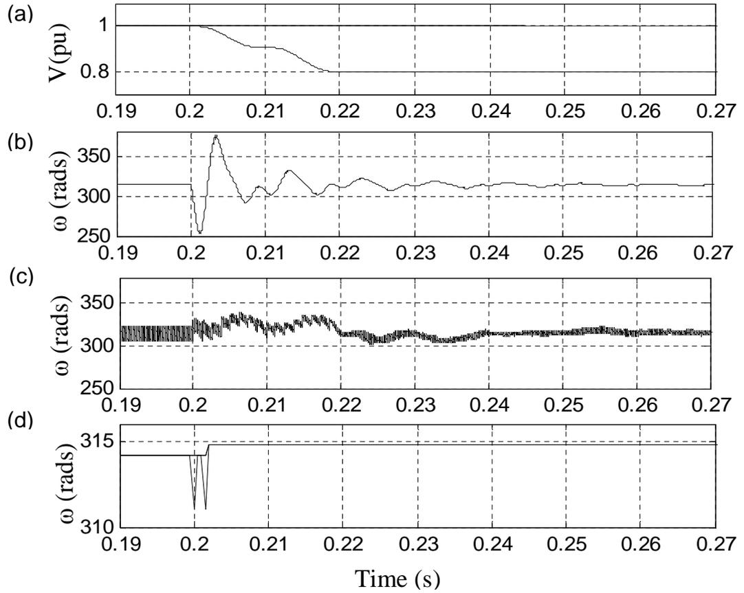
Figure 4.9: Comparison of response times for frequency tracking under type B fault (a) Peak Voltage (pu) (b) DDSRF-PLL, (c) CDSC-PLL, (d) EO-PLL
