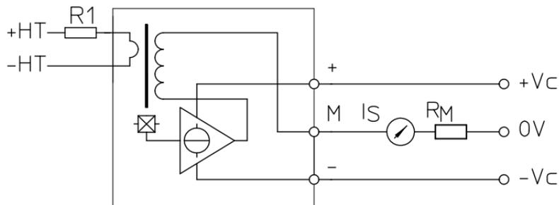
Figure 6.17: Voltage Transducer Circuit
