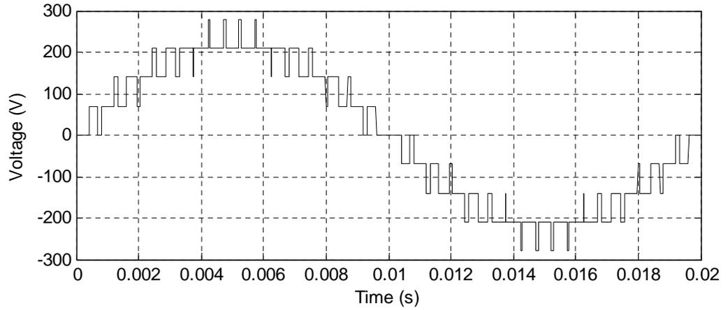
Figure 3.13:Phase Voltage of the FC-MMC under PS-PWM
