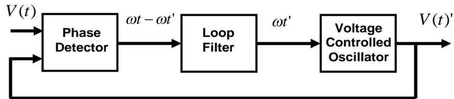
Figure 1.12: Basic structure of a closed loop synchronisation technique
