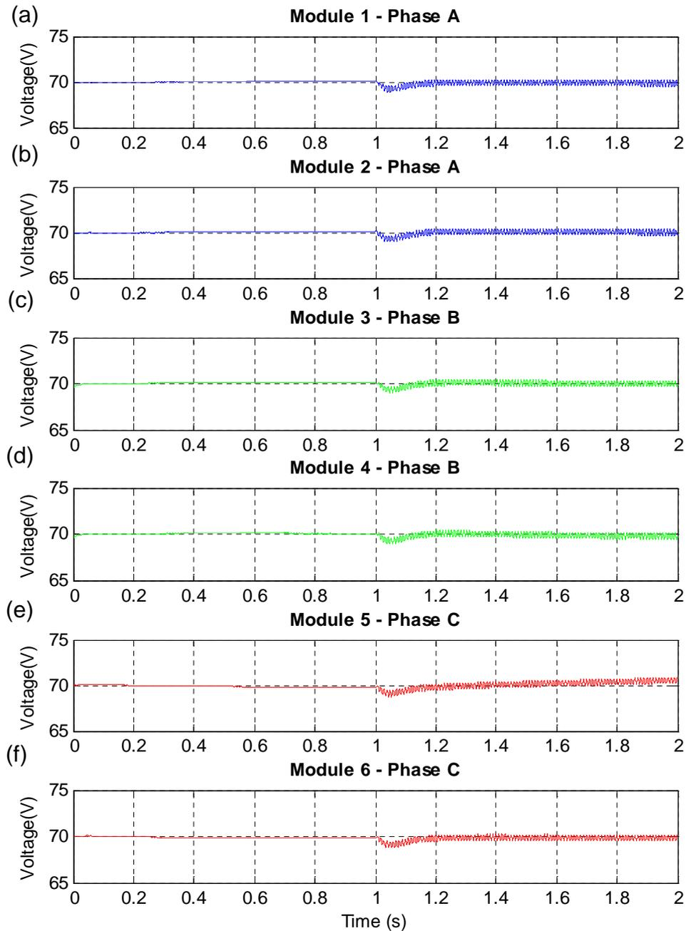
Figure 5.18: Outer Capacitor Waveforms
