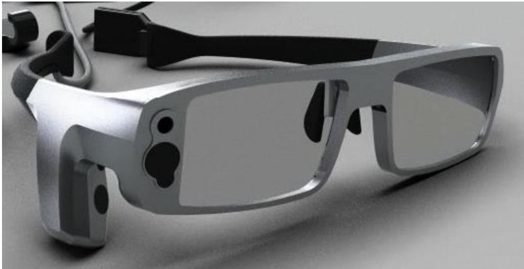
Figure 7.1. The Tobii 1.0 eye-tracking glasses that were used for data collection in this thesis.
