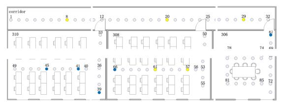
Fig. 2-3-3 Experiment environment, distribution of the access points and new AP layout in [48]
