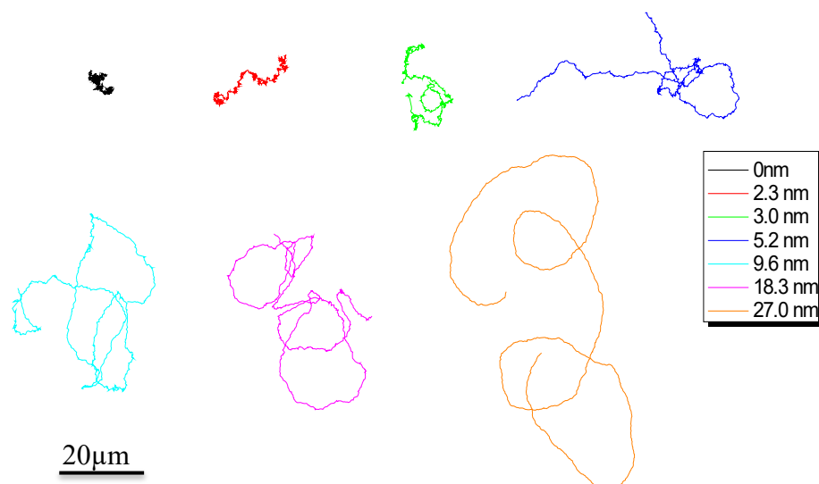
Figure 3-11 Typical trajectories of swimmers measured during the experiment. The maximum Pt thickness is indicated in the legend. All trajectories are represented for 33 seconds.
