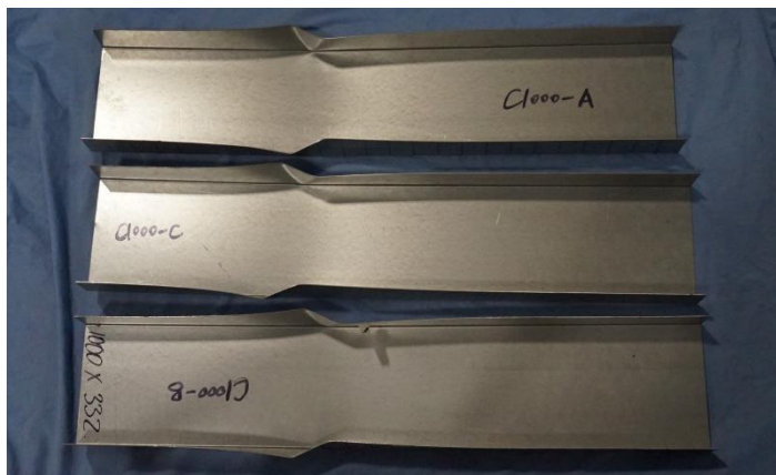
Figure 7.10. Failure modes of 1000 mm long columns with section type C
