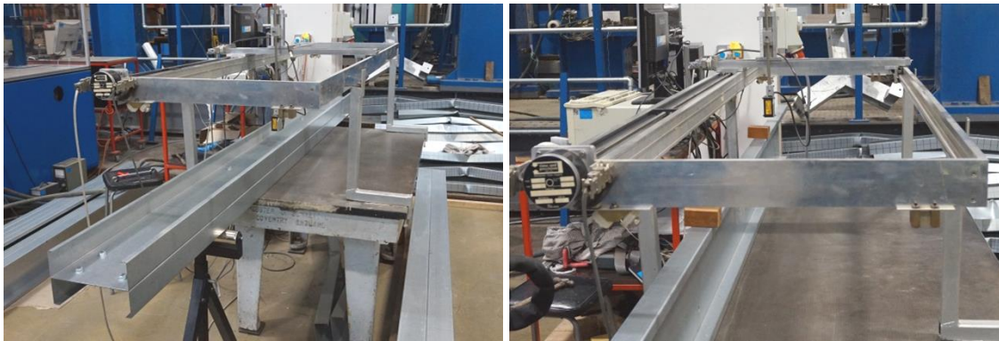
Figure 9.3. The set-up for imperfection measurement
