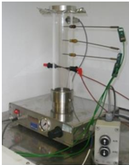
Figure 4.2: Modified Hartmann dust explosion tube
