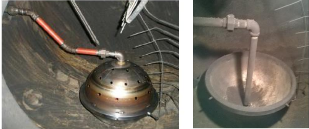
Figure 4.13: Re-design of the hemispherical disperser
