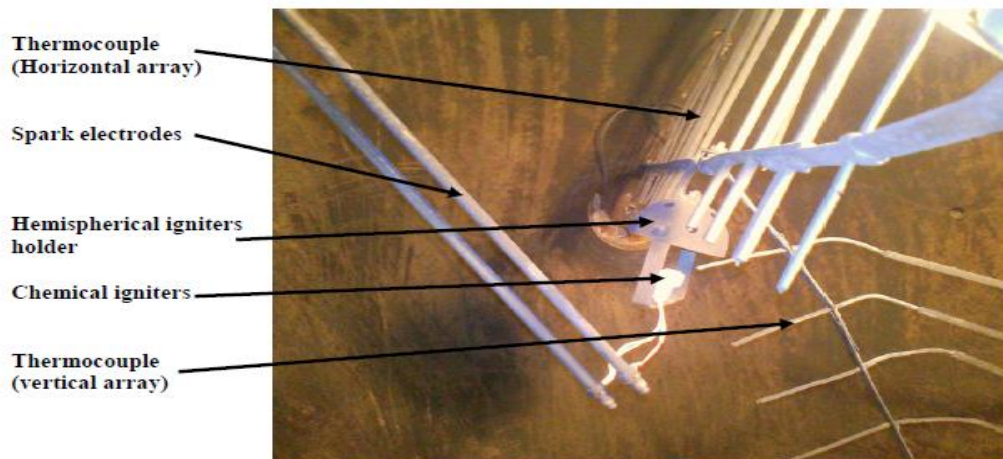
Figure 4.8: Array of thermocouples and igniter
