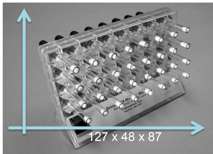
FIGURE 2.2. A Drosophila Activity Monitor: 32 individual flies can be tested at the same time (one fly per hole) and, as a fly walks in the tube, it triggers an infrared beam. As the beam is
