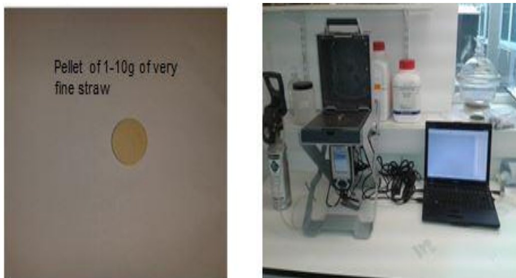
Figure 15: The sample pellet and P-XRF machine
