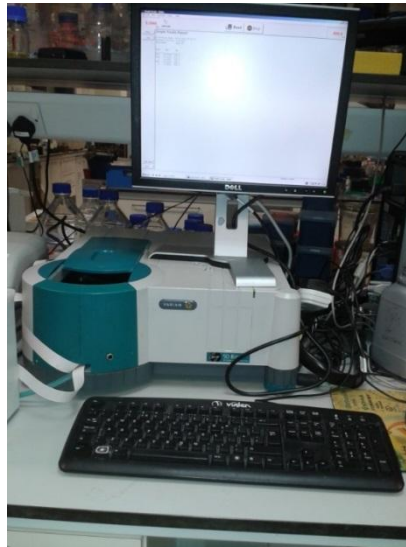
Figure 16: Spectrophotometer: The detection of total lignin was carried out with a UV-detector at 280 nm after Acetyl Bromide Assay
