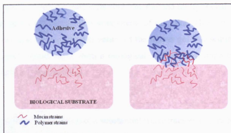
FIGURE 2.7 Molecular model of interdiffusion of polymer chains in adhesion of a polymer with the mucous layer. Left diagram shows polymer and mucous layer before the contact, whilst diagram on the right, shows the interdiffusion of chains after a certain period of contact
